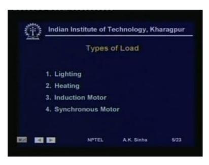
Now, we will talk about different types of load. I have shown here 4 different types of loads. There may be many more, but these are the general types of load that we have. We have lighting load which consists of incandescent lamps, fluorescent lamps, may be discharged lamps. That is those light bulbs that we have incandescent bulbs, then we have fluorescent tubes or compact fluorescent lamps.
