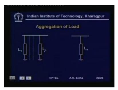
That is at a substation you have large number of loads. These each of this individual loads will have different characteristics. Now, what we need to do is aggregate all of them into one load on the substation. Now, if you want to do that, then we have to again as I said earlier, know different percentage of various categories of loads that we have. And we know the division of various types of loads in these categories. So, we can form
