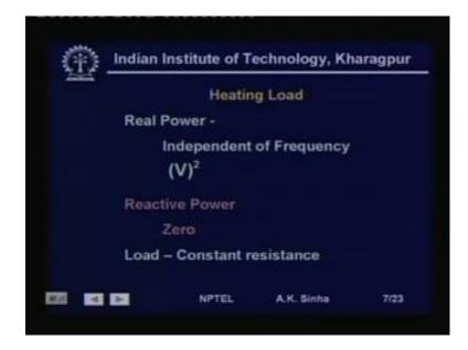
Next we will discuss the heating load. Now, for heating load are basically can be modeled as pure resistors. So, if we are modeling it as pure resistor, then the real power will be equal to V into i and i is equal to V by r. So, actually a real power will be proportional to V square by R, R being constant. So, real power is proportional to the square of the voltage.
