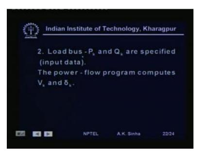
Then, other type of busbar is a load busbar, where both real and reactive power are specified. At this busbar what we what are the unknowns, if we know V and delta at this busbar we have all the variables. So, here P and Q are specified, that is injection real and reactive power injection is specified. And the unknowns at this busbar are V and delta,
