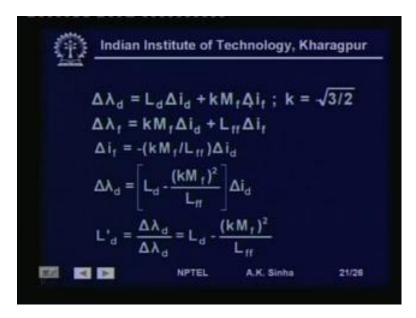
So, we have this changes created by applying of minus v d across the terminals are shown here as delta lambda d is equal to L d delta i d plus k M f delta, if where k is root 3 by 2. And delta lambda f is equal to k M f into delta i d plus L f f into delta i f. Now, since here, all the other sources have been shorted when we are applying this source. So, this is shorted which means delta lambda f is 0, therefore using this delta lambda f as 0 we can calculate delta i f.
