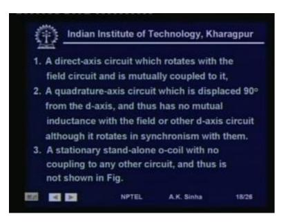
Before we do that, we will like to see what is the importance of this these equations. Now, these equations tell us that a direct-axis circuit, that is the Park's transform converts the stator coils into a direct-axis circuit which rotates with the field circuit and is mutually coupled to it. We have a quadrature-axis circuit, which is displaced at 90 degrees from the direct axis. And has no mutual inductance with the field of the other daxis circuit.
