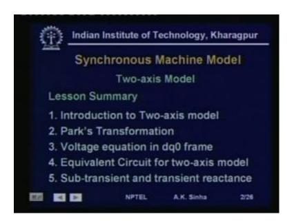
Well, in this lesson we will discuss about the two-axis model, as we talked in lesson 13. We modeled round rotor machine, we said that the other type of machine which is the salient pole machine. That modeling we will be taking up in this lesson and this will require a two-axis model. Because, the magnetic circuit is not uniform for a salient pole machine as we will see.
