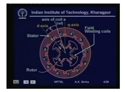
In this figure here, salient pole machine with four protruding poles are shown in this machine. As we see, we have a North pole followed by a South pole, then again a North pole and a South pole. Now, since there are four poles, we also have the coils according to that. We have coils a dash a for phase a, then we have b dash b for phase b which is lagging this phase a by 120 degree. Then we have c dash c which is lagging this by 120 degree.
