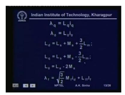
And we will get lambda q is equal to L q into i q and lambda 0 is equal to L 0 into i 0, where, we have this lambda L d as the direct-axis self inductance. That is what we are saying is that, this is the self inductance of fictitious coil which is representing the a, b, c frame coils or the actual a, b, c phase coils in the direct axis. M f is the mutual inductances between the field winding, that is the rotor and the direct-axis fictitious coil.
