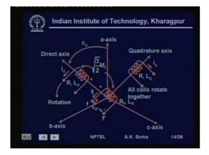
Thus what we see is that the a, b, c phase coils are now replaced by three coils. One which is a direct-axis coil, another is at 90 degrees to it, that is at the quadrature axis. And third coil which is basically as representing the 0 sequence quantities. Since, we will be mostly interested in balanced operation 0 sequence quantities will be 0. So, we do not show that winding here at all.
