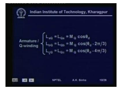
And finally, the mutual inductance between armature coils and the Q winding, this again also will be given by the same L a Q is equal to L Q a is equal to M Q into cos theta d. L b Q is equal to L Q b is equal to M Q into cos theta d minus 120 degrees L c Q is equal to L Q c is equal to M Q into cos theta d minus 240 degrees. Now, since we have seen that most of these inductances, that we have the mutual and the self inductances are basically dependent on the rotor position.
