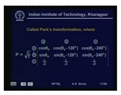
Now, the Park's transformation is shown here, this is carried out for the stator coils. The rotor coils, we do not need to carry this transformation, because we find that the rotor circuit is all the time having a same inductance, the same magnetic circuit. Now, this transformation is written as P, in fact this is somewhat a modified transformation, it is not the original Park's transformation.
