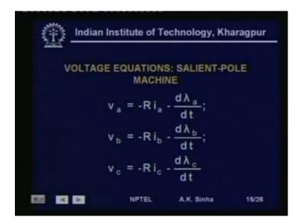
Now, let us write the voltage equation for the synchronous machine. Now, we have the voltage v a equal to minus R into i a minus d lambda a by d t. That is the voltage across the phase a coil is going to be equal to the voltage drop, which is R into i a and d lambda a by d t. That is the rate of change of flux linkage with coil a. Now, these negative signs are coming, because we have considered a generator mode of operation.
