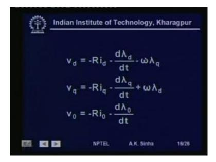
Then, we will get the in d q 0 frame of reference of, as voltages v d equal to minus R into i d minus d lambda d by d t minus omega lambda q, where omega is the synchronous speed of the machine, that is it is d theta d by d t. Similarly, we will get v q is equal to minus R i q minus d lambda q by d t plus omega lambda d; and v 0 is equal to minus R i 0 minus d lambda 0 by d t.
