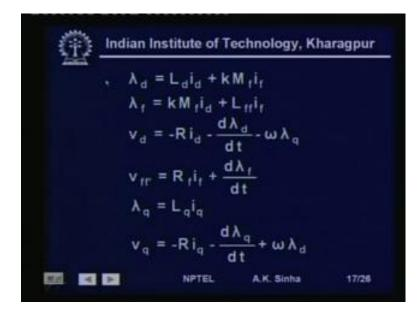
So, again we can write this lambda d is equal to L d i d into k M f i f lambda f is equal to k M f id plus L f f into i f. This is the flux linkage of the coils in the direct axis. This what we had seen earlier lambda d is equal to L d i d plus root 3 by 2 M f. If we are writing this root 3 root over 3 by 2 as k, therefore we have here lambda d is equal to L d i d plus k M f into i f. Similarly, lambda f is equal to k Mf into id plus L f f into i f.
