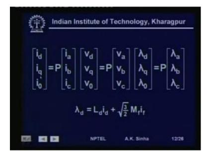
If we pre multiply this matrix to a, b, c frame currents, that is currents in phase a, phase b, phase c given by i a, i b, i c. If we pre multiplied by the P matrix or the Park's transformation matrix. Then the currents that we will get will be i d, i q, i 0, that is the currents will be transformed into d q 0 frame of reference, where D is the direct-axis and Q is the quadrature-axis and 0 represents the 0 sequence quantities.
