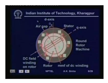
Now, we generally have two types of synchronous machines. One we call as the round rotor machine, where the rotor is built up of solid cylindrical iron on which we have a winding, which is excited or connected to a DC voltage. And this will allow a current to flow in their winding and thereby it produces a field. Now, this field as shown here will produce a North and South pole like this, if the current is flowing in this direction. And the axis of the field will be like this.
