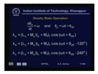
Now, if the speed is constant this means d theta d by d t is equal to omega, which is the speed in radiance per second that is constant. So, from here we will get theta d is equal to that is if we integrate this we can write this as theta d is equal to omega into t plus theta d 0, where, theta d 0 is the value of the angle at time t 0, which we can choose at any arbitrary point. And this omega is basically the synchronous speed of the rotor.
