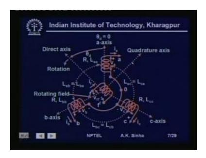
We have a direct axis that is the axis of the field which is at sometime. Suppose this is the position at t is equal to 0. Then this is theta d 0, then what is theta d 0 minus 90 is showing the position of the quadrature axis with respect to the reference axis and that means, this is showing us the angle delta.
