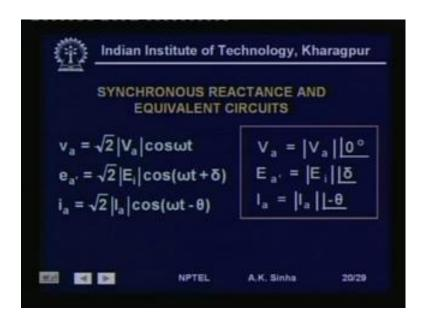
Now, we will talk about synchronous reactance and the equivalent circuits. We have v a we can write the instantaneous voltage v a as equal to root 2 V a capital V a cos omega t. E a dash the induce voltage or the generated voltage as root 2 E i cos omega t plus delta and the current i a is equal to root 2 I a cos omega t plus theta. Or in Phasor forms as V a is equal V a angle 0 E a dash is equal to E i angle delta and I a, as I a angle minus theta.
