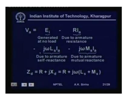
And here we can write this V a is equal to E i minus R into I a minus j omega L s into I a due to armature self reactance minus j omega M s into I a due to armature mutual reactance. So, this we can write these terms due to the inductances can be put as together. And we can write this as the impedance total impedance seen by the winding as Z d is equal to R plus j X d which is equal to R plus j omega L s plus M s.
