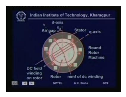
Next, we will try to build a circuit model for a 3 phase synchronous machine with round rotor. Now, here if we see what we have is we have 3 phase windings, the axis of the winding is for phase a winding will be like this. Similarly for phase b winding it will be like this and for phase c winding it will be on this side and so on. So, we will have the axis of these windings 120 degree out of phase from each other.
