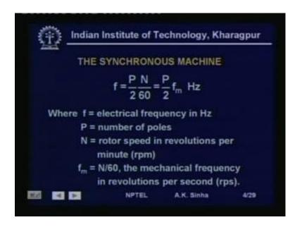
So, this relationship as you can see here is given by f the frequency of supply is equal to P by 2 into N by 60; where P is the number of poles of the machine, N is the speed of the rotor and rpm. This we can also write as P by 2 into f m where f m is equal to n by 60 the mechanical frequency in revolutions per second.
