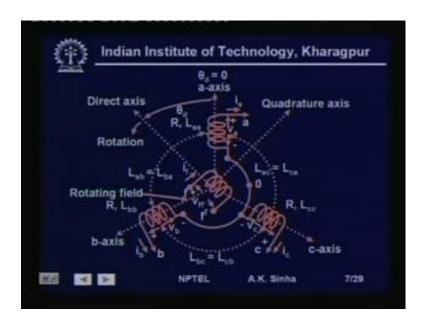
So, with that we can consider this synchronous machine as having a rotor with a winding and the stator having 3 phase windings, this a phase a winding phase, c winding and phase b winding like this. Now, what we generally do is one end of these windings are connected to together and this forms the star point. And we say that the stator winding is connected three phase stator winding is connected as a star winding.
