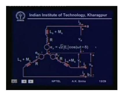
Therefore now using these relations that we have developed till now we have this voltage V a equal to the no load or the generated voltage due to the field ea dash minus R into i a. The current is flowing through this minus L s plus M s into d i a by d t that is the voltage drop due to the inductance of the coil.
