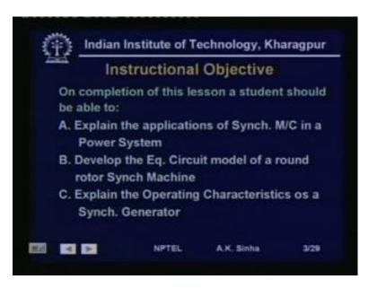
Well once this lesson is over we should be able to explain the applications of synchronous machine in a power system, develop the equivalent circuit model of a round rotor synchronous machine. And explain the operation, operating characteristics of a synchronous generate. Well what is a synchronous machine? A synchronous machine is a machine which has a rotor, which is excited by a DC winding and on the stater it has three windings for three phase power.
