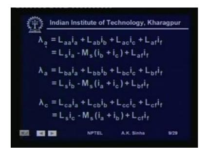
So, with these inductances, now known in this form we can write down the flux linkages with each of these windings. That is the flux linkage of winding a is going to depend on the current flowing in that winding as well as current flowing in the other stator windings. And it is also going to depend on the current flowing in the field winding.
