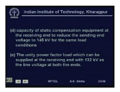
Also we would like to find out the capacity of static compensation equipment at the receiving end to reduce the sending end voltage to 145 kV for the same load conditions. (Refer Slide Time: 38:19)
