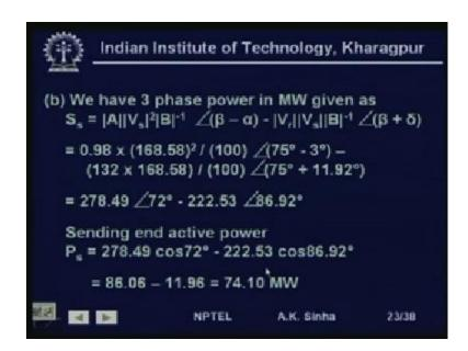
Now, for the b part, where we need to find out the sending end real and reactive power. We have three phase power in Mega Watt given as S s is equal to A V s squared divided by B, with an angle of beta minus alpha for division by B. We are writing B inverse, that is 1 by B minus V r, V s divided by B with an angle beta plus delta. Now, here, mind it, when we are writing this as three phase power, then we are writing V s, V r all as line to line voltages.
