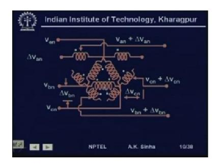
Now, the same thing, if we do by injecting voltage, which is not in phase, but in quadrature. If you look at this transformer, we have a transformer here, like this, which is connected to the primary three phases a n, b n and c n are connected at these points. We have another winding, which has half on this side and half on this side. That is the mid points is connected to this point a and this winding is having the phase of b c.
