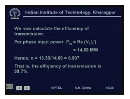
And then we multiply these two, then we are going to get and we take only the real part of that, then we get this as equal to 14.69 Mega Watt. Now, per phase power, which is received, is 40 by 3, which is 13.33. Therefore, efficiency of transmission is output divided by input, which comes out to be 13.33 divided by 14.69. That is 0.907 or the efficiency is 90.7 percent. So, this is one simple problem, that we solved.
