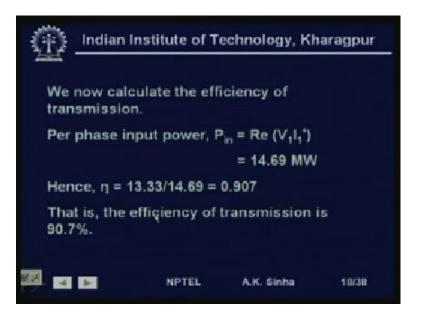
Now, we can calculate the efficiency of the transmission, so per phase, input power will be given by real part of V 1, I 1 conjugate.
