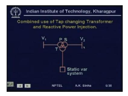
Now, sometimes, we would like to use a combination of the transformer taps as well as the reactive power injection devices. Such as, static power systems or static compensation, any static compensation device, like may be stat com, another devices. So, here I am showing this, there is between these two buses voltage V 1 is at a sending end and voltage V 2 as at the receiving end. We have a transmission line and may be a three winding transformer, which is connected near the receiving end.
