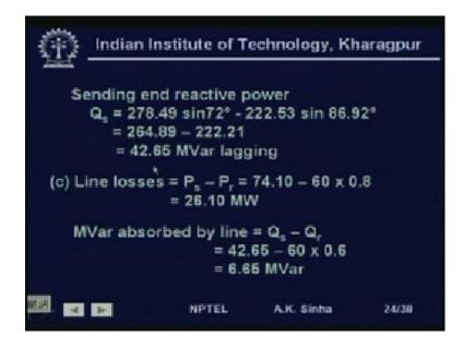
Similarly, we can calculate the sending end reactive power Q s, which will be 278.49 into sin of 72 degrees minus 222.53 into sin of 86.92 degrees. That is, we have to take the sin of the angles, what we had got for S s. Therefore, this comes out to be 264.89 minus 222.21 which is equal to 42.65 Mega Vars lagging. So, this way, we have calculated the sending end real and reactive power.
