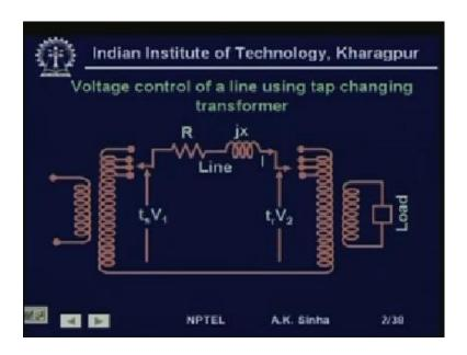
That is, if we go here t s into V 1 will be equal to t r into V 2 plus the drop, which takes place here. If the current flowing in this line is I, then it will be I into Z, Z is equal to R plus j x.
