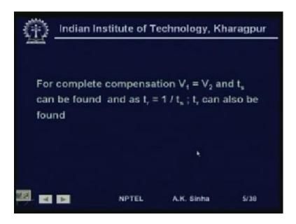
Once, we get t s we know t r is equal to 1 by t s. So, we can also solve for t r. In fact, for any ratio of V 1, V 2 we solve this for t s and then t r.
