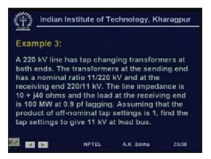
Now, let us take another example, a 220 kV line has tap changing transformers at both ends. The transformers at the sending end has nominal ratio of 11 to 220 kV and at the
