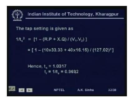
Now, R is given as 10 X is given as 40, therefore substituting this on the relationship for the transformer. That we had derived today, 1 by t s squared is equal to 1 minus R into P plus X into Q divided by V 1, V 2. So, substituting all these values of R, P, X, Q, V 1, V
