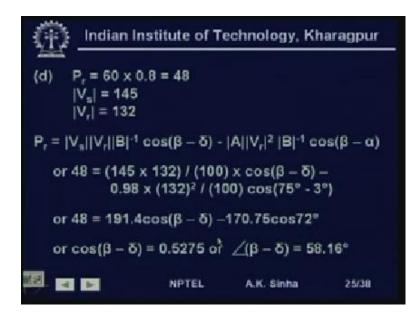
Next, we say that, we want to keep the sending end voltage at 145 kV and the receiving end voltage is kept at 132 kV, then what is the amount of compensation, that is required. Now, the since we are transmitting 60 MVA at 0.8 power factor lagging, which comes out be 48 Mega Watt. Therefore, for this P r is equal to 48 Vs is equal to 145 kV, V r is equal to 132 kV.
