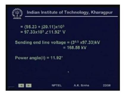
So, when we do this calculation, this comes out to be 95.23 plus j 20.11 into10 to the power 3. That is equal to 97.33 into 10 to the power 3, volts with an angle of 11.92, which tells us that the sending end voltage phase to neutral voltage is 97.33 kV. And the power angle is 11.92 volts, because this is the angle of the sending end with respect to the reference.
