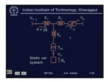
The whole diagram an electrical circuit can be represented by this, where, we have V 1 the sending end, the current I is following through this. X 1 is the reactance of the transmission line, we have neglected the resistance. So, it is the reactance of the transmission line, plus the reactance of the primary side of the transformer winding. X 2 is the reactance of the secondary side of the transformer winding. And X 3 is the reactance of the tertiary winding.
