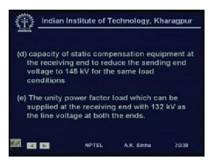
Also we need to find, the unity power factor load, which can be supplied at the receiving end with 132 kV as the line voltage at both the ends. Now, if we want to keep the voltage at both the ends at 132 kV, then what is the amount of unity power factor load?
