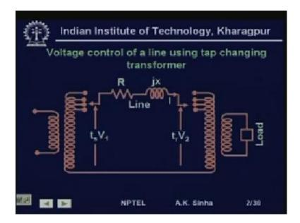
In this case here and here, both the voltages on the transmission line, two ends being equal.
