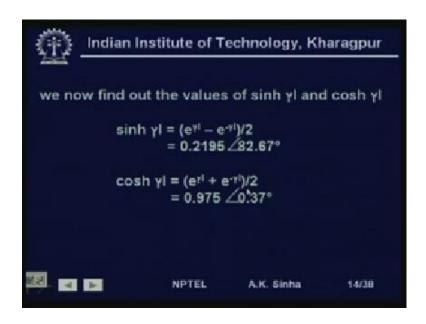
Hyperbolic gamma l sign hyperbolic gamma l is equal to e to the power gamma l minus e to the power of minus gamma l divided by 2, which is after substituting the value of gamma l will come out to be 0.2195 with an angle 82.67. Similarly, cos hyperbolic gamma l will be equal to e to the power gamma l plus e to the power minus gamma l. This whole divided by 2, which will come out to be on substituting the values of gamma l. This comes out to be 0.975 with an angle 0.37 degrees.
