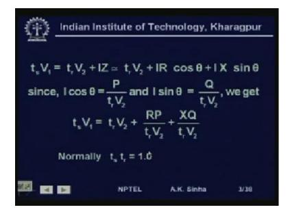
Therefore, we have t s into V 1 is equal to t r, V 2 plus I into Z. Now, this will be approximately equal to t r into V 2 plus I into Z is I into R plus j x, which we can write as approximately equal to I into R cos theta plus I into X sin theta. Now, we also know that, I cos theta will be equal to P by t r into V 2, because t r into V 2 is the voltage. So,
