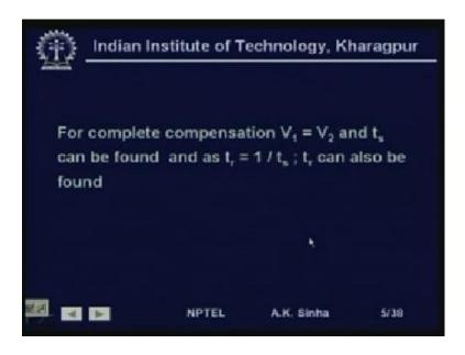
So, from this, we can find out the value of t s for a complete compensation. That is, when V 1 is equal to V 2. Mind it, we are writing all these values V 1, V 2 as per unit values. So, if we want both of them to be 1 per unit, then we can write this as V 1 is equal to V 2 or both side voltages, becoming equal.
