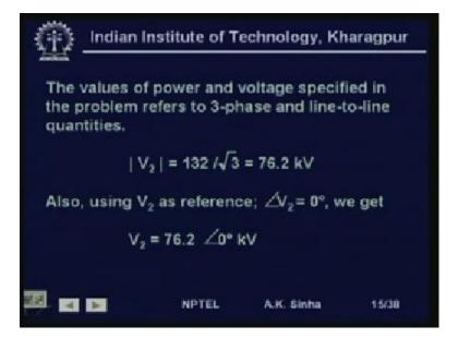
So, knowing sign hyperbolic gamma l cos hyperbolic gamma l and Z c. We can calculate a, b, c, d parameters for the transmission line. Now, the value of power and voltage is specified in the problem refers to three phase and line to line quantities. That is the values, that we are given in the problem is in terms of 132 kV, which is a line to line voltage and 40 Mega Watt, which is a three phase power.
