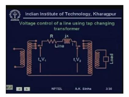
So, we will start with voltage control of a line using tap changing transformers. Here, we have this transmission line, given by it is simple short line model of R plus j x. We have neglected the shunt capacitance for the line in this model. And we have step up transformer, at the sending end. And we are assuming that we have a generator on this side and we have a step up transformer here.
