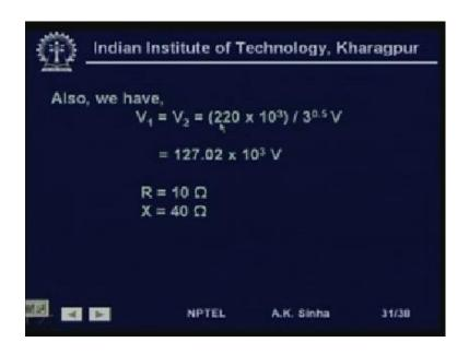
Now, we have V 1 is equal to V 2 is equal to 220 kV and since, we want to work out on a per phase basis. So, we divide it by root 3. So, we will get the line to neutral voltage. So, 220 into 10 to power 3, divide by root 3 volts. This is coming out to 127.02 Kilo Volts.
