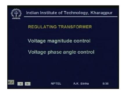
Now, many times we use regulating transformers. Basically, these transformers are used for injecting voltage into the transmission system. If we inject the voltage in the same phase as the voltage on the transmission system, then what we will be doing is, either we can add the voltage. And therefore, boost the voltage or if we want we can inject the voltage in opposite phase. Then, we will be reducing the voltage or bucking the voltage.
