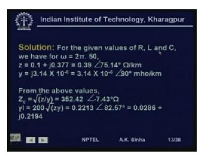
Now, for the given values of R L and C, we have omega. That is the equal to twice pi into f f is 50 hertz, therefore, we can calculate the series impedance per unit length or per kilometer as 0.1, which is the resistance plus j, 0.377. That is twice pi f into L. That is 1.2 milli henry, per kilometers. So, this comes out to be 0.1 plus j 0.377, which is equal to 0.39 with an angle of 75.14 in ohms, per kilometer.
