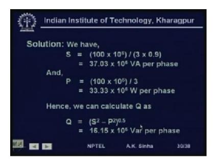
So, this is the example, for what we take for tap changing transformer in today's class. So, now S is equal to 100 MVA, let us 100 Mega Watt is being transmitted at 0.9 power factor lagging. So, S per phase will be 100 into 10 to power 6, this is Mega Watt divided by 3. So, that is Mega Watt per phase divided by 0.9 will give me because 0.9 is the power factor, this will give me the MVA.
