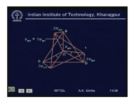
And if we see the phasor, it comes out to be V a is the voltage plus delta V a n is added here. V b is the voltage plus delta V b n is added here. V c is the voltage and delta c n is added here. So, now the new voltage a dash, b dash and c dash will be these points. And we see that, though there may not be large change in the magnitude, the angle of these phases has change. That is a dash is now leading a by this angle theta.
