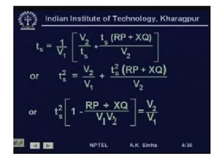
Then, if we do that, then we can write t r is equal to 1 by t s. And therefore, substituting that, we get t s is equal to 1 by V 1. That is V 1 t s is equal to V 2 by t.
