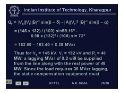
So, we will use this. Now, we know Q r is equal to V s, V r divided by B into sin beta minus delta minus A V r square divided by B into sin beta minus alpha. So, again substituting the values, we will get Q r is equal to 145 into 132 divided by 100 into sin 58.16. This is beta minus delta into A 0.98 into V r square 132 squared divided by 100 into sin 72 degrees. So, after calculating this comes out to 162.60 minus 162.40, which is equal to 0.2 Mega Var.
