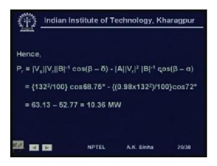
Now, since we have calculated beta minus delta, we can write down the equation for P r, V s, V r by B into cos beta minus delta minus A V r square by B into cos beta minus alpha substituting all the values, we will get this as 10.36 Mega Watt. That is, if we want to keep the voltage at both ends equal to 132 kV and we want to supply unity power factor load. Then the load that we can supply will be only 10.36 Mega Watt.
