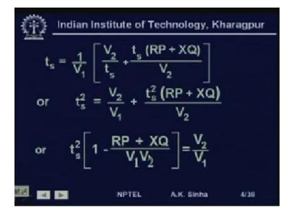
So, this becomes V 2 by t s plus t s into R P plus X Q by V 2, which if we multiply the both sides by t s. Then, we get t s squared is equal to V 2 by V 1, because this t s will cancel out plus t s squared, because it is multiplied by t s. So, t s squared R P plus X Q divided by V 2, I am sorry, this should be V 1, V 2. And therefore, if we take this taking on this side, then we will get t s squared one minus R P plus X Q divide by V 1, V 2.
