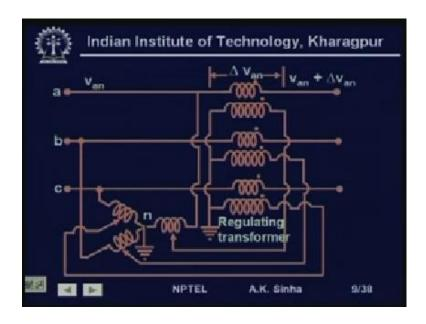
So, here, this is voltage magnitude controller or regulating transformer, which controls the voltage magnitude only. If you look at this, here we have transformer winding, which is a three phase winding, connected to the three phase transformer. And we have taps on this winding. Now, based on all these three taps on the three phases are all ganged. So, they will move together.
