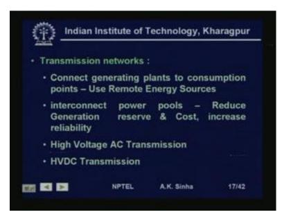
Now, transmission systems basic job is to connect generating plants to consumption points. That is to use remote energy sources, since the energy sources are not very near to the loads. So, we need to transmit this energy. Same is the situation with hydel plants. They are built near the dams where these resources are available. And we will have to transmit all this power, to places where it needs. So, a transmission system does this job.
