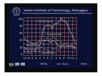
Now, as we see from this diagram which is a typical system load profile. That here what we have seen is, the system load is never constant, it keeps on changing at different times. We have a very low loading at early morning time, may be around say around, this is showing. So, late in the night we have very low loading, this should not be 10 this should be 2, 4, 6, 8, 10, 12 and so on, anyway this is.
