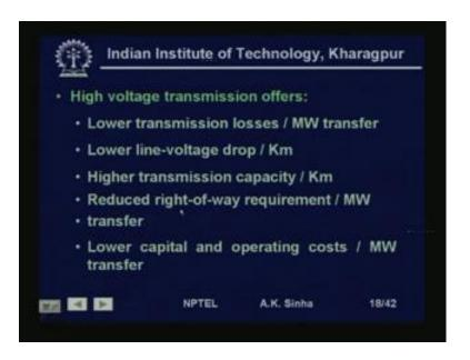
Now, what are the advantages of using high voltage transmission system. First is we have lower transmission losses per megawatt of power being transferred. We have lower line to voltage drop per kilometer. Because, we are working at high voltage the i square r losses. Since the voltage is high, the current will be low for the same amount of power. So, i square r losses are going to be low. So, transmission losses are going to be low, if we work at high voltage.
