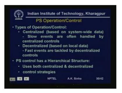
So, this is what is the goal of the operation and control of power system. Of course, this is achieved by means of what we call, a hierarchical control system, where the larger controls and the slow acting controls are done by means of a centralized controls, whereas the first acting controls, like protection another systems. They are done by means of decentralized control, that is local controls.
