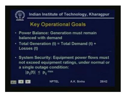
So, one of the key operational goals as we said is power balance. Because, when you generation must balance with the demand. That is when I switch on the generation must go up. But, how does a generator see that you have switched on your device, it does not know. So, this kind of indication comes to it by means up a drop in frequency. So, when a operator sees, that the frequency is dropping what he does is, he increases the input of this stem to the turbine, and because this input has increased.
