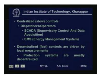
Centralized controls some of the example has SCADA system, EMS systems. Decentralized controls as I said protection systems. Some controls like your speed governing system for turbines, for generators all these are also decentralized control.
