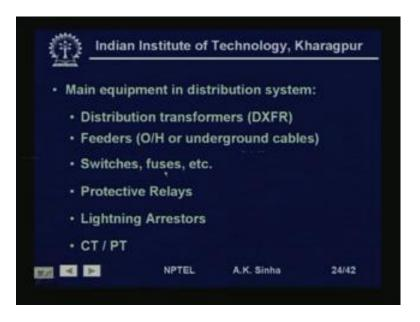
The main equipment of a distribution systems are again you have in the distribution system. Once you have got the power at higher medium voltage, you step it down by means of distribution transforms. Which then we have feeders or which are basically overhead or underground cables to provide the transmission. Or to carry this electrical energy up to the consumer premises, we have again switches, fuses etcetera.
