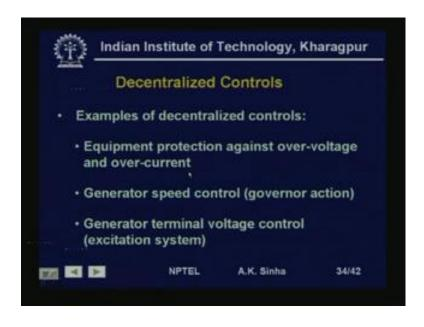
All these are generally done on for centralized control purposes. Whereas, decentralized control as we said speed governing system, protection system, voltage control system. Automatic voltage regulators or the excitation control of each generator, these are decentralized control options.
