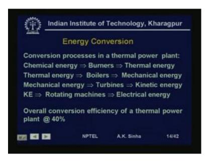
Here if we see, initially the chemical energy in a coal, is in the burner is converted converts it to thermal energy. Then, thermal energy is converted to mechanical energy in the boilers. And that is the steam at high temperature in pressure. The mechanical energy of this steam is converted by turbines into kinetic energy. The kinetic energy of the rotation is converted into electrical energy in the rotating machines, which is mostly a three phase synchronize machine.
