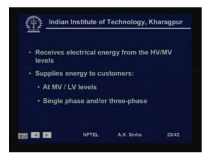
Now, the distribution system receives electrical energy from high voltage and medium voltage levels. From the transmission system and sub-transmission system. In fact, below the transmission we also have, what we call as sub transmission system. But, generally all this is clubbed into one part, which we call the transmission system. Then it is supplies this energy to the consumers, at medium level and low voltage levels.
