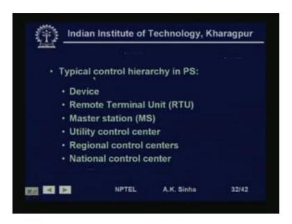
Typical control hierarchy is device. Then we have remote terminal units, master stations, utility control centers, regional control centers and national control centers. So, from the device the information goes after the national control center. They are concentrated at these levels and then, they are send further.
