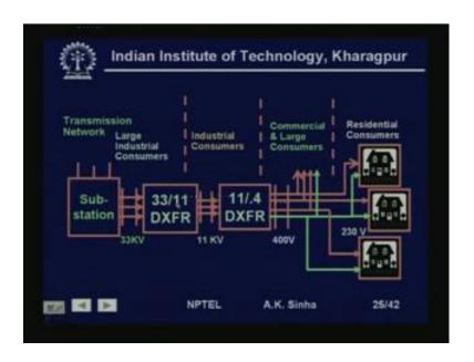
This is very simple representation of a distribution system, from the transmitter network. We come to a substation at the high voltage or medium voltage level. There we have, once we have got this power at 33 KV level, by means of transformer here. This goes up to some large industrial consumers at 33 KV level or may be at 11 KV level. So, we have a 33 to 11 KV level transformer, which we call distribution transformer are used for this purpose.
