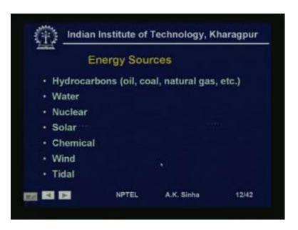
So, here if we see based on the energy sources, if we are using hydrocarbons. That is oil, coal, natural gas, etcetera. Then, oil and coal plants are generally called the thermal power plants. Because, oil and coal is used that is the thermal energy is burnt in a boiler. And this heat of this as used to makes steams which is use to run steam turbines. Similarly, natural gas is used to be burnt in gas turbines and produce electrical energy.
