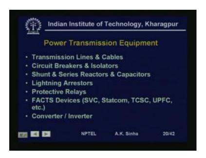
The other equipment that we use are of course, lines and cables to carry the power, circuit breakers and isolators. Circuit breakers are used to disconnect the line when case of falters. Some other reason, isolators are also same kind of switches. That main difference between circuit breakers and isolators are that circuit breakers can break a circuit in which current is flowing. Whereas, isolators are used only to isolate circuit, when it is not carrying any current.
