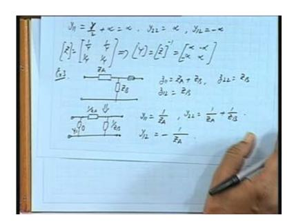
So this plus this will be Z B itself okay now if you are ask to calculate the Y parameters for this then I will take an equivalent phi. So this is 1 by Z A admittance, this one, this admittance is 1 by
