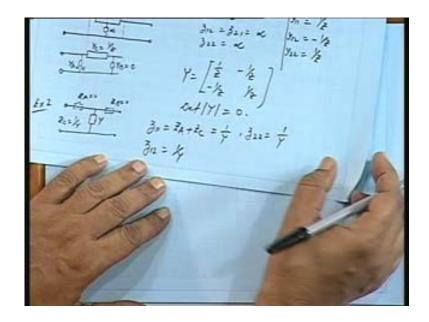
So how much is Z 11, ZA plus ZC is it not that is equal to 1 by Y, what about Z 22 similarly, 1 by Y okay and Z 12 yes, Z 12 will be again no Z 12 does not have a negative sign, it is y 12 in the short circuit case only you get negative sign in the impedance terms you do not get a negative signs, so Z 12 is just this impedance which is 1 by Y.
