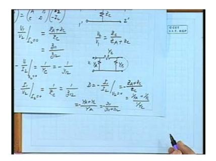
So I short this and how much is I 1, I 1 is this current and this entire current through YC will flow through the short circuited path so I 2 flows through this. So it is this current by this current, so what is this current what fraction of the main current is this YA by YA total by C, YC, yes, yes, 1 by YA by if you talk in terms of impedance say it is ZA by ZA plus ZC, is it not. So I 1 by
