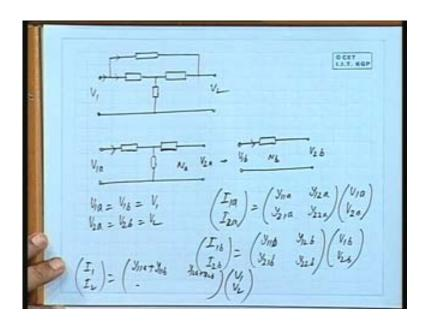
When I say the 2 networks are in parallel what are the common features, what are the things which are common the voltage applied here V 1 and V 2 are same if I call it V 1 A and V 2 A for this network V 1 B and V 2 B then V 1 A equal to V 1 B is equal to V 1 and V 2 A is equal to V 2 B is equal to V 2. This voltage is same as this and this, this voltage is same as this and this okay.
