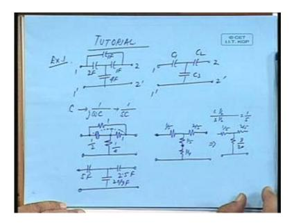
Now in this case, as you know a capacitor is having an impedance if you talk in terms of sinusoids it will be 1 by omega C, it is a j here if you talking Laplace domain it will be 1 by Sc that means the impedance is inversely proportional to C. So I can take these capacitances to the equivalent impedances or even resistances with the values which will be just inverse of these something like half ohms, one fourth ohm, 1 ohm and 1 ohm, I can replace it by an equivalent impedance circuit.
