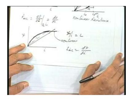
So an inductance will be present whether it is a straight conductor or a coil whether it is carrying AC or DC okay for example, when you go to the market to buy a an inductance, you do not say I will be using it for AC please give me an inductance to be used for an AC, you do not specify this is 2 milli Henry, 3 milli Henry, you specify only the value in Henry, I want so much current
