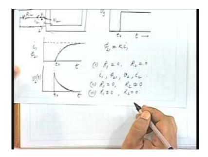
So flux is also increasing like this, so what is the voltage induced, it will be N 2 times D phi 21 by dt. So it will be depending on the slope, is it not, so how is a slope changing. Initially the slope is this much and gradually it is becoming 0 so if you apply dc, dc supply on to a transform
