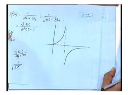
Let us see the admittance of this, it will be 1 over this quantity okay 1 by j omega 1 minus j by omega c. So how much is it if I multiply by omega c divided by omega square LC minus 1 j can
