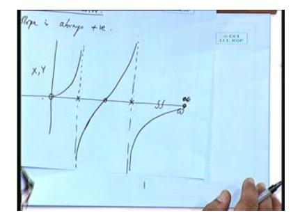
So this is for x or y either of them then from a pole, from a pole it has to go through 0 and approach again infinity from minus infinity it can go to plus infinity passing through a 0 it cannot go this way because then it will ensure a negative slope and we have seen the slope has to be positive. Similarly from this infinity to 0 it will asymptotically approach 0 this can be the possible x omega characteristics for a given set of pole 0 configuration is that alright.
