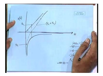
At infinity, this is infinity so this is a pole so you see pole, 0, pole, 0, pole again they are coming alternately okay. So LC network, LC network if we have similar to this if I take y(s) an admittance function the poles and 0s will be just replacing interchanging their positions this will be a 0, this will be a pole and so on so there also pole 0 poles and 0s will be appearing alternately. Hence forth, we will draw a diagram.
