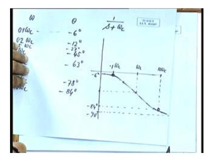
So we will make a table like this omega if the function is like 1 by S plus some omega c, some critical frequency then omega if it is omega c by 10 that is .1 times omega c and 10 times omega c then the corresponding thetas are this should be minus 6 degrees and this one will be 90 minus 6 degree, so minus 84 degrees, you just compliment, is it all right? if it is
