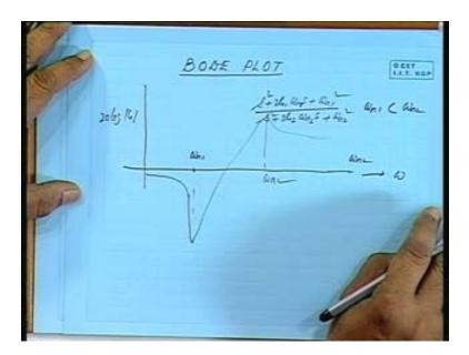
Omega  $n_1$  there was a frequency omega  $n_2$ , so what I meant was omega  $n_1$  is less then omega  $n_2$  and it was in the numerator S squared plus twice zeta 1 omega  $n_1$  S plus omega  $n_1$  squared divided by S squared plus twice zeta 2, omega  $n_2$  S plus omega  $n_2$  squared. So the curve was somewhat like this okay this was omega  $n_2$ , this was omega  $n_1$  okay. In the phase plot this
