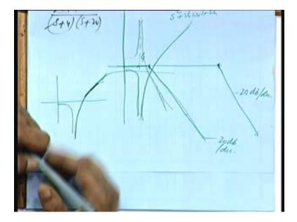
It will look like this it will be a function which will be going like this and then 20 db fall and 40 db increase so from 4 onward it will be 20 db per decade net result all right and then from 20 omega equal to 20 onward, it will become horizontal. So the net result will be somewhat like this 3 and 4 are very close so you will not able to see 40 db slope anywhere it will be gradually going up to 20 db per decade slope and then finally catching up with the horizontal line.
