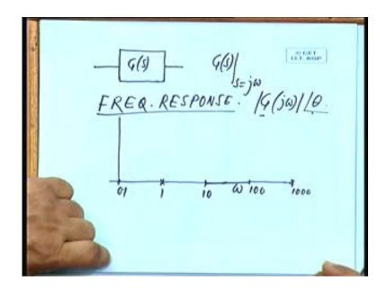
So this will be having an magnitude and a phase what is the magnitude? 1 by 10 root 2, what is the phase? minus 45 degrees at this frequency omega will be 10. So 50 was the amplitude of the input that gets multiplied by that magnitude of G j omega is that all right. So it will be 51 by 10 root 2 this will be the amplitude of the output  $\sin 10$  t the same frequency  $\sin 10$  t with the phase shift of theta here theta is minus 45 degrees, this will be the output. So the current you can
