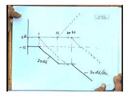
So at omega equal to10 you are having a numerator function that means it will be increasing 20 db per decade line will be like this and at omega equal to 1 it is falling like this 20 db per decade at 20 again it is falling like this. So what is the net sum it is this plus, this plus, this plus, this, so minus 12 db the net value say in this range is minus 12. So it will be following this way minus 12 then at omega equal to1 there is a slope of 20 db per decade the fall starts.
