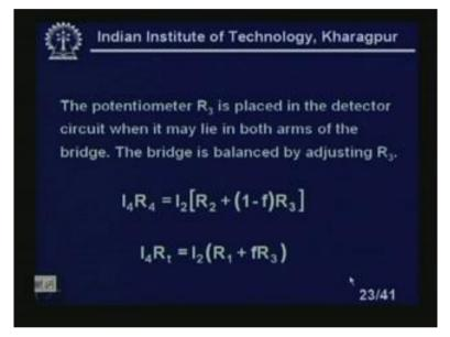
Now, the potentiometer R 3 is placed in the detector circuit when it may lie in both arms of the bridge. The bridge is balanced by adjusting R 3. So, I am writing the equation I 4 R 4, if I look at the top one, equal to I 2 R 2 plus 1 minus f into R 3 is the first equation on the bridge balanced on the right hand side or and also I can write I 4 R t I 2 R 1 plus f R 3.
