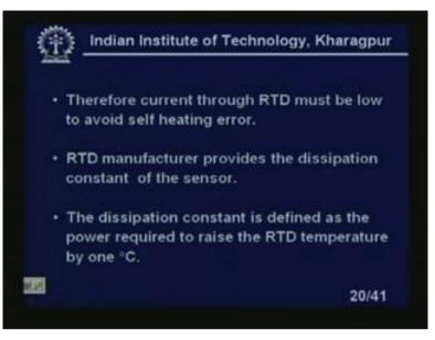
Therefore, the current through RTD must be low to avoid the self heating error. Now, usually RTD manufacturer provides the dissipation constant of the sensor. What is the dissipation constant? The dissipation constant is defined as the power required to raise the RTD temperature by 1 degree centigrade, right?
