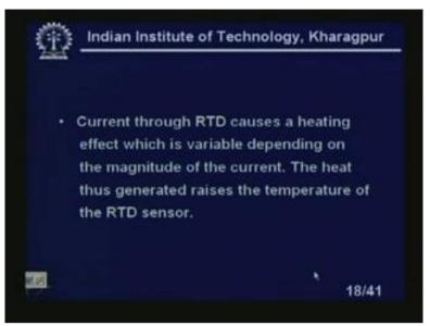
Now, current through RTD causes a heating effect, which is variable depending on the magnitude of the current. The heat thus generated raises the temperature of the RTD sensor.
