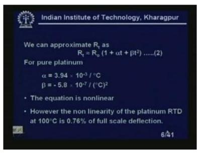
We can approximate R t as R t equal to R naught 1 plus alpha t plus beta t square; R t equal to R naught 1 plus alpha t plus beta t square. This is equation number 2. For pure platinum, alpha equal to 3.94 into 10 to the power minus 3 per degree centigrade and beta equal to minus 5.8 into 10 to the power minus 7 per degree centigrade square. Equation is nonlinear. You see, the equation 1, which we have discussed, we have seen it is a nonlinear equation.
