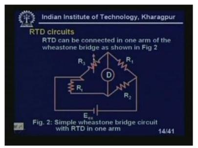
Now, RTD circuits, how will I, now actually what is in the RTD circuit? If the temperature changes, the resistance will change. So, somehow or other, I have to measure that resistance change, right, so that the resistance change can be calibrated in terms of temperature. That is the very simple, how we can make the measurements and how we can measure the, how we can make or how we can make convert this resistance change in temperature. That is our goal in formatting RTD circuits.
