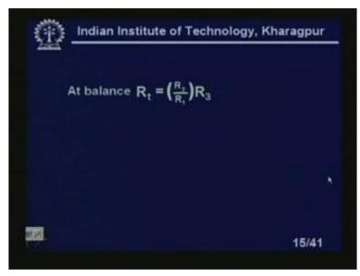
At balance, obviously you know that it will be R 2 by R t equal to R 2 by R 1 into R 3. It is very simple. I should not draw it, even though it is a basic Wheatstone bridge, anyway and for sake of completeness, I am drawing.
