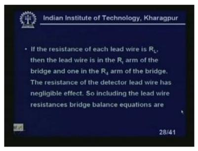
If the resistance of each lead wire is R L, then the lead wire is in the R t arm of the bridge and one in the R 4 arm of the bridge. Quite obviously, it is in the R t arm of the bridge and the R 4 arm of the bridge. The resistance of the detector lead wire has negligible effect, because it is not coming in the picture. So, because it will make,
