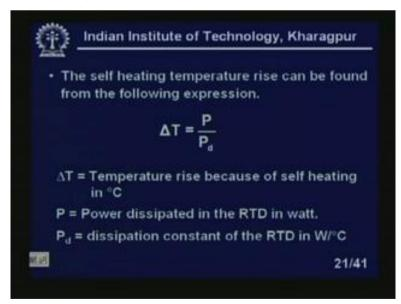
Now, the self heating temperature rise can be found from the following expressions; very simple, delta T equal to P by P d. What is this P? Delta T is the temperature rise,
