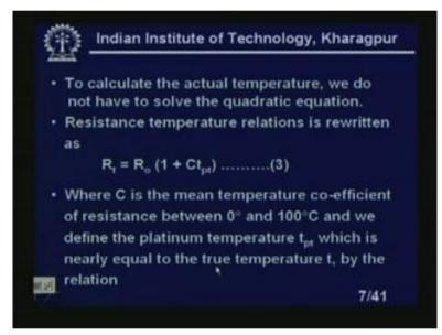
So instead, the resistance temperature relation is rewritten as R t equal to R naught multiplied by 1 plus C into t pt. This is equation number 3, where C is the mean temperature coefficient of resistance between 0 degree and 100 degree centigrade.
