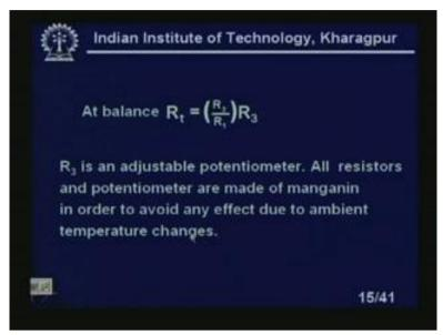
So, this is the balance equation; I have taken R t equal to R 2 by R 1 into R 3. So, R 3 is an adjustable potentiometer. All resistors and potentiometers are made of manganin, in order to avoid any effect due to ambient temperature changes. You know, manganin has a lowest temperature coefficients of resistance, so we always choose manganin to avoid any ambient temperature change, right?
