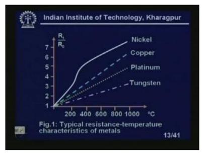
So, now this is the figure 1, where you can see the typical resistance temperature characteristics of metals. We can see, here we have plotted R t by R 0 in y-axis, temperature in the x - axis. Obviously, at zero degree centigrade R t by R 0 will be 1. You have plotted in the, first one is of nickel. Then you have plotted for copper, then you have plotted for platinum, then you have plotted for tungsten. You can see that the platinum, sensitivity of the platinum is rather low.
