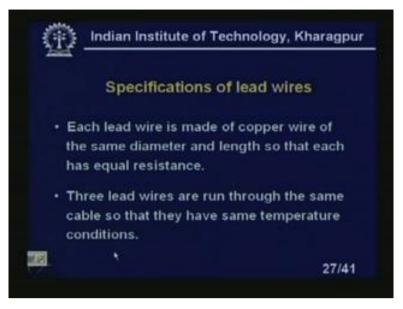
The three lead wires are run through the same cable, so that they have assumed or they have the same temperature conditions. This is also necessary.
