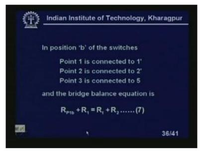
And in position 'b of the switches, we have changed the connections. We have changed the connection. Point 1 is connected to 1 dash, then 2 is connected to 2 dash and 3 is connected to 5, right? So, the bridge balance equation is R p1b plus R 1 equal to R t plus R 2, right. This is bridge balance equation.
