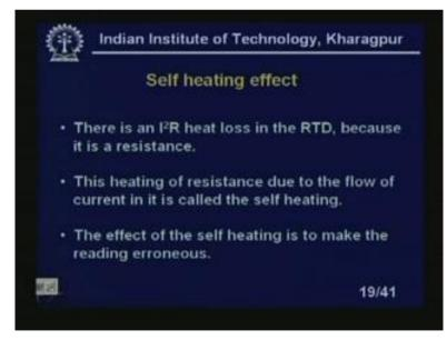
Self heating effect - there is an I square R heat loss in the RTD, because it is a resistance. There is an I square R heat loss in the RTD, obviously any resistance. So and this self heat is called a self heating effect. You see, it cannot avoid, it, this is, this
