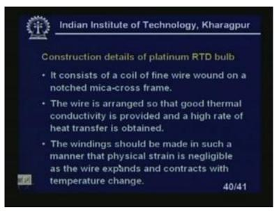
Now, construction details of the platinum RTD bulb - you see here the construction details. It consists of a coil of fine wires wound on a notched mica cross frame. We will show that. The wire is arranged, so that the good thermal conductivity is provided and a high rate of heat transfer is obtained. This is, another thing is necessary and the windings should be made in such a manner that the physical strain is negligible as the wire expands and contracts with the temperature changes.
