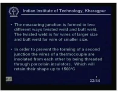
In order to prevent the forming of a second junction, the wires of a thermocouple are insulated from each other by being threaded through the porcelain insulator, which will retain their shape up to 1500 degree centigrade, because the two wires might get connected. If it is connected, you will get a second junction that is undesirable, so what we will do? We will pass through the insulator and it can retain a shape of 1000, up to temperature of 1500 degree centigrade. It looks like this.
