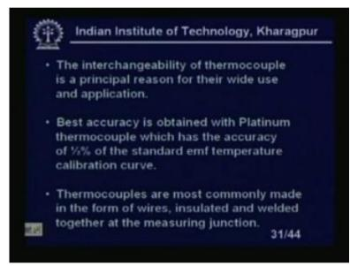
The interchangeability of the thermocouple is a principle reason for their wide use and application. Best accuracy is obtained with the platinum thermocouple, which has the accuracy of half percent of the temperature emf calibration curve. Thermocouples are most commonly made in the form of wires insulated and welded together at the measuring junction. As I told you, there are two types of weld. A twisted weld and a butt weld. What is that?
