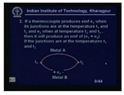
Now, if a thermocouple produces emf e 1, when its junctions are at the temperature t 1, you can see here, if a thermocouple produces emf e 1, when its junction at the temperature t 1 and t 2, these are the temperature at t 1 and t 2, so with two different temperature, this is a metal A, this is a metal B, this is a whole ...... I got a voltage e 1, right and e 2, let that, for that we have to go for next slide.
