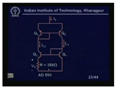
This is the simplified circuit of the cold ... AD590. You see, the two transistors. Its, I T is divided in two half Q 3 Q 4 and Q 2 Q 1 and there is a resistance R. The details is coming next.
