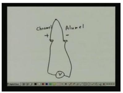
You see it is a, if I take like this one, this is our thermocouple, right? So, suppose this is chromel and this is alumel, so this will give you positive voltage, the positive side of the voltage. You see, thermocouple output is a pure DC voltage, right, so there should be, some probability will be there, so which is positive, this is negative. This is very important, while you will see in the lead wires, connections and all those things.
