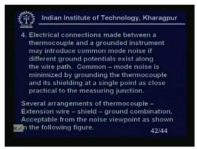
Electrical connections made between the thermocouple and the grounded instrument may introduce common mode noise, if different ground potential exists along the wire path. Common mode noise is minimized by grounding the thermocouple and its shielding at a single point as close practical to the measuring junction. Now, several arrangements you can have for extension wire shield and ground combination acceptable from the noise view point, as shown in the following figure.
