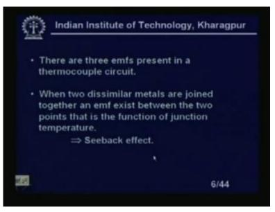
Now, there are three emf present in this thermocouple circuit, right? We have when two, Seeback effect when two dissimilar metals are joined together and emf exists between the two points that is the function of the junction temperature. This is the most prominent. Otherwise, we will find the other, like Peltier's and the Thompson of all, also will exist there, but it is not that prominent.
