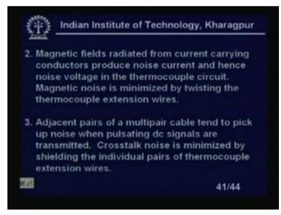
Now, magnetic fields radiated from the current carrying conductors produce noise current and hence noise voltage in the thermocouple circuit. So, magnetic noise is minimized by twisting the thermocouple extension wires. Adjacent pairs of a multipair cable tend to pick up noises when pulsating dc signals are transmitted, as I told you. Now, crosstalk noise is minimized by shielding the individual pairs of thermocouple extension wires.
