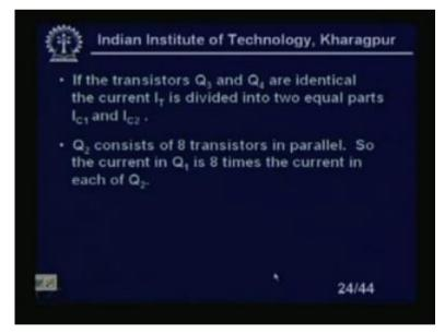
If the transistors Q 3 and Q 4 are identical, the current I T is divided into two equal parts I C1 and I C2. Let us go back, so we can go, so I C1 and I C2, it is going in the I C1 and I C2 dividing two equal parts I C1 and I C2. Now, Q 2 consists of 8 transistors
