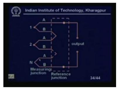
You see, this is actually a thermopile or a multiple thermocouple. There is a measuring junction, several measuring junction, it can be 'N' such measuring junction. Cold junction will be at one temperature, measuring junctions at one temperature. So, this is the reference junction. So, what will be the output? Output will be the 'N' times the voltage of the single thermocouple. This is because, they all are in series, right? So, I will get obviously large output, right?
