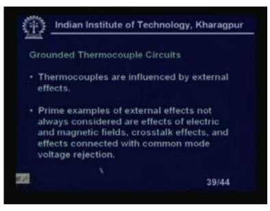
Now, grounded thermocouple, you see thermocouples are influenced by the external effects. Prime examples of the external effects not always considered are the effects of electric and magnetic fields, crosstalk effects, I mean effects connected with the common mode voltage rejection.
