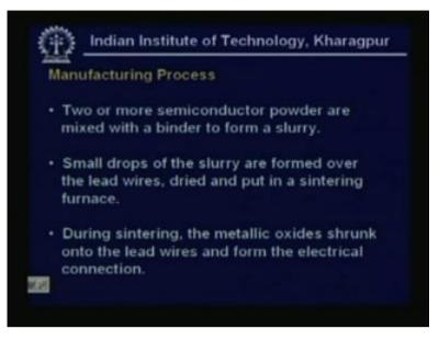
Now, manufacturing process if you will look at, two or more semiconductor powder are mixed with a binder to form a slurry. Small drops of the slurry are formed over the lead wires, dried and put in a sintering furnace. During sintering, the metallic oxides shrunk onto the lead wires and form the electrical connection.
