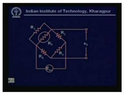
This is another circuit of the thermistor, which is used in a bridge circuit. You will see here, there is typical reason why we have connected a resistance in parallel with the thermistor. Now, as I told you, thermistor is a nonlinear device. So, linearity is a great problem with the thermistor, so what they are doing? They always, there is a common thumb rule that you use a resistance in parallel with the thermistor, right? So, what will happen you see?
