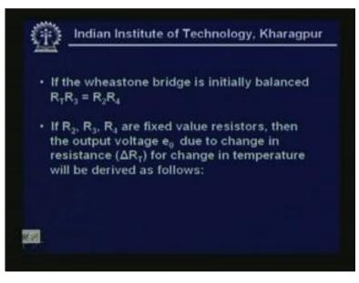
Now, if the Wheatstone bridge is initially balanced, we assume that the Wheastone bridge is initially balanced, even not, not necessarily that the, all the resistance will be
