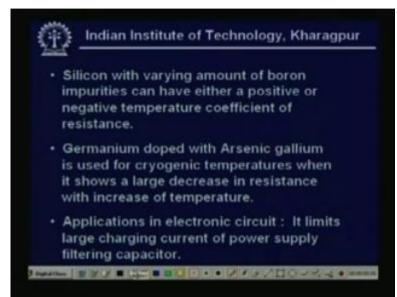
Now, silicon with varying amount of boron impurities can have either a positive or negative temperature coefficient of resistance. So, you can have either positive thermistor or a negative thermistor. We are not interested to have a positive temperature coefficient, because we have many other sensors. But we need negative temperature coefficient that also with a very high sensitivity, which is available in th case of thermistor.
