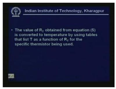
The value of R T obtained from the equation 5 is converted to a temperature by using tables that list T as a function of R T for the specific thermistor being used, right? So,
