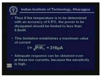
So, thus if the temperature is to be determined with an accuracy of 0.5 degree centigrade, the power to be dissipated should be limited to less than 0.5 milliwatt, right? This limitation establishes a maximum value of the current. What is that maximum value, we will show this. So, you see that the maximum value of current which will pass through the thermistor can be P by R T equal to 316 micro ohm, micro ampere.
