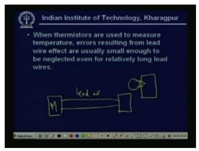
Now, when the, when thermistors are used to measure the temperature, the errors resulting from the lead wires effect are usually small enough to be neglected even for
