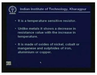
It is made of oxides of nickel, cobalt or manganese and sulphides of iron, aluminium or copper.
