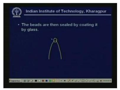
The beads are then sealed by coating it by glass. It looks like this, actually. So, two wires we will take. I should, I will draw it here. I should draw it here, so two wires are
