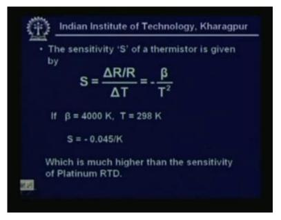
The sensitivity S of a thermistor is given by S is equal to delta R by R by delta T. If you can derive, then I will get minus beta by T square. If beta, for an example if beta is equal to 4000 Kelvin and T is 298 Kelvin, S, we will find the S, the value of the S to be equal to minus 0.045 per Kelvin and this is much higher than the sensitivity of Platinum RTD. Platinum RTD is not that this sensitive, because both are resistance, resistive sensors.
