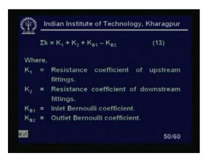
Small k equal to K 1 plus K 2 plus KB1 minus KB 2 this is equation number 13 what is that? Where K 1 is the resistance coefficient of upstream fittings; K 2 is the resistance coefficient of downstream fittings. KB 1 is inlet Bernoulli's coefficient and KB 2 outlet Bernoulli's efficient. So, this will may give summation k, right.
