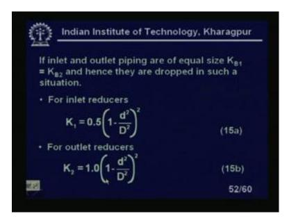
If inlet and outlet pipings are of equal size then we can say inlet and outlet piping to the valve or to and from the valve then KB 1 will be KB 2 and they are dropped in such a situations. So, for inlet reducers I can write K 1 equal to 0.51 minus d square upon capital D square to the power whole square. And for outlet reducers I can write K 2 equal to 1 1 minus small d square by capital D square to the power whole square and it is fifteen point b equations.
