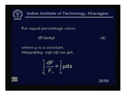
Now, for the equal percentage value it is slightly different we are defining as d derivative of F with respect to x. That means, derivative of flow with respect to fraction of the flow with respect to fraction of the stem position will be mu in to t where mu is a constant integrating equation 4 we get dF by F where varies from F to F naught and mu into dx when x to 0, right.
