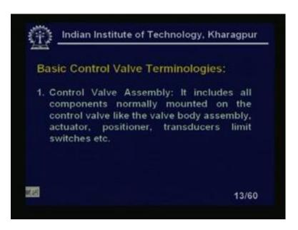
Now, basic control valve terminologies control valve assembly. It includes all the components normally mounted on the control valve like the valve body assembly, actuator positioned, transducers limit switches etc.
