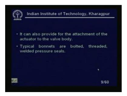
It can also provide for the attachment of the actuator to the valve body, clear. Typical bonnets are bolted threaded and welded pressured seals, because this are totally sealed otherwise there will be a problem.
