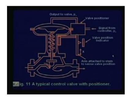
So, this is all about I am talking about this I mean valve positions and all these things you see here this arms attached to stem to sense the valve position. And this is arm it is sense the stem of the valve position this will come to parallel and these are the valve position and signal from the pc will come, right.
