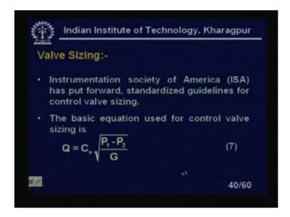
Valve sizing; instrumentation society of America ISA put forward standard standardized guideline for control valve sizing. The basic equation used for control valve sizing is q equal to Cv route over p 1 under the square p 1 minus p 2 upon G under the square route this is equation number 7.
