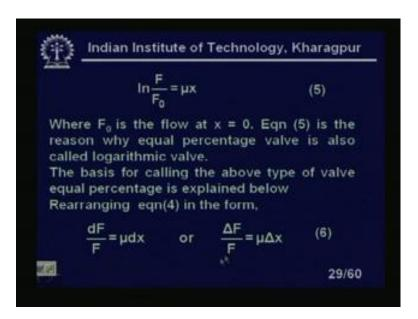
You see here 6 for sorting change in the stem position, percentage change of the flow will be constant mu. Because delta F by F by delta x will be equal to mu, which is a constant, clear? That is the reason we are calling it equal percentage valve, clear?
