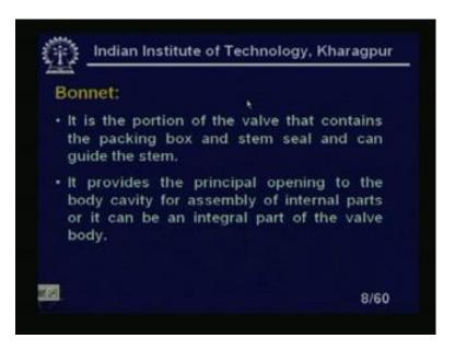
Bonnet it is the portion of the valve that contains the packing box and the stem seal and can guide the system stem, right. As I told you if I look at bonnet, this is the called the bonnet, right. It provides the principle opening to the body cavity for assembly of the internal parts or it can be an integral part of the valve body. It is can be of the integral part of the valve body.
