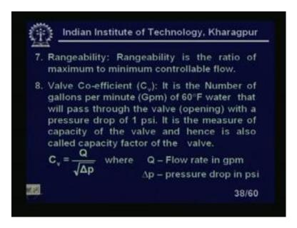
Rangeability; rangeability is the ratio of the maximum to minimum controllable flow, valve coefficient Cv. It is the number of gallons per minute of 60 degree Fahrenheit water. That will pass through the valve opening with a pressure drop of 1 psi. And it is the measure of capacity of the valve and hence is also called the capacity factor of the valve, right. Cv is equal to Q upon square root of delta p where Q will be flow rate in gallon per minute and delta p is the pressure drop in psi.
