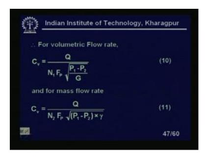
For volumetric flow rate I can write Cv Q upon N 1 F p Q upon N 1 F p under the square route P 1 minus P 2 by G is G is a specific gravity as I told you and for mass flow rate. So, we are writing Q into F p under the square route P 1 minus P 2 into gamma gamma in that case will be density.
