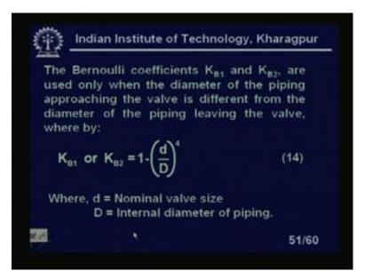
Now, the Bernoulli's coefficient KB 1 and KB 2 are used only when the diameter of the piping approaching the valve is different from the diameter of the pipe leaving the valve. If the 2 valve diameter is same pipe diameter diameter of the pipe I mean same I mean at
