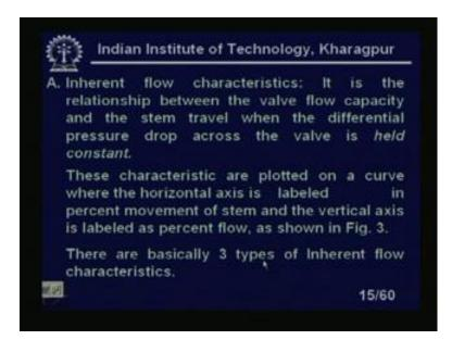
Inherent flow characteristics; it is the relationship between the valve flow capacity and the stem travel when that the stem travel as I told you is repeatedly it is a basically the percentage lift of the stem, right. That is called the stem travel. Stem travel when the differential pressure drop across the valve is held constant, right. I will repeat it is the relationship between the valve flow capacity And the stem travel when the differential pressure drop across the valve is held constant.
