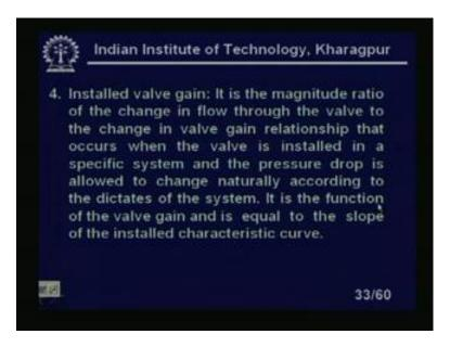
Installed valve gain it is the magnitude ratio of the change in the flow through the valve to the change in the valve gain relationship. That occurs when the valve is installed in a specific system and the pressure drop is allowed to change naturally according to the dictates of the system. Initially we have assumed the pressure drop will remain constant. It is the function of the valve gain and is equal to the slope of the installed characteristics curve.
