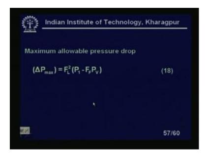
So, maximum allowable pressure drop which is to be calculated delta P max equal to Fl square which is P 1 minus Ff into Pv this is equation number 18.
