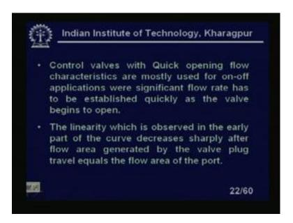
Control valves with quick opening flow characteristics are mostly used for on-off applications were significant flow rate has to be established quickly as the valve begins to flow right in on-off characteristics we need this type of thing. The linearity which is absorbed in the early part of the curve early part of the curve decreases sharply after the flow area generated by the valve plug travels equals to the flow area of the port, right.
