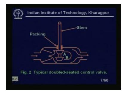
This is the the control valve previously what I have discussed it is called a single seat valve. But here we have a double seat valve, the double seat valve has a some I mean I have not drawn the full. I have drawn only the stem and all these things double seated valve is also necessary for many applications, fine.
