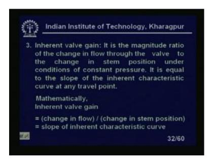
Inherent valve gain, it is the magnitude ratio of the change in the flow through the valve to the change in the stem position under condition of the constant pressure. It is equal to the slope of the inherent characteristics curve at any travel point, right. Mathematically inherent valve gain can be written as change in flow upon change in stem position or change in lift which is the slope of the inherent characteristics curve, right.
