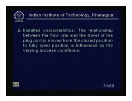
Now, we are talked about the inherent valve characteristics let us come to the installed valve characteristics or install characteristics. The relationship between the flow rate and the travel of the plug as it is moved from the close position to fully open position is influenced by the varying process conditions. This again the process, because so far we
