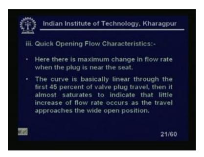
Now, third one is a quick third one of inherent valve characteristics is a quick opening flow characteristics. What is this? Let us look at. Here there is a maximum change in flow rate when the plug is near the seat. And total and slowly it will get saturated, clear. However it is very simple you see here.
