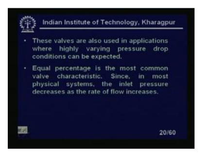
These valves are also used in applications where highly varying pressure drop condition can be expected. So, different applications are there where we are using this type of different types of controller. Equal percentage is the most common valve characteristics. Since, in most physical system the inlet pressure decreases as the rate of flow increases as the rate of flow increases inlet pressure decreases. So, that will be it will be suitable for that type of applications.
