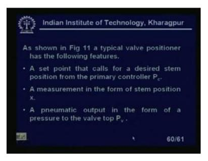
As shown in figure 11 a typical valve positioner has the following features what are the features of the valve positions? Let us look at a set point that calls for a desired stem position from the primary controller Pc. It is coming from the primary controller a
