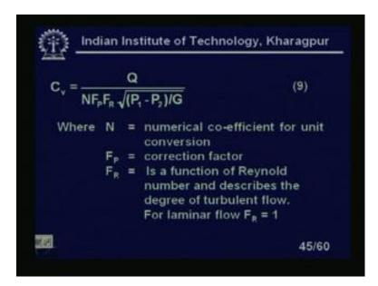
Q Cv valve discharge coefficient equal to Q upon N FPFR under the square root P 1 minus P 2 by G what is that where N is the numerical coefficient for unit conversion FP is the correction factor FR is the function of Reynold number, and describes the degree of turbulent flow for laminar flow FR equal to 1.
