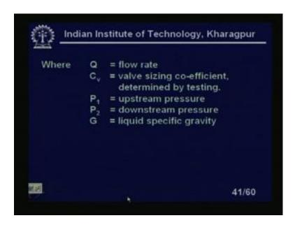
Where Q is the volumetric flow rate, Cv is the valve sizing coefficient determined by testing, P 1 is the upstream pressure, P 2 is the downstream pressure and G is the liquid specific gravity, clear?
