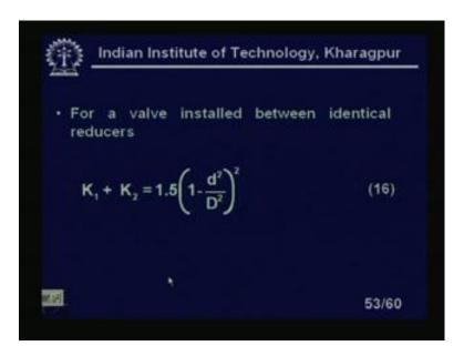
For a valve installed between identical reducers I can write K 1 plus K 2 equal to 1.5 multiplied by 1 minus d square upon small D square by capital square to the power whole square this is equation number 16.
