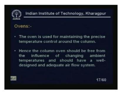
Now, ovens as I told you the oven is used for maintaining the precise temperature control around the column. Hence the column oven should be free from the influence of changing the ambient temperature and should have a well designed and adequate air flow systems. There should be good air flow systems otherwise temperature control will be difficult.
