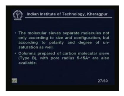
The molecular sieves separate molecules not only according to size and configuration, but according to the polarity and degree of unsaturation as well. Columns prepared from carbon molecules sieve type B with pore radius of 5 to 15 Armstrong are also available.
