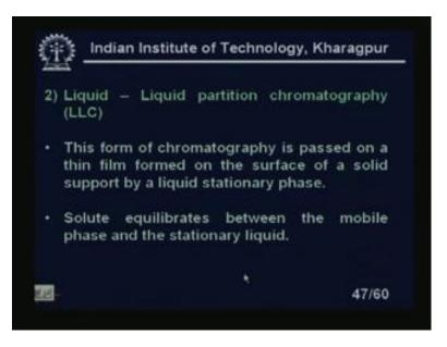
Liquid-liquid partition chromatography; this form is chromatography is passed on the thin film formed on the surface of a solid support by a liquid stationary phase clear? Solute equilibrates between the mobile phase and the stationary liquid.
