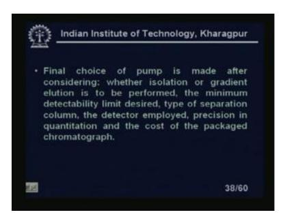
Final choice of pump is made after the considering; whether the isolation or gradient elusion is to be performed and the minimum detectability limit desired type of separation column. The detector employed precision in quantitation and the cost of the packaged chromatograph.
