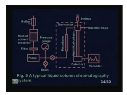
You see this is a typical liquid column chromatography the entire instrumentations we are showing here. We have a reflux systems we can see here. I am sorry you see here.
