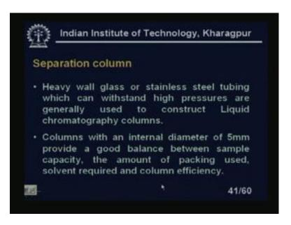
Separation column; heavy wall glass or stainless tubing which can withstand high pressures are generally used to construct liquid chromatographic columns. Columns with an internal diameter of 5 millimeter provide a good balance between the sample capacity. The amount of packing used the solvent required and column efficiency.
