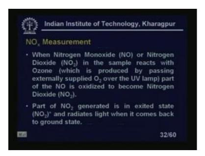
When nitrogen monoxide or nitrogen dioxide in the sample reacts with the original, which is produced by passing externally supplied O2 over UV lamp part of the NO is oxidized to become a nitrogen dioxide right. Part of the NO2 generated in is in the exited state exited states actually we are defining it by this please note.
