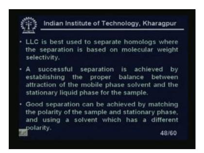
LLC is best used to separate homologs where the separation is based on the molecular weights selectivity right. A successful separation is achieved by establishing the proper balance between the attraction of the mobile phase solvent and the stationary liquid phase for the sample. Good separation can be achieved by matching the polarity of the sample and the stationary phase and using a solvent which has different polarity.
