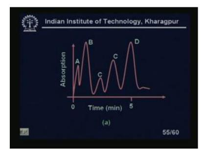
You see this is a typical chromatograph which we got at the detectors or the strip chart recorders although we have different components, we have a gas we have a components of A B C D, this will be I am sorry. So, this will be A B C; this will be D different components and this will be E right.
