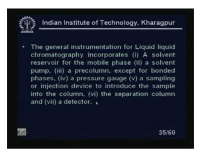
The general instrumentation for liquid liquid chromatography incorporates a solvent reservoir for the mobile phase a solvent pump, a precolumn except for the bonded phases; a pressure gauge; a sampling or injection device to introduce a sample in to the column; a separation column and a detector.
