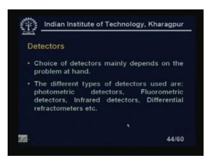
Detectors choice of detectors mainly depends on the problem at hand. The different types of detectors used we have photometric detectors, fluorometric detectors, infrared detectors, differential refractometers.
