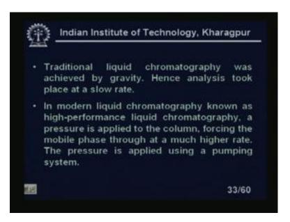
Traditional liquid chromatography was achieved by gravity hence analysis took place at a slow rate. In modern liquid chromatography known as the high performance liquid chromatography, a pressure is applied to the column forcing the mobile phase through the through at a much higher rate and the pressure is applied using a pumping systems. Instead of gravity we are using pumping system.
