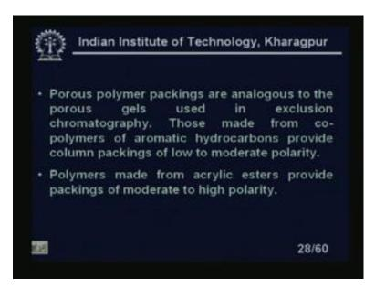
Porous polymer packings are analogous to the porous gels used in the exclusion chromatography. Those made from the copolymers of aromatic hydrocarbons provide column packings of low to moderate polarity. Polymers made from the acrylic esters and provide the packing of moderate to high polarity.
