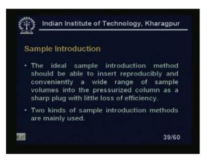
Sample introduction; the ideal sample introduction method should be able to insert reproducibly and conveniently a wide range of sample volumes into the pressurized column as a sharp plug with little loss of efficiency. Two kinds of sample introduction methods are mainly used one is the syringe injection.
