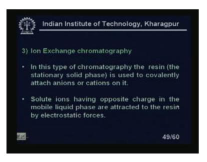
Ion exchange chromatography; here in this type of chromatography the resin the stationary solid phase is used to covalently at attach anions or cations on it, right. Solute ions having opposite charge in the mobile liquid phase are attracted to the resin by electrostatic forces right.
