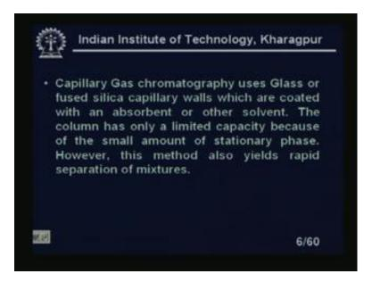
Now, capillary gas chromatography uses a glass or fused silica capillary walls which are coated with an absorbent or other solvent. And the column has only a limited capacity because of the small amount of stationary phase. However, this method also yields rapid separation of the mixtures right.
