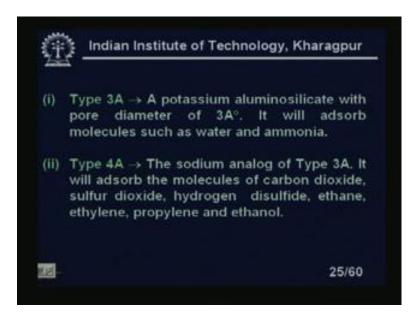
Type 3 A; a potassium aluminosilicate with the pore diameters of 3 Armstrong. It will absorb the molecules such as water and ammonia. It will absorb the molecules of water and ammonia. Type 4 A; it is a sodium analog of type of 3 A; it will absorb the molecules of carbon dioxide, right. Sulfur dioxide, hydrogen disulfide, ethane ethylene, propylene and ethanol, right.
