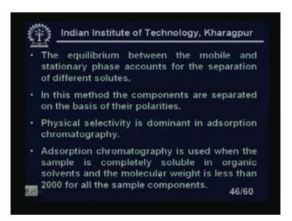
The equilibrium between the mobile and the stationary phase accounts for the separation of the different solutes. In this method the components are separated on the basis of their polarities. Physical selectivity is dominant in adsorption chromatography. Adsorption chromatography is used when the sample is completely soluble in organic solvents and the molecular weight is less than 2000 for all the sample components. We have for more than 2000 we have some different methods.
