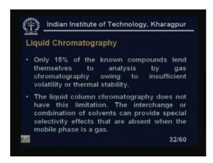
Liquid chromatography let us know only 15 percent of the known compounds lend themselves to the analysis by gas chromatography owing to the insufficient volatility of thermal stability. This is the most important the gas should not vaporize every time we have said right. The liquid column chromatography does not leave the limit this limitation. The interchange or combination of the solvents can provide special selectivity effects that are absent when the mobile phase is a gas.
