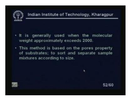
It is generally used when the molecular weight approximately exceeds 2000s in case where it is less than 2000 we have adsorbent method here we have a molecular exclusion. I mean gas chromatography which is used for the molecular when the molecular weights more than, approximately exceeds 2000. This method is based on the pores property of the substrate to sort and separate sample mixtures according to size.
