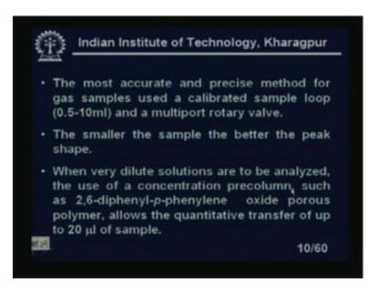
The most accurate and precise method for the gas sample used a calibrated sample loop of 0.5 10 milliliters and a multi port rotary valve. So, different types of rotary valves will be used in the case of in the case of this type of sample injections because sometime we need a valve. So, the precise amount can be injected. The smaller the sample the better the peak shape that I told you the peak shape should be better and better and how the peak should look like let us look at that.
