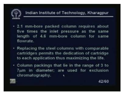
2.1 millimeter bore packed column requires about five times the inlet pressure or as the same length of the 4.6 millimeter bore column for the same flow rate. Replacing the steel columns excuse me steel columns with comparable cartridges permits the cartridges
