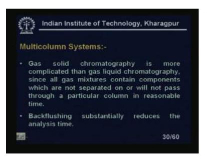
Multicolumn systems gas solid chromatography is more complicated than the gas liquid chromatography. Since all gas mixtures contain components which are not separated on or will not pass through a particular column reasonable time. Backflushing substantially it reduces the analysis time.
