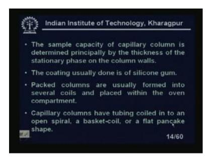
The sample capacity of capillary column is determined principally by the thickness of the stationary phase on the column walls. The coating usually done is of silicon gum. Packed columns are usually formed into several coils and placed within the oven compartments.
