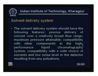
Solvent delivery system; the solvent delivery system should have the following features; precise delivery of solvent over a relatively broad flow range; maximum pressure attainable. Compatibility with other components in the high; performance liquid, chromatography system, compatibility with the wide choice of the solvents and low noise levels in the detector resulting from any pulsations.
