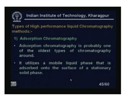
Types of high performance liquid chromatography methods; adsorption chromatography; adsorption chromatography is probably one of the oldest type of chromatography around. It utilizes the mobile liquid phase that is adsorbed onto the surface of the stationary solid phase.
