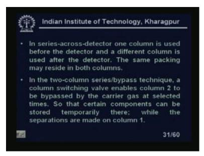
In series-cross-detector across detector one column is used before the detector and a different column is used after the detector. The same packing may reside in both the columns. In two column series bypass technique a column switching valve, valve enables
