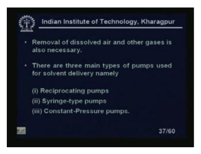
Removal of the dissolved air and other gasses is also necessary. So, there are three main types of delivery pumps used for solvent delivery system namely reciprocating pumps, syringe-type pumps and constant-pressure pumps.
