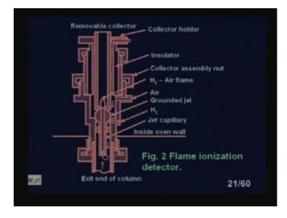
Now, you see this is the flame ionization detector as I told you this flame ionization detector is one of the detectors since the different components in the flame ionization detectors. This is a exit end of the column let us look at you see here a jet capillary is there it is the I mean flowing through this one. This is the hydrogen air flame and air is
