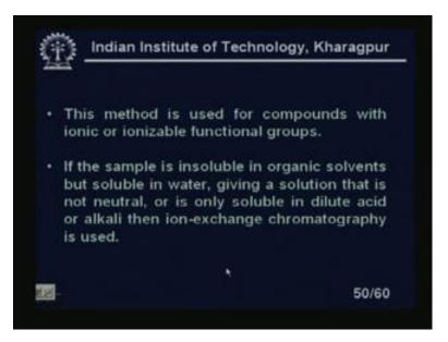
This method is used for compounds with the ionic and ionizable functional groups. If the sample is the insoluble in the organic solvents, but soluble in water giving a solution that
