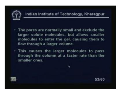
The pores are normally small and exclude the larger solute molecules, but allows smaller molecules to enter the gel causing them to flow through the larger volume. This causes
