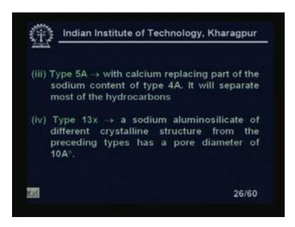
Type five A; with calcium replacing part of the sodium content of type four A and it will separate most of the hydrocarbons. In many I mean this particular industry this is very
