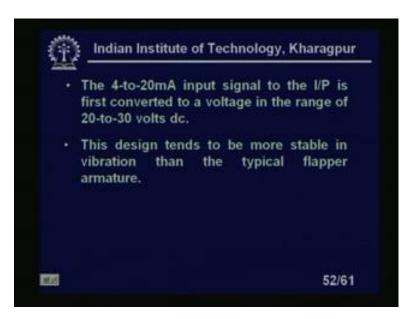
The 4 to 20 milliampere of current input signal to the I to P is first converted to voltage in the range of 20 to 30 volts dc right. Now, this voltage is actually given to the flapper
