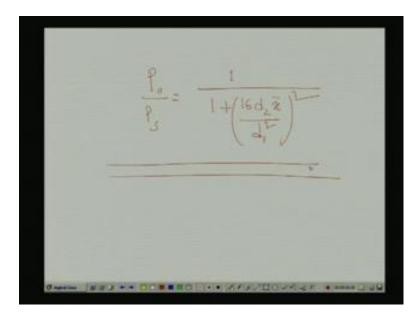
Po by Ps equal to 1 upon 1 plus 16 d square d 2 here I write x bar here I write by d 1 square to the power whole square this is our equations. This is actually we have explained in our ultimate equations; that means, normalized output how the normalized output is relates to the displacement.
