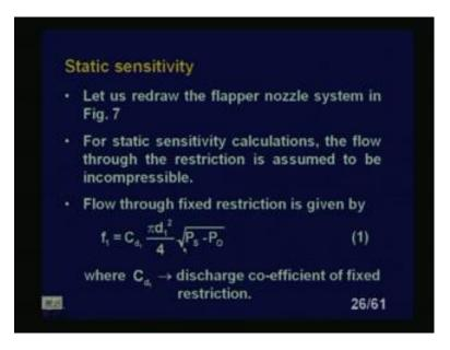
So, Cd 1 is the discharge coefficient of fixed restrictions; that means, supply side restrictions Ps Po you know there is a output pressures and Ps is the our supply pressure.
