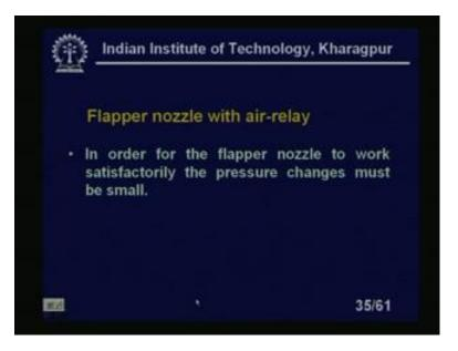
Flapper nozzle with air relay this is another important thing in order for the flapper nozzle to work satisfactorily the pressure changes must be small. We have seen that the pressure change must be small I mean very small. This is by using an air relay an excellent thing you see the how it works?
