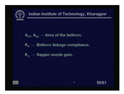
Say 1 Ab 1 Ab 2, the area of the bellows Kb the bellows linkage compliance Km the flapper nozzle again.
