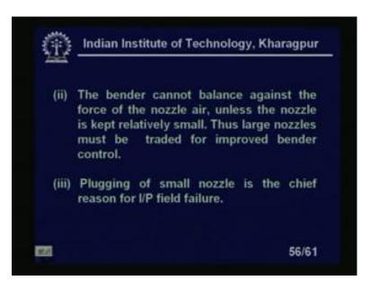
The bender cannot balance against the force of the nozzle air unless the nozzle is kept relatively small thus large nozzles must be traded for improved bender control. Plugging of small nozzles is a chief reason for I to P field failure.
