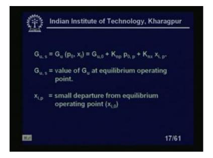
So, we can write Gus equal to Gu Po Xi equal to Guo plus Knp P o p plus Knx Xi p. Gus is the value of Gu at equilibrium operating point and Xip the small departure from the equilibrium operating point.
