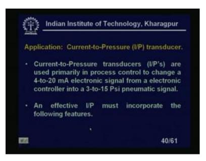
Now, current to pressure convertor I to P convertor as I told you this is very widely used in industry. Current to pressure transducers are used primarily in the process control to change a 4 to 20 million ampere of electronic signal from a electronic controller into 3 to 15 psi for a pneumatic controller. An effective I and P most incorporate the following features.
