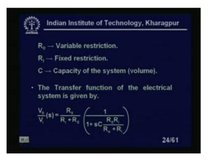
Where is Ro? Is a variable restriction Ri is the fixed restriction. What is the fixed restriction? That is at the input the side the restrictions, which we are getting that is the fixed restrictions. Then C is the capacity of the systems that is the volume, so these actually makes our flapper nozzle system. The transfer function are easily we can find
