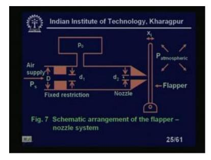
You see here let us I mean we can redraw the equation the flapper nozzle systems. We have just redrawn we have change the position it does not matter it can be flapper can be this side this can be that side. I mean the nozzle can be the supply air from this side or that can be that side it does not matter much. You see the same the circuit I mean the flapper nozzle diagram, because we refer to this that is the reason why I have redrawn this in the figure 7.
