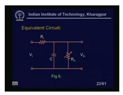
You see this is out flapper nozzle systems. This Ri and C Ri is the input side; that means, supply side restrictor representing. And this is Ro is the load side restrictors I am giving Vi I am Vo this is a electrical representations of our flapper nozzle system.
