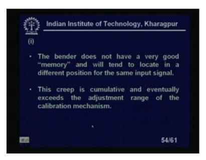
The bender does not have a very good memory; that means that it has a creep which memory means it is called in the systems and will tend to locate in a different position for the same input signal. That means, creep is cumulative cumulant and eventually it exceeds the adjustment range of the calibration mechanism.
