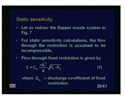
Now, let us how will I compute the static sensitivity of the flapper nozzle systems. Let us redraw flapper nozzle system as I told you in the figure 7. That just we have redrawn the figure it is same as the figure 7 there is no difference. For static sensitivity calculation the flow through the restriction is assumed to be incompressible flow through the restrictor is incompressible in first we have assume. In many field dynamics we thought we have seen that we have assumed like this 1.
