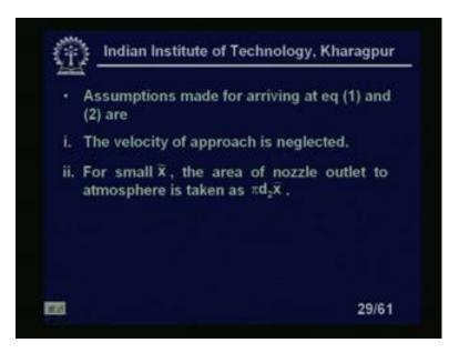
Now, assumptions made for arriving at equation one and two I mean how there are what are the assumptions basic assumptions. We have taken the velocity of approach is neglected for small x bar the area of the nozzle outlet to the atmosphere is taken as pi d 2 into x bar instead of pi d 2 square by 2 pi d 2 square by 4. We have taken pi d 2 into x
