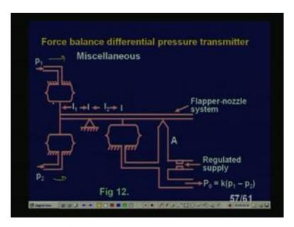
Force balanced differential pressure transmitter; you see this we have seen the 2 pressures are coming this side. You can see here two pressures I mean P 1 sorry this P 1
