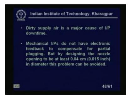
Dirty supply air is the major cause of I to P downtime mechanical I P's do not have electronic feedback to compensate for partial plugging. But designing the nozzle opening to be at least point 0 4 centimeter; that means, 0.015 inch in diameter this problem can be avoided.
