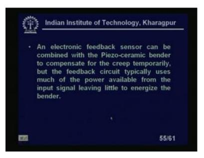
An electronic feedback sensor can be combined with the piezo-ceramic bender to compensate for the creep temporarily for the... But the feedback circuit typically uses such more power available from the input signal having little to energize the bender.
