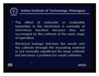
The effect of reducible or oxidizable impurities in the electrolyte is normally of shortterm duration, because they are scavenged by the cathode at the early stage of operation. Electrical leakage between the anode and cathode through the insulating material is not normally significant for leakage for large cathode, but becomes a problem for a small cathodes.
