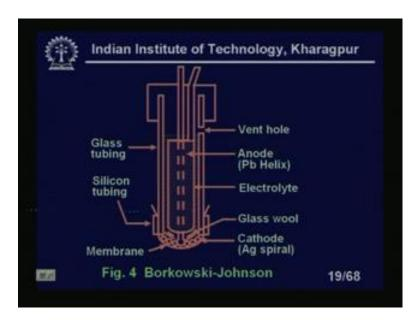
You see here, we have a glass tubing anode is there which is helix, then we have electrolyte. We have a glass wool, there a cathode which is I mean, silver spiral sorry and we have a membrane silicon tubing is there. So, this is our glass tubing and 2 2 wires are coming out.
