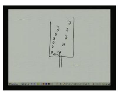
That I have a vessels and I am purging, oxygen through this one. So, bubble will go out, like this one, it will go the air bubble will go. So, it will purge along this one. So, this type of this may cause problem in other type of dissolve oxygen probe, it will not make a problem in this probe. Let us go back when vertically, inserted in an air spurged cylinder vessel the Mackereth probe exhibited response free from any effects of air bubbles.
