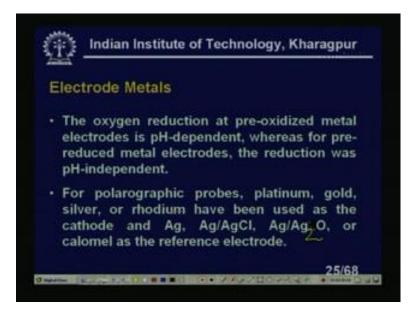
The oxygen reduction at pre-oxidized metal electrode is a p H dependent, where as for pre-reduced metal electrodes the reduction was p H independent. For polarographic probes, platinum gold silver and or rhodium have been used as a cathode and silver and silver silver chloride, silver silver dioxide. This A g 2 O please note, it is not A g 2 it is A g 2 will be in subscript. So, it is like this, so it will be 2 O sorry 2 O. So, I can or calomel as a reference electrode is used.
