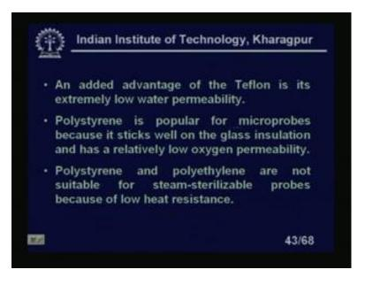
An added advantage of the teflon is, it is extremely, low water permeability, so this is another advantage of the teflon. Polystyrene is popular for microprobes, because it sticks well on the glass insulation and has a relatively, low oxygen permeability. Polystyrene and polyethylene are not suitable for steam sterilizable probes, because of low heat resistance. So, the problem is there on one side is a low oxygen permeability and the other side it has a low heat resistance.
