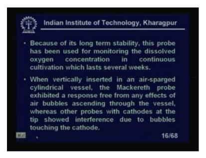
Because of it is long term stability, this probe has been used for monitoring the dissolved oxygen concentration in continuous cultivation, which lasts several weeks in some cases, I said 72 hours in some cases, it is can be continue over a week. So, in that type of situation, this electrode is very much suitable, though the response time is very. I mean, is quite bad, I should say which does not matter, because I will not sample, I will not measure every minutes.
