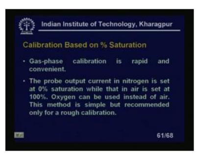
Calibration based on percentage saturation. Gas phase calibration is rapid and convenient. The probe output current in nitrogen is set at 0 percent saturation while that in the air that in the air is set at 100 percent. Oxygen can be used instead of air this method is simple, but recommended only for a rough calibrations.
