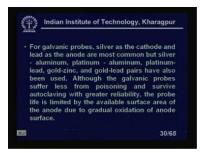
For galvanic probes the silver as the cathode and lead as the anode are most common. But sliver aluminum platinum aluminium platinum lead gold gold lead pairs have also been used although the galvanic probes suffered less from poisoning and survive autoclaving with greater reliability. The probe life is limited by the available surface area, of the anode due to gradual oxidations of the anode surface, this is again problem.
