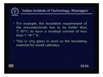
For example, the insulation requirement of a the microelectrode has to be better than ten to the power 7 into the power 10 ohm. That means, you can see it is around coming around 70 gig ohm and have a residual current of less than 10 to the power 11 ampere. That means, 0.1 picoampere. So, it is quite small this is why glass is used as the insulating material for small cathodes it will give you very less residual current.
