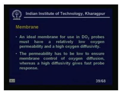
Membrane: an ideal membrane for use in D O 2 probes must have a relatively, low oxygen permeability, high oxygen diffusivity. The permeability has to be low to ensure the membrane control of the oxygen diffusion whereas, the high diffusivity gives a fast probe response, so you have to make a compromise.
