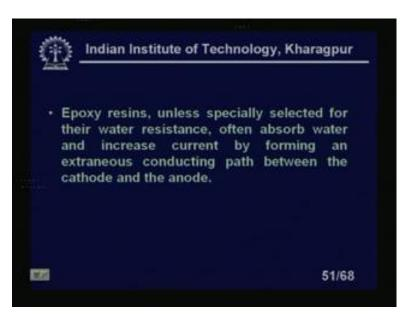
Epoxy resins, unless specially selected for their water resistance, often absorb water and increase current by forming an extraneous conducting path between the cathode and the anode. This is again problem.
