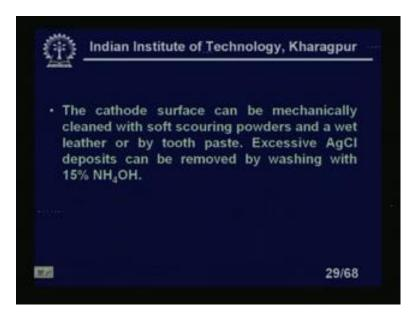
The cathode surface can be mechanically, cleaned with soft scouring powders. So, if you regularly, clean it with a cleaning powders and wet leather or by tooth paste. So, excessive silver chloride deposits can be removed by washing with sodium. I mean, ammonium hydroxide 15 percent ammonium hydroxide is possible. This I told you from the very beginning, where we were at cleaning of the electrodes.
