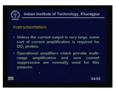
Instrumentation: let us look at... Unless the current output is very large, some sort of current amplifications is required for D O 2 probes. So, we know various types of current amplification that, single condition is we can do, it has improved a lot. So, that is not a problem, operational amplifiers, which provide multi-range amplifications and current suppression are normally, used for this purpose.
