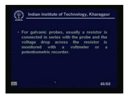
For galvanic probes, usually a resistor is connected in series with the probe and the voltage drop across the resistor is monitored with a voltmeter or a potentiometric recorder.
