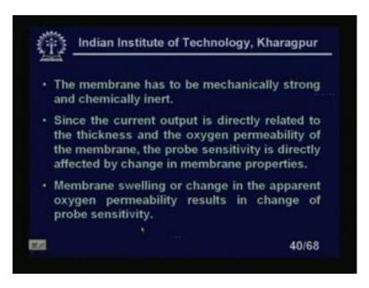
The membrane has to be mechanically, strong and chemically, inert right; that means, mechanically strong means; it can, should withstand the high pressure. It can should I mean, in a position to withstand high temperature at least 120 degree centigrade. Little more than 1 atmosphere, it is to be I mean, because if you do for autoclaving. So, this I
