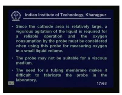
So, need for a tubing membrane makes, it difficult to fabricate the probe in the laboratory this is another problem, which is like in the Clarke electrodes is very simple to make.
