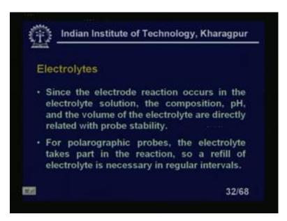
Electrolytes since the electrode reactions, occurs in the electrolyte solution the composition comma p H and the volume of the electrolytes are directly related to the probe stability. For polarographic probes the electrolyte takes part in the reaction, so a refill of electrolyte is necessary in the regular intervals. This is a very important thing is very difficult so that what we have to do? A, we have to use a reservoir, we will discuss in the next slide.
