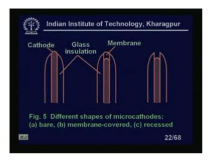
You can see here, so 5 a b c all these are this is a bare this is glass insulation. This is a cathode, this is a membrane, and this is like this one recessed membrane covered and recessed 3 difference we have shown.
