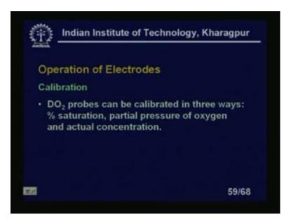
Now, operations of the electrodes, let us look at calibration this is most important thing D O 2 probes can be calibrated in three ways saturations in partial pressures of oxygen and actual concentration.
