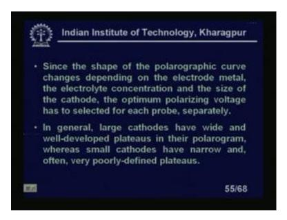
Since the shape of the polarographic curve changes depending on the electrode metal the electrolytic concentration and the size of the cathode the optimum polarizing voltage has to be selected for each probe separately. In general the large cathodes have wide and well developed plateaus in their polarogram whereas; small cathodes have narrow and often very poorly defined plateaus.
