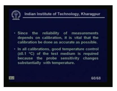
Since the reliability of measurements depends on the calibration it is vital that the calibration done as accurate as accurate as possible right. So, the calibration will show the some equation by which we can make the calibrations. In all calibrations good temperature control; that means, 0.1 degree centigrade plus minus one of the test medium is required, because the probe sensitivity changes substantially with temperature, right.
