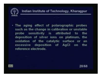
The aging effect of the probes, such as the change in calibrations or unstable probe sensitivity is attributed to the depositions of silver ions on platinum, and the oxidations of the catalytic surface or an excessive deposition of silver chloride on the reference electrode. (Refer Slide Time: 29:08)
