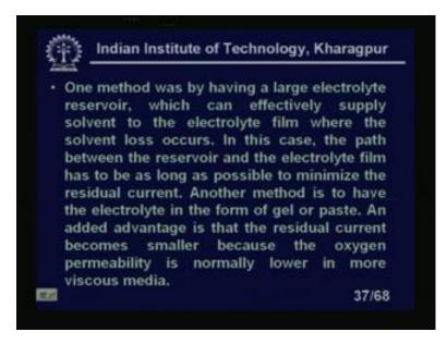
One method; by having a large electrolyte reservoir as I told you which can effectively supply solvent to the electrolyte film where the solvent loss occurs. In this case the path between the reservoir and the electrolyte film has to be as long as possible to minimize, the residual current. Another method is to have electrolyte in the form of gel or paste and added advantage is that the residual current becomes smaller, because the oxygen permeability is normally, lower in more viscous medium.
