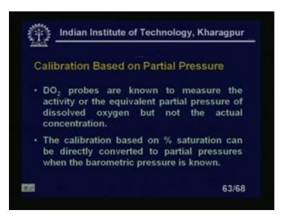
Calibration based on partial pressure D O 2 probes can known to measure the activity of the equivalent partial pressure of the dissolved oxygen, but not the actual concentrations. We actually calibrate in terms of actual concentration, but actually it is measuring the partial pressure. The calibration based on percentage saturation can be directly converted to partial pressures when the barometric pressure is known right.
