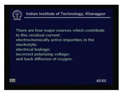
There are 4 major sources which contribute to the residual current: electrochemically active impurities in the electrolyte, electrical leakage, incorrect polarization voltage, back diffusions of oxygen.
