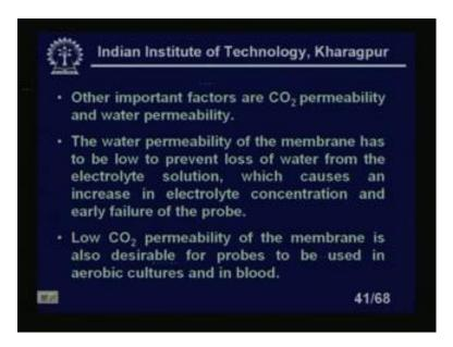
Other important factors are C O 2 permeability, and water permeability the water permeability, of the membrane has to be low to prevent loss of water from the electrolyte solution, which causes an increase in the electrolyte concentrations. And early failure of the probe low C O 2 permeability of the membrane is also desirable for probes to be used in aerobic cultures. And in blood sometimes, under the means, of oxygen concentrations and that is also important.
