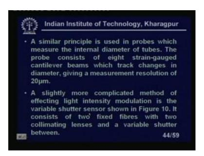
A similar principle is used in probes, which measure the internal diameter of the tubes the probe consists of 8 strain gauged cantilever beams which track changes in diameter giving a measurement of resolutions of 20 micron right. So, in many situations we need this term. A slightly more complicated method of effecting light intensity modulation is the variable shutter sensor shown in ten where it consists of 2 fixed fibres with 2 collimating lenses and a variable shutter between.
