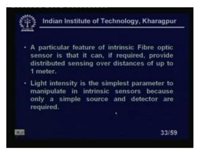
A particular features of intrinsic fibre optic sensor is that, it can if required provide distributed sensing over the distances of up to 1 meter. Light intensity is the simplest
