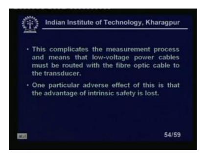
This complicates the measurement process and means that the low voltage power cables must be routed with the fibre optic cable to the transducer. One particular adverse effect of this is that the advantage of intrinsic safety is lost because we are using the electrical system. So, that intrinsic safety which we talked about, so much of the optical fibre that is lost there.
