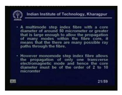
Now, a multimode step index fibre with a core diameter of around 50 micrometer. Or greater that is larger enough to allow the propagation of many modes in many incident situations. Many modes within the fibre core, it means that the there are many possible
