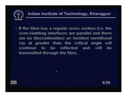
If the fibre has a regular cross section that is the core cladding interface are parallel. There are no discontinuities an incident, incident meridional ray at greater than, the critical angle will be continue to be reflected. And will be transmitted through the fibre that is a very good.
