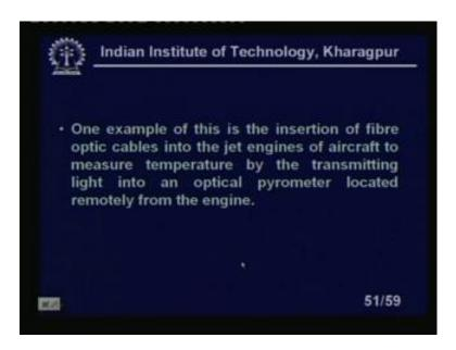
One example of this is insertion of fibre optic cables into the engines of aircraft to measure temperature by the transmitting light into an optical pyrometers located remotely from the engine.
