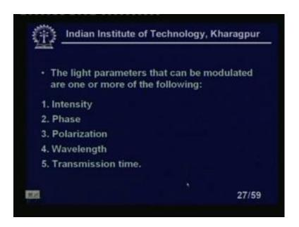
The light parameters that, can be modulated are one or more of the following intensity can be modulated, phase can be modulated, polarization will be there wavelength can be modulated and transmission time. ((Refer Time: 36:42)) see in most of the case, we find
