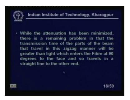
While the attenuation has been minimized, there is a remaining problem in that the transmission, time of the parts of the beam. That travel in the zigzag manner will be greater, than the light which enters the fibre at 90 degrees to the face. And so travels in a straight line to the other end. So obviously, if it falls on a 90 degree is not, it if the light falls on a 90 degree, because we are talking about. So, much you see if I take a dark 1.
