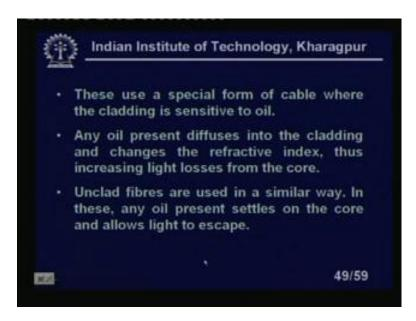
So, that case what is the principle you see these uses a special form of cable where the cladding is sensitive to oil any oil presents diffuse diffuses into the cladding. So, oil will
