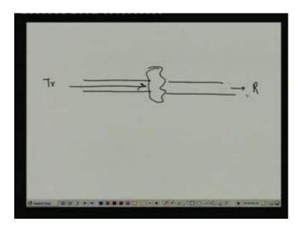
And sorry let me take it is I have a fibre here and I have a fibre here. So, I am getting the smokes comes here what will happen the intensity of light received at this end this is the transmitter and this is our receiver. So, what will happen intensity of the light will be decreased since the smoke will; obviously, decrease the intensity of light. So, the; obviously, this can be used as the smoke detectors. So, it will turn on some alarm or some announciation right.
