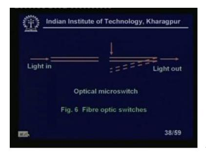
This is the fibre optic switches; that means, is optical micro switch; that means, if I the fibre bends like this one the fibre bands in this directions. So; obviously, if the light have a light sources, have a light receiver, so obviously I would not get in get a light output. So, this is all the use of optical micro switch right. So, this is also a example of fibre optic switches.
