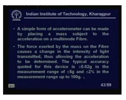
Now, a simple form of accelerometer can be made by placing a mass subject to the acceleration on a multimode fibre. The force exerted by a by the mass on the fibre causes a change in the intensity of light transmitted. And thus allowing the acceleration to be determined and the typical accuracy quoted for this device is plus minus 0.02 g in the measurement range of plus minus 5 g 6 extremely good. I should say and plus minus 2 percent in the measurement range up to 100 g.
