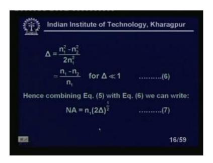
Between the core and the cladding which is defined as delta equal to n 1 square minus n 2 square by 2 n 1 square, so which we can write n 1 minus n 2 by n 1 for delta. If it is delta less, less 1 we can write like this one equation, number 6 hence combining equation 5 with equation 6. We can write that, numerical aperture is equal to n 1 2 delta to the power half, which is equation number 7.
