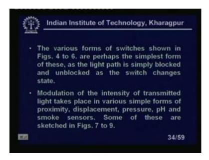
The various forms of switches shown in figure 4 to 6 are perhaps the simplest form of these as the light path is simply, blocked and unblocked as the switch changes position right changes state. Let us, look at modulation of the intensity of light of the transmitted light takes, place in various simple forms of proximity, displacement pressure pH and smoke sensors. And some of these are sketched in figurers 7 to 8.
