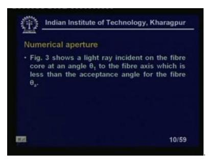
Now, what is the numerical aperture? The numerical aperture very I mean, it is a less specification of the fibres. So, must know, what is the numerical aperture? So, we will calculate here, the numerical aperture for a optical fibre. You see, figure 3 shows a light
