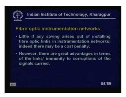
Now, fibre optic instrumentation networks looks like this that little or any saving arises of the installing the fibre optic links in instrumentation networks indeed there may be a cost penalty. Because many sensors we are using; however, there are great advantages in terms of the links immunity to corruptions of the signal carried.
