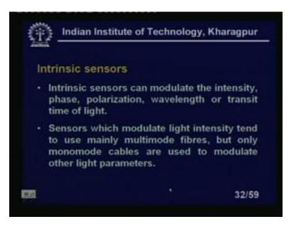
Now, intrinsic sensors, Intrinsic sensors can modulate the intensity phase polarization, wavelength or transit time of the light right. This one sensors, which modulate light intensity tend to use mainly, multimode fibres, but only the monomode cables are used to modulate to other light parameters.
