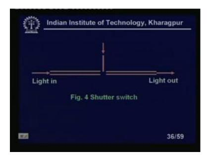
This is you see, the, a simple shutter switch; that means, if the shutter comes down; obviously, will find if the shutter comes down. The shutter comes down like, this one what will happen? You see there it will modulate the light, because if the light is coming intensity would not get in here. So, this is this is a shutter switch.
