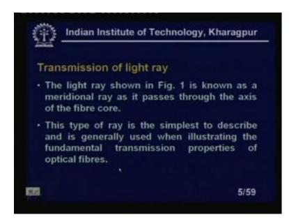
Transmission of light ray; the light ray shown in figure one this just the previews figure known, as a meridional ray as it passes through the axis of the fibre core. If cores, the fibre cores, we will call meridional ray this type of ray is the simplest to describe and is generally used when illustrating the fundamental transmission properties of the optical fibre. This always we use these fundamental transmission properties of the optical fibre.
