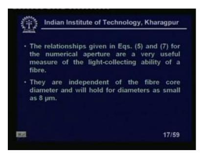
The relationships given in equation 5 and 7 for the numerical apertures are a very useful measure of the light collecting ability of a fibre, because we a must know accordingly.
