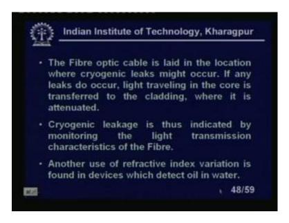
The fibre optic cable is laid in the location where cryogenic leaks might occur. If any leaks do occur light traveling in the core is transferred to the cladding, where it is attenuated. Cryogenic leakage is thus indicated by monitoring the light transmission characteristics of the fibre. Another use of the refractive index variation is found in the devices which detect oil in water in many case it is nesscery to detect.
