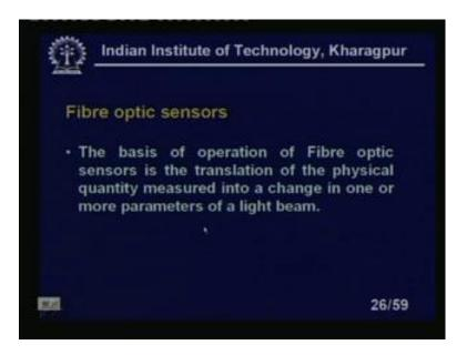
Now, let us come to the fibre optic sensors. Now, there are basis of the operation of the fibre optic sensors is the translation of physical quantity measured into a change in one of the ((Refer Time: 36:19)) or more parameters of a light beam.
