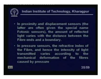
Let us look at in proximity and displacement sensors the latter are often given to the special name Fotonic sensors. And the amount of reflected light varies with the distance between the fibre ends, and a boundary in pressure sensors. The refractive index of the fibre and hence the intensity of light transmitted varies, according to the mechanical deformation of the fibres, caused by the pressure, we will show some example.
