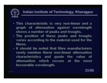
This characteristics is very non-linear and a graph of attenuation, against the wavelength shows a number of peaks and troughs the position of these peaks. And troughs varies according to the material used for the fibres, it should be noted that the fibre manufactures, rarely mention these non-linear attenuation characteristics. And quote the value of attenuation, which occurs at the most favorable wavelength.
