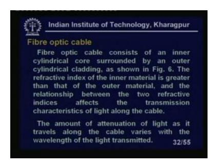
Fibre optic cable fibre optic cable consists, of an inner cylinder core surrounded by an outer cylindrical cladding as shown in figure 6. What is that figure 6? Let us look at a little far it went.
