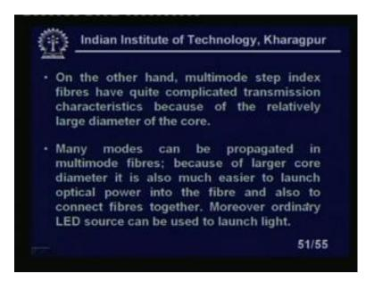
On the other hand multimode step index fibers have quite complicated transmission characteristics, because of the relatively large diameter of the core. Many modes can be propagated in the multimode fibres because of the larger core diameter. It is also much easier to launch optical power into the fibre also that connect the fibres together 2 fibre can be easily connected by together. Moreover ordinary LED source can be used to launch light that is most important I do not need laser.
