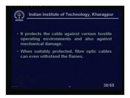
It protects the cable against various hostile operating environments also against, mechanical damage. So, mechanical damage, so that it will give you this, protections will give you that type of things, when suitably protected the fibre optic cables can even with stand the flames, if you engulfed by the flames fibre optic cables. If we have observed that, the fibre optic cables can survive it is impossible, the cases of the copper cable and all those things.
