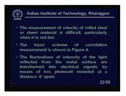
The measurement of velocity of rolled steel of sheet material is difficult, particularly, when it is red hot. The basic scheme of the correlation measurement is shown in figure 4 which have already shown. The fluctuations of intensity of the light reflected from the metal surface. Are transformed in to electrical signals by means of 2 photocells mounted at a distance d apart.
