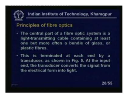
Principle of fibre optics; the central part of a fibre optic system is a light transmitting cable containing at least 1, but more often a bundle of glass or plastic fibres. This is terminated at each end by a transducer as shown in figure 5 at the input end. The transducer converts the signal from the electrical from into light, right.
