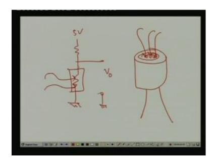
I can take a right. So, I am giving a 5 volt here, and this is my photo resistors light is falling on this looks likes as I told you earlier its capsulations. So, it is looks like this 2 leads are coming up, you can see the photo resistor here. Lights are falling on this right and this voltage; obviously, what will and if the light falls, you will find that this voltage will change right. So, if I measure, because this resistance will change. So, this voltage Vo across this will also change.
