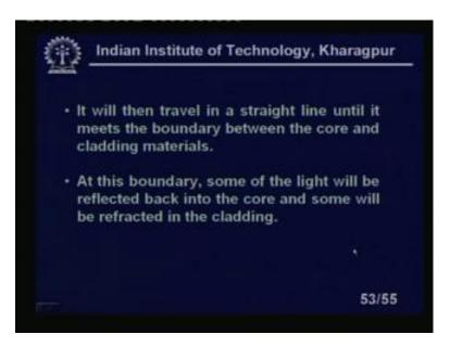
It will then travel in a straight line until it meets the boundary between the core and cladding materials. At this boundary some of the light will be reflected back into the core and some will be refracted in to the cladding, right.
