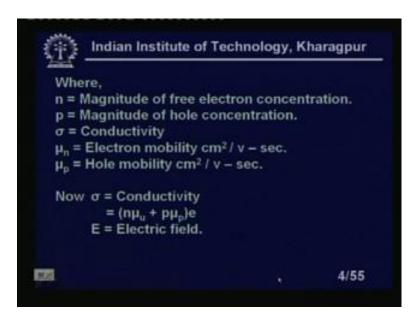
Where n is the magnitude of free electron concentration, p is the magnitude of hole concentration, sigma is the conductivity, mu n is the electron mobility in centimeter square of an by volt second and mu P is a hole mobility in centimeter square per volt second. Now, sigma conductivity will be given by n mu n this is mu n this is mu n p plus mu p multiplied by e, where e is the electronic charge E is electric field.
