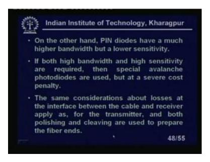
On the other hand, PIN diodes have much higher bandwidth, but has a lower sensitivity we need a amplification obvious that is not a problems. So, we can have a amplifier. In both high bandwidth and high sensitivity are required then the special avalanche photodiodes are used. But at a severe cost the same considerations about losses at the interface between the cable and receiver apply as for the transmitter and both polishing and the cleaving are used to prepare the fiber ends.
