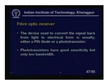
Fibre optic receivers device used to convert the signal back from light to the electrical form is usually either a PIN diode or a phototransistors right. Photo PIN diode is more popular use. Phototransistors have good sensitivity, but only low band width the bandwidth of the photo transistors is very small.
