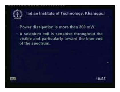
Power dissipation is more than 300 milli watt and a selenium cell. Selenium is also used as a photo resistor; selenium cell is sensitive throughout the visible and particularly, towards the blue end of the spectrum right.
