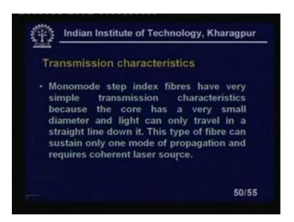
Transmission characteristics: Let us look at the monomode step index fibre have very simple transmission characteristics, because the core has a very small diameter the light can only travel in a straight line down it? This types of fibre can be sustain only one mode of propagation and equivalents requires coherent laser source that is a problem, because light will be transmitted in straight line.
