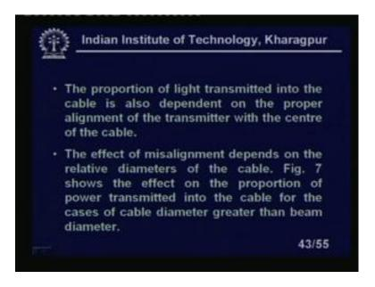
The proportion of the light transmitted into the cable is also dependent on the proper alignment of the transmitter with the center of the cable right. The effect of the misalignment depends on the relative diameter of the cable. And figure 7 shows the effect on the proportion of power transmitted into the cable for the cases of cable diameter greater than the beam diameter.
