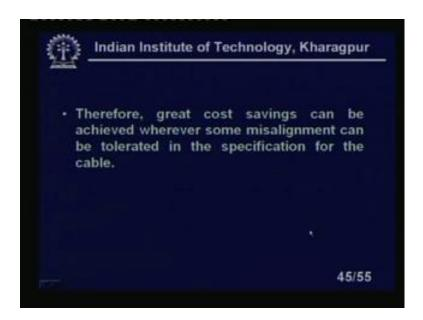
Therefore the great cost savings can be achieve wherever some misalignment can be tolerated. That is the reason multimode fibre is always preferred over the monomode fibre is little misalignment will not affect much.
