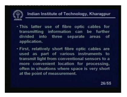
The later use of the fibre optic cables for transmitting information can be further divided into 3 separate areas of application. First relatively short fibre optic cables are used as part of the various instruments to transmit light from the conventional sensors to a more conventional, convenient location for processing often in situations where space is very short at the point of measurement.
