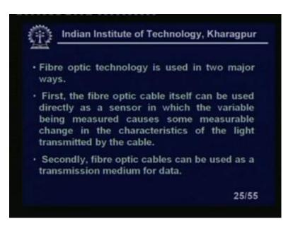
So, there is no ((Refer Time: 38:08)) as such. Fibre optic technology is used in 2 major ways, first the fibre optic cable itself can be used directly as a sensor, in which the variable being measured causes, some measurable change in the characteristics of the light transmitted by the cable. Secondly, the fibre optic cable can be used as a transmission medium for data.
