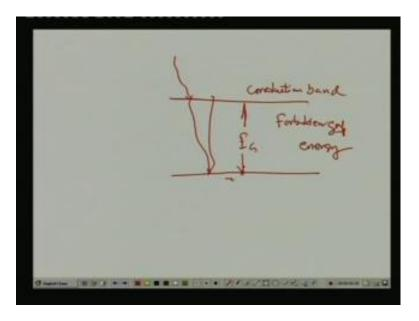
I have a conduction band. So, when the light falls, which is comes here, some of the electron; this is the forbidden gap energy EG. So, these energy these amount of energy must stored so that the electron will come to the conduction band. This is the conduction band and this is our forbidden gap energy, right.
