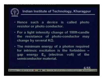
Hence such a device is called a photo resistor or photo conductor, clear? For a light intensity change of 100 foot candle the resistance of photo conductor may change by several kilo ohm, right. The minimum energy of photon required for intrinsic excitation
