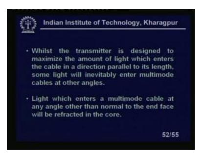
Whilst the transmitter is designed to maximize the amount of light, which enters the cable in a direction parallel to its length some light will only will inevitably enter multimode cables at the other angels which is quite obvious. And it is going to total internal refraction at coming to the end one end. Light which enters a multimode cable at any angle other than the normal to the end face will be refracted in the core right.
