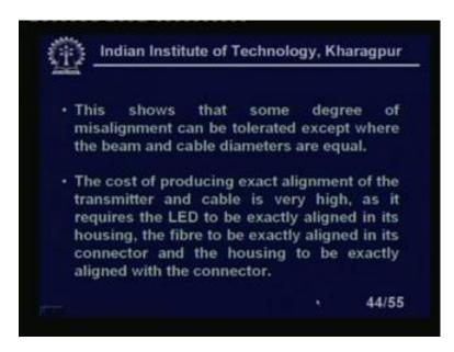
You see this shows that the some degree of misalignment can be tolerated except where the beam and the cable diameters are equal. The cost of producing exact alignment of the transmitter and the cable is very high as it requires the LED to be exactly aligned in its housing, and the fibre be exactly aligned in its connector and the housing to be exactly aligned with the connector.
