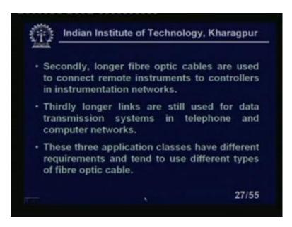
Secondly longer fibre optic cables are used to connect remote instruments to controller in instrumentation networks. Longer fibre optic cables are used to connect the remote
