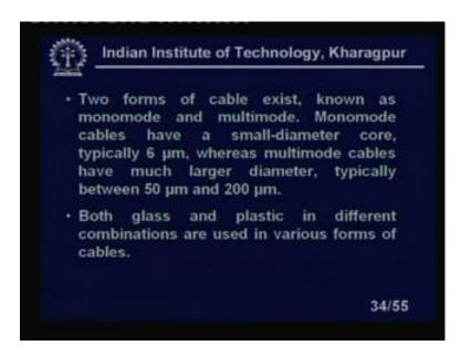
The 2 forms of cable exist, known as monomode and multimode, we have a monomode fibre. Monomode has some I mean, monomode has a I mean, launching the light in the
