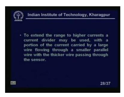
To extend the range or to the higher currents say current divider may be used with a portion of the current carried by a large wire flowing through a smaller parallel wire with
