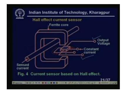
Hall Effect current sensor; this is the current sensor, based on Hall Effect you see the you see here a current. I want to measure this current, which is flowing through this wire. This is the section of the wire, which I have shown section of the wire you see this is the
