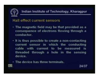
The Hall Effect current sensors the magnetic field may be that provided as a consequence of electrons flowing through a conductor. So, this is as I told you earlier, because this Hall Effect hall voltage actually developed due to the flow of electron in the semiconductor. In the conductor or in the metal or in the semiconductor, because some people say that the actually the metal that this the current flowing through the metal is due to electron was first established by the Edwin Hall.
