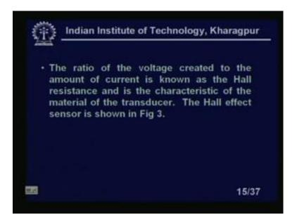
The ratio of the voltage created to the amount of current is known as the hall resistance. And the characteristics of the material of the this is the characteristics of the material of the transducers and the hall effect sensors is shown in figure 3.
