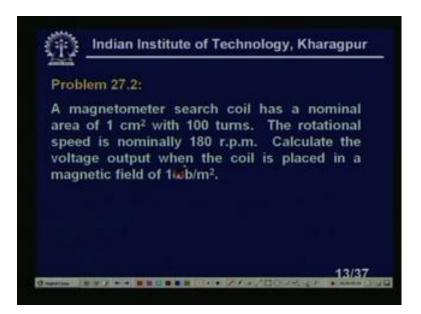
This is the problem 27.2. The problem is a magnetometer search coil has a nominal area of 1 centimeter square with 100 turns the rotational speed is nominally at 180 rpm. Calculate the voltage of output when the coil is placed in a magnetic field of 1 Weber by meter square please note it is not omega this is W right. And this will be simply W or I should take please note this is W right Weber per meter square. So, let us make the solution of this problem. So, again I am telling this is W.
