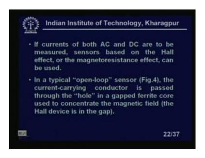
If currents of both AC and DC are to be measured sensor based on the Hall Effect or the magnetic I mean resistance magneto resistance effect can be used right. In a typical open loop sensor the current carrying conductor is passed through the hole in a gapped ferrite core used to concentrate the magnetic field that is we have shown. It is the gap ferrite
