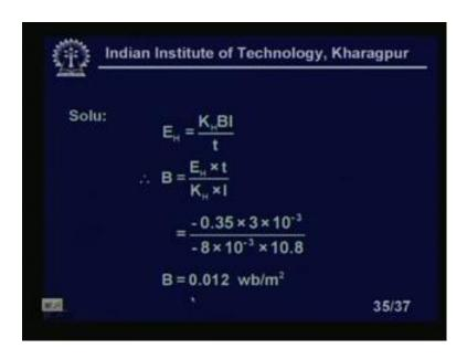
Solution EH is equal to KH is BI by t we have seen. So, B equal to KH t by KH by KH by into I. So, this you just put all these value of B. So, B equal to 0.012 Weber per meter square.
