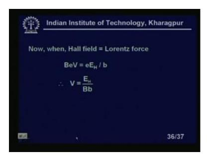
So, now when the hall field a Lorentz force must be I mean balance. So, I can write it is the moment of the velocity B is the velocity of the electrons inside the hall sensors. So, e EH by b, so V equal to EH by B by small b let me go yes. So, which will give you the speed of the electron as 9 7 2; these are all the dimensions of the hall plates, B is a dimension of the hall plates 9 7 2 2 meter per second right. With this I come to the end of the lesson 27 of industrial instrumentation.
