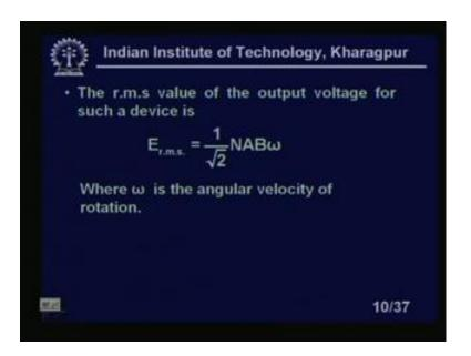
So, let us look at that the rms value of the output voltage for such a device will be given by E rms 1 by root 2 NAB into omega. What are the other things, what are the regions where omega is the angular velocity of rotation of the coil the figures I will show you. Let us go back to figure first because it is very reticules if I see this is our coil.
