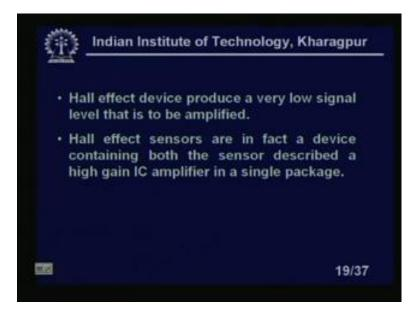
Hall effect device produce a very low signal level. So, that it is to be amplified. So, it needs an amplifications, because the voltage is very, very small please note it it is not a very large voltage. So, it could amplifier known as amplifier is necessary though the
