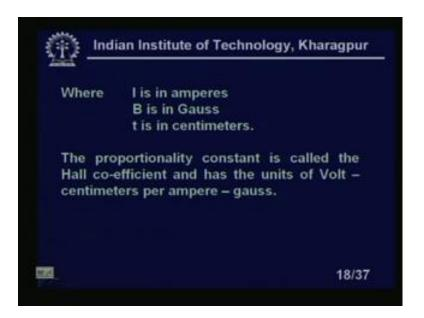
Where I is in amperes B is in gauss and t is in centimeters right the proportionality constant is called the hall coefficient. And has the units of volt centimeters per ampere gauss right. So, it is a hall coefficients and is the characteristics of the particular material bar has the unit of the volt centimeters per ampere gauss.
