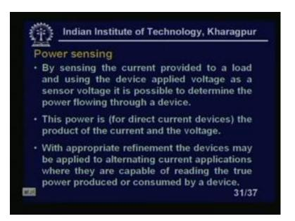
Power sensing: by sensing the current provided to a load and using the device applied voltage as a sensor voltage it is possible to determine the power flowing through the device right. This power is for direct current devices the product of the current and the voltage. With appropriate refinement and the devices may be applied to the alternating current applications where they are capable of reading, the true power produced or consumed by the device.
