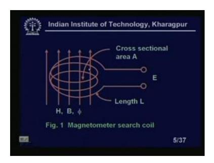
Actually we are assuming in the actual diagram you see if I go back to the diagram I have shown I have shown it like that. That H is perpendicular to the plane of the flat coil is not it. You see the H is perpendicular to the plane of the flat coil, but that is not the fact that be not be the fact though it is also less desirable, that it should be perpendicular that is output will be higher.
