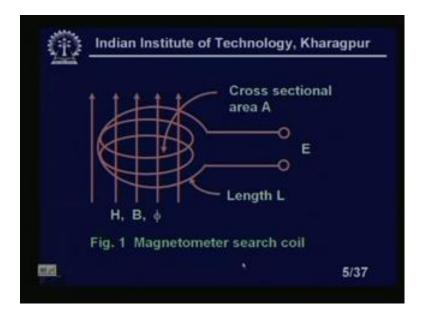
See this is the a coil which is and it is placed under magnetic field right and its cross sectional area is A length is L, and I am getting output voltage here E. Actually these output voltage is to be to get some output voltage, please go the 2 things is important either the magnetic field must vary or this coil was change its position. There should be
