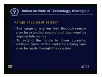
Range of the current sensor the range of a given feed through sensors may be extended upward and downward by appropriate wiring. So, by I mean you can wiring; that means, I can make it larger and smaller. To extend the range to lower currents multiple turns of the current carrying wire may be made through the opening that, because there is an opening through which current sensors will go.
