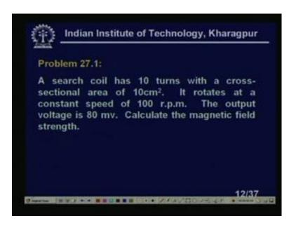
Now, let us solve some problem. So, that we will be more comfortable in the, so the problem is a search coil has 10 turns and with a cross sectional area of 10 centimeter square. It rotates at a constant speed of hundred revulsion per minute the output voltage
