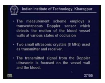
Now, measurement scheme employs a transcutaneous Doppler sensor which detects the motion of the blood vessel walls at various states of occlusion, right. Two small ultrasonic crystals 8 megahertz used as a transmitter as well as receiver. The transmitted signal from the Doppler ultrasonic is focused on the vessel wall and the blood.
