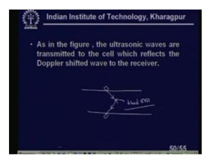
So, I have a source and I have a receiver here ultrasonic waves I am transmitting. So, it is getting here reflected back from the blood vessel. This is our blood vessels, blood cells rather I should say blood cell right. Reflects the Doppler shifted wave to the receiver. So, this getting reflected I am. This is getting reflected.
