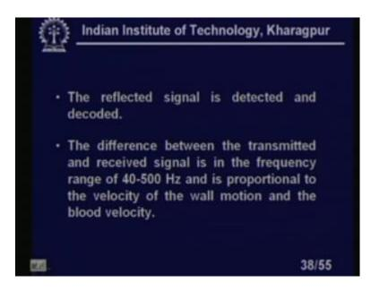
The reflected signal is detected and decoded, right. Decoding means; that means, I am decoding converting into the amplitudes and all those frequency depend I mean frequency voltage convert or that type of signal. Difference between the transmitted and
