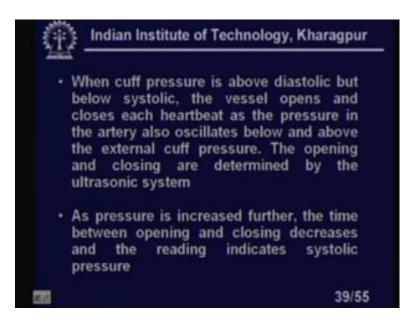
As pressure is increased further the time between the opening and closing decreases, and the reading indicates the systolic pressures, right.
