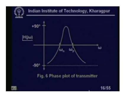
You see this is the phase plot of the transmitter. So, you can see within omega n omega p it is a 90 degree plus 90 degree phase shift, and outside that range it has a minus pi by 2 phase shift what does it mean?
