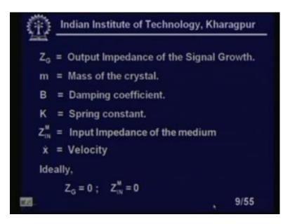
I am discussing all this where you see the ZG the output impedance of the signal. So, let me go back again ZG, ZG is here on the generator side, output impedance of the signal growth, mass of the crystals m, damping coefficient B, K the spring constant. ZMIN is the input impedance of the medium. X dot is a velocity and ideally we can assume always ZG equal to 0 and ZMIN. That means, output impedance of the signal growth is 0 and the input impedance of the medium is also 0.
