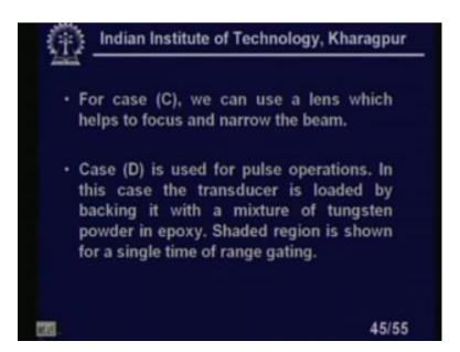
For case C, we can use a lens which helps to focus and narrow the beam. Sometimes we need to narrow the beam since it can be utilized to do there. Case D is used for pulse operations In this case the transducer is loaded by the backing it with a mixture of tungsten powder in epoxy and the shaded region is shown for a single time of range gating.
