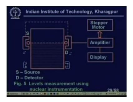
This is of the scheme of the level measurements. We have a source you see here. We have a detector here and. So, this is the level measurement using nuclear instrumentation. So, I have a liquid here. So, how it works?
