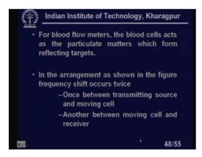
For blood flow meters the blood cells act as a particulate matters which form the reflecting targets right. Because as you know in the case of Doppler shift flow meters I mean in the case of transit time flow meters this is basically used in the case of clean
