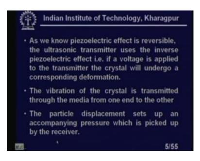
As we know piezoelectric effect is reversible. The ultrasonic transmitter uses the inverse piezoelectric effect as I just right now I told. That that is if a voltage is applied to the transmitter, the crystal will undergo a corresponding deformation, right. If I apply a voltage to a crystals, so there will be deformation of the crystal. So, how can I utilize? Let us look at you see I have I have a crystal here.
