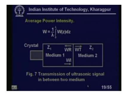
Average power intensity, is given by W equal to 1 by lambda integral omega z dz lambda over the integration of the limit lambda to 0. It looks like this you see the transmissions of ultrasound signal between 2 medium. You see the medium 1 and this is medium 2. This is crystals this is the reflected wave. We will see the regions what are the regions.
