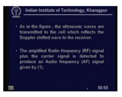
The amplified radio frequency signal plus the carrier signal is detected by the produce an audio frequency signal. It is the basic principles of a audio I mean our heterodyne receivers. This classical method actually utilized here also AF signals given by equation 1.
