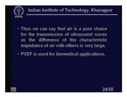
Thus we can say that the air is a poor choice for transmission of ultrasound waves, right. As a difference of the characteristic impedance of the air with others is very large, right PVDF is the polymer actually is used for biomedical applications.
