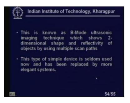
This is known as B mode ultrasonic imaging techniques which shows 2 dimensional shape and reflectivity of the objects by using multiple scan paths. This type of simple device is seldom used now; however, has been replaced and more elegant systems. So, with this I come to the end of lesson 25 which is on the ultrasonic sensors. Welcome to
