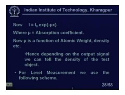
So, we have same or if the densities I mean the density might be different, but the atomic weight it can be the same. For level measurement we use the following scheme.
