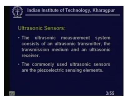
Ultrasonic sensors, if I look at the ultrasonic measurement system consist of an ultrasonic transmitter. The transmission medium and ultrasonic receiver whenever there
