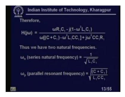
Therefore, I can say that H j omega if I write in the j omega domain. So, omega R 1 C 1 minus j all inside 1 minus omega square L 1 C 1, upon omega C plus C 1 minus omega square L 1 C C 1 plus j omega square C C 1 R 1. Thus we have 2 natural frequencies. series natural frequency which is 1 upon root over L 1 C 1. And the parallel resonant frequency omega p root over C plus C 1 upon L 1 C C 1 all another square root obviously.
