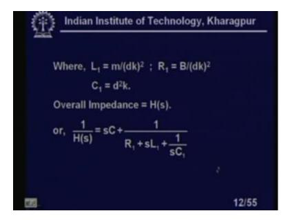
Where; obviously, when I reflect I mean the primary side, what is the relation between the I mean what we tried previously in the secondary side and what it has now in the primary side? That was been related by the, I mean I mean some coefficients which is decay. L 1 equal to m upon dk square R 1 equal to B upon dk square and C 1 equal to d square into k, right. Now, overall impedance I should say 1 by Hs or 1 by Hs SC plus 1 upon R 1 SL 1 plus 1 by SC 1.
