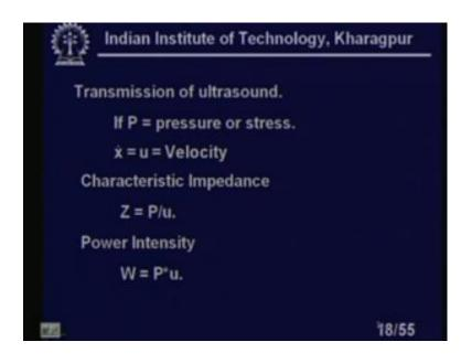
Transmissions of ultrasound; how will you transmit this ultrasound signal if P is the pressure or stress and X dot equal to u is the velocity, because X is the displacement. So, we have taking the derivative of that. So, the characteristic impedance Z equal to P by u. the power intensity W equal to P into u.
