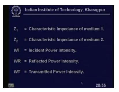
Where Z 1 is the characteristic impedance of the medium 1.What is Z 1? This is Z 1. Z 2 is the characteristic impedance of medium 2, right. And WI is the incident power intensity and WR the reflected power intensity and WT is the transmitted power intensity.
