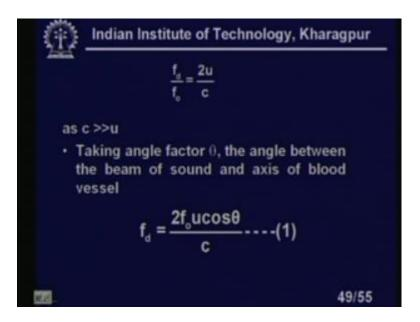
So, of the fd by f naught equal to two u by c as c is much much greater than u. Velocity of the ultrasonic must be much much greater than the velocity of the blood flowing in the artery. So, what I can say that taking angle factor theta the angle between the beam of sound and the axis of blood vessel fd equal to twice f naught u cos theta by c equation number 1.
