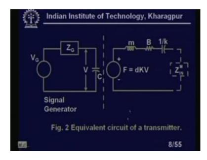
This is the equivalent circuit of a transmitter. I see we have a signal generators, on the other side we have m B 1 by K what are these regions will be shown in the next slide this is the equivalent circuit of a I mean piezoelectric transmitter, right which is actually we ultrasonic transmitter, I should say. So, its contrast in context with the, I mean piezoelectric crystals.
