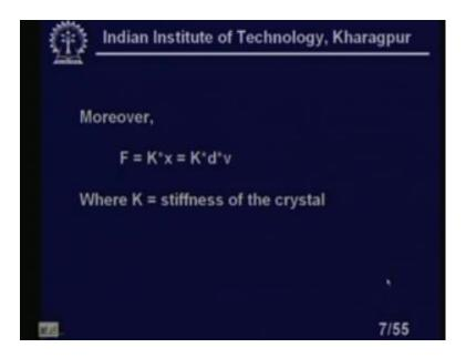
Moreover F we can write K multiplied by x K into x into d into v, where K is the stiffness constant of the crystal.
