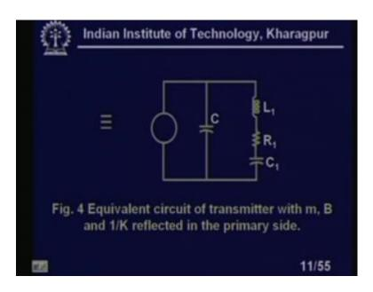
Now, this is the equivalent circuit, this is equivalent circuit of the transmitter with m B and 1 by K reflected in the primary side. If I reflect in the primary side; obviously, I will get L 1 R 1 C 1.
