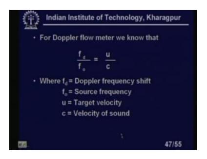
For Doppler flow meter we know that fd by fo equal to u by c where fd is the Doppler frequency shift. And fo is the source frequency which is basically ultrasonic frequency u is the target velocity and c is the velocity of sound sorry. It is source frequency not velocity. This f naught is the source frequency or the frequency of the ultrasonic sensor.
