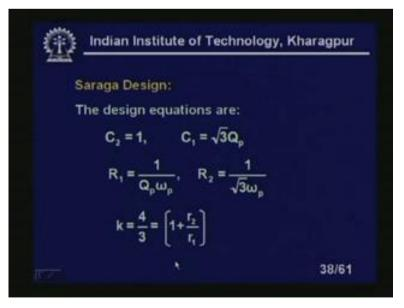
Saraga design, you see here the design equations are C 2 equal to 1, C 1 equal to root 3 Q p and R 1 equal to 1 upon Q p omega p, R 2 equal to 1 upon root 3 omega p. So, small k equal to always 4 by 3 upon 1 plus r 2 by r 1, right? So, it is fixed.
