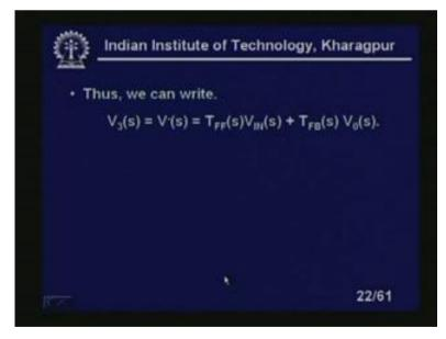
Now, we can write here also as before V 3 S equal to V minus S which is zero, obviously, T FF S, no it is not zero, because it is a negative feedback topology.
