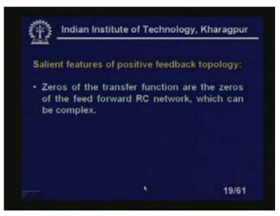
So, salient features of this positive feedback topology you see the, what is the salient features? Zeros of the transfer functions are the zeros of the feed forward RC network, which can be complex, right? Quiet obvious, you see what I am talking about.
