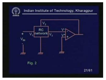
Now, this is a negative feedback topology. You see, this is a stable circuit. I do not need any positive feedback, whereas in the positive feedback, I mean a circuit we have seen that if it is positive feedback I have to give certain amount of negative feedback, right?
