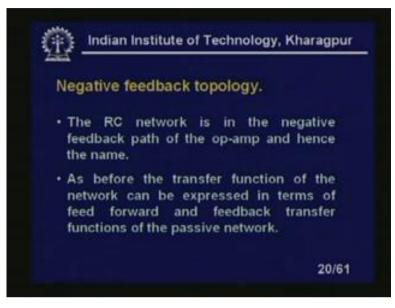
Now, negative feedback topology, if you look at the negative feedback, this RC network is in the negative feedback path of the op-amp and hence the name negative feedback topology, clear? As before, the transfer functions of the network can be expressed in terms of the feed forward and feedback transfer function of the passive network, right?
