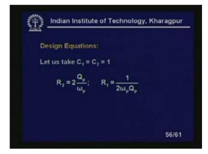
Now, design equations here in the case of a negative feedback topology, simple negative feedback topology or negative feedback without positive feedback circuits, looks like this. Let us take C 1 equal to C 2 equal to 1 and R 2 equal to 2 Q p by omega p and R 1 equal to 1 upon 2, 1 upon 2 omega p Q p.
