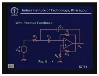
This is band pass circuits we have discussed, is not it? So, this is an enhanced negative feedback band, band pass circuit. That means negative feedback circuits with positive feedback. So, in band pass circuits, always it is desirable that the selectivity should be higher and higher. That is a good. Why? Quiet obvious, if I see there, here so that means what will happen? If I say, why I am telling?
