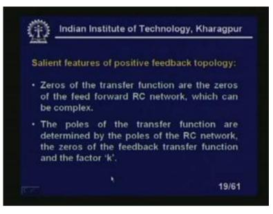
Whereas, the poles of the transfer functions are determined by the poles of the RC network, the zeros of the feed forward, feedback transfer function and the factor k. What is this, let us look at.
