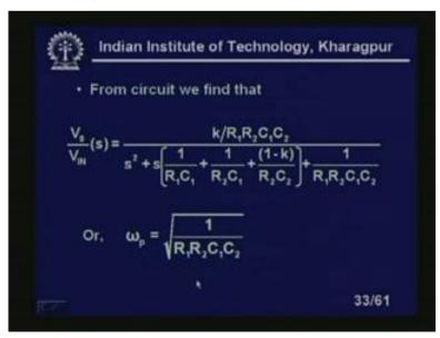
The transfer function, from the circuit so I can write V naught S by V IN S equal to small k upon R 1 R 2 C 1 C 2 upon s square plus s 1 upon R 1 C 1 plus 1 upon R 2 C 2 plus 1 upon 1 minus k upon R 2 C 2 plus 1 upon R 1 R 2 C 1 C 2, where this frequency or pole frequency will be given by omega p equal to root over 1 upon R 1 R 2 C 1 C 2.
