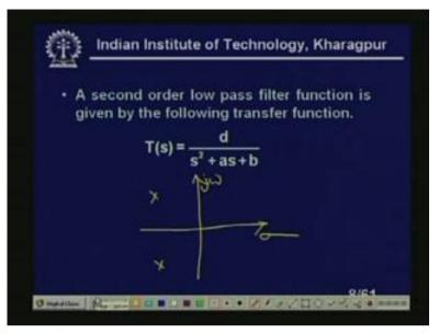
A second order low pass filter function is given by the following transfer function - d equal to s square plus as plus b, right? Now, even though in this case that the, our pole zero pattern will look like this, suppose sigma j omega plane, this is sigma, this is j omega, we have a complex conjugate poles and no zeros, right? So, this is called the pole zero pattern of low pass filter, clear?
