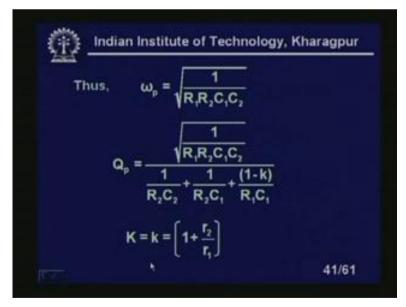
So, omega p equal to root over 1 upon R 1 R 2 C 1 C 2, Q p equal to root over 1 upon R 1 R 2 C 1 C 2 upon 1 upon R 2 C 2 plus 1 upon R 2 C 1 plus 1 minus k R 1 C 1. So,
