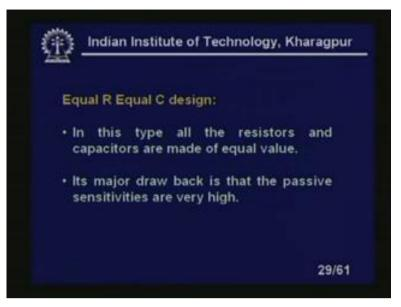
Equal R equal C design: in this type of, in this type all the resistors and capacitors are made of equal value. Major drawback is that the passive sensitivities are very high.
