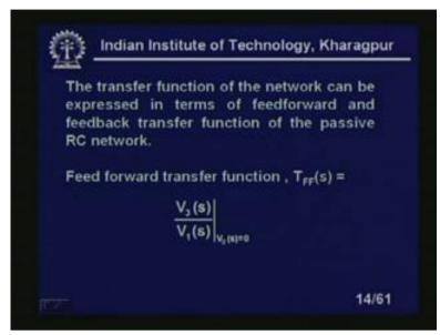
The transfer function of the network can be expressed in terms of the feed forward and feedback transfer functions of the positive passive RC network. Feed forward transfer function V, T FF S equal to V 3 S upon V 1 S making V 2 S equal to zero, right?
