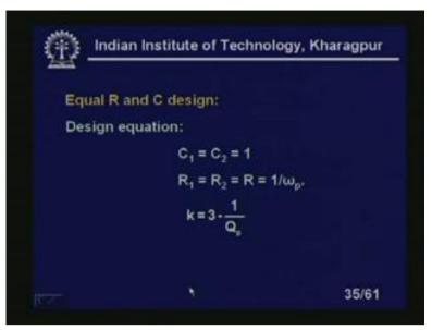
Now, equal R equal C design is, basically is actually you will find that in this equal R equal C design for the Sallen and Key low pass filter C 1 C 2 equal to 1 or R 1 R 2 equal to R equal to 1 upon omega p. So, obviously k, small k equal to 3 upon 1 by Q p.
