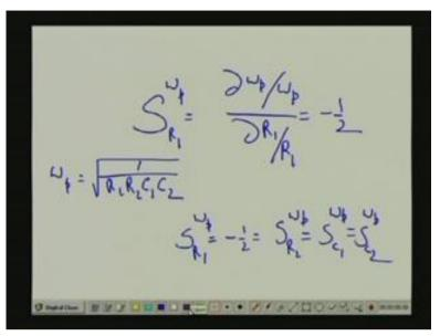
If I write that means S omega p R 1 will be delta omega p by omega p delta R 1 by R 1. In this case it is minus half, right and interestingly you see that in this case that since omega p is equal to root over 1 upon R 1 R 2 C 1 C 2, so S omega p R 1 is equal to minus half, I can write S omega p R 2 S omega p C 1 S omega p C 2.
