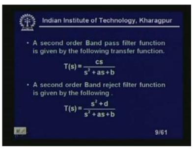
A second order band reject filter function will be given by the following equation - s square plus d upon s square plus as plus b, right? In this case that d must be equal to, that means it, the pole zero pattern will look like in the case if d is equal to b, then we call it band reject function.
