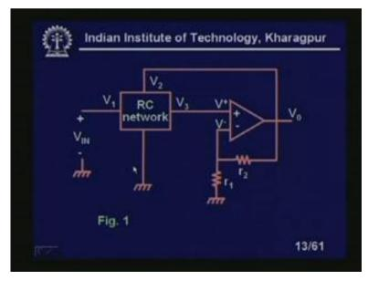
Because if you look at the circuit, you see that this is a positive feedback topology. RC networks in the positive feedback path, but if I keep the circuit as it is, circuit will not be stable. We need to make the circuit stable; we have to give some negative feedback. So, this negative feedbacks are given by these two resistances r 1 and r 2, clear?
