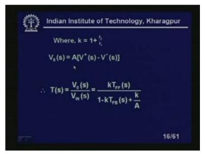
Now, where k equal to 1 plus r 2 by r 1 and V naught S equal to A. Obviously, output voltage will be equal to the amplifier gain multiplied by the difference of the signals which is coming in the inverting, non-inverting and inverting signal input, so which can be written as k T FF S 1 minus k T FB S plus k by A, right, small k by A.
