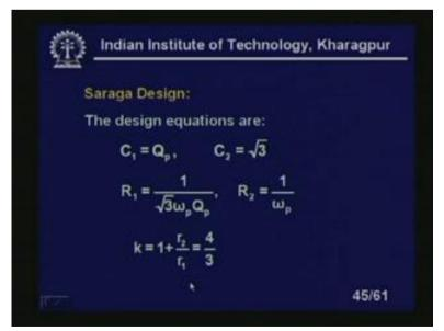
Saraga design for the high, I mean this structures are high pass structures. C 1 equal to Q p, C 2 equal to root 3. So, it is R 1 equal to 1 upon root 3 omega p Q p and R 2 equal to 1 upon omega p. Small k equal to 1 plus r 2 by r 1 equal to 4 by 3.
