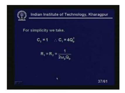
For simplicity we take C 2 equal to 1, C 1 equal to 4 Q p square. R 1 R 2 equal to 1 upon 2 omega p by Q p.
