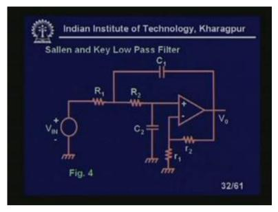
So, this is the Sallen and Key, famous Sallen and Key low pass filters using single amplifier structure, where we need 4 resistors. These two resistors values are different. This is small r 1 and r 2. This will determine the negative feedback which you are giving the positive feedback circuit. This is your RC network, so it is positive feedback topology, because RC network is in the positive feedback path.
