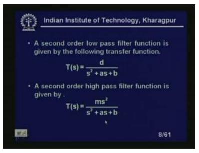
You see, this is high pass function. Now, K is absorbed in m, because we have a gain, constant K. Here also d is, K is absorbed in d.
