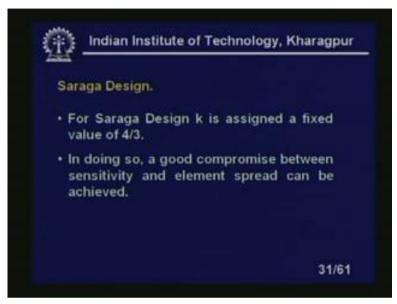
Saraga design: so, we have k is always, small k is always designated. It is assigned value of 4 by 3. In doing so, a good compromise between the sensitivity and the element spread can be achieved, right? So, we can have a good compromise between the two.
