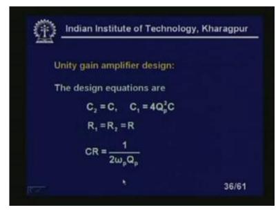
Now, unity gain amplifier design is that design equations are C 2 equal to C and C 1 equal to 4 Q p square C. Now you see, the Q p is slightly if it is 1 the capacitor spread
