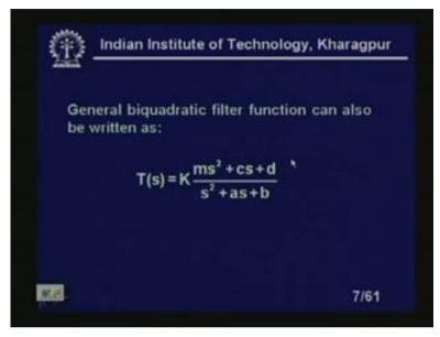
So, you can see that in this case if I make m and c zero, then I can get the, because if we look at the generalized functions that it see, you see, if I make m and c zero I will get, coefficients m and c zero, I will get a low pass function. If I make c and d zero, then I will get a high pass function, is not it?
