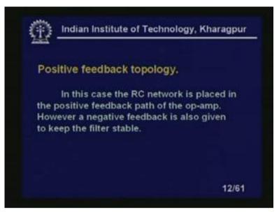
Now, positive feedback topology, you see what will happen? In that case of positive feedback topology we will have, in this case this RC network is placed in the positive feedback path of the op-amp and however a negative feedback is also given to keep the filter stable, right?
