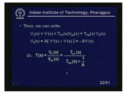
So, V 3 S equal to V minus S equal to T FF S into V IN S plus T FB S into, into V zero S. So, V zero S equal to A V, I mean this is the output voltage, obviously equal to the gain of the op-amp multiplied by the difference between inputs which is coming, right? V plus S and since V plus S is zero, in the case since it is connected to
