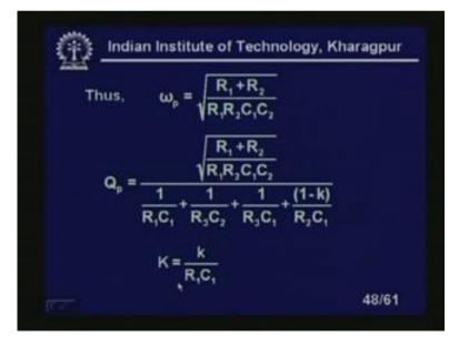
So, as before we can find this pole frequency, pole selectivity and the gain from the expressions which looks like omega p equal to R 1 under the square root R 1 plus R 2 upon R 1 R 2 C 1 C 2 Q p equal to under the square root R 1 R 2 R 1 plus R 2 upon R
