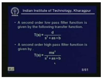
A second order high pass filter function is given by this - T s equal to ms square s upon s square plus as plus b.
