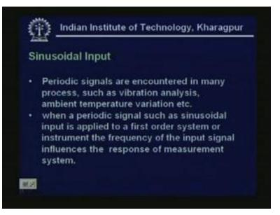
You see, the periodic signals are encountered in many process such as vibration analysis, ambient temperature variation, then, etc. When a periodic signal such as sinusoidal input is applied to a first order system or instrument, the frequency of the input signal influence the response of the measurement system. So, the frequency will control a lot of parameters; we will find that. So, frequency is of prime importance in the case of sinusoidal system.
