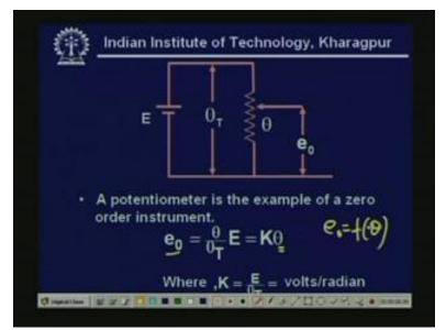
If I go back, I can see here, you see here that output voltage is directly proportional to theta. So, e is a function of theta, so which can be utilized to make a position sensor and it is a zero order instrument. So, obviously there is no phase lag or no time lag, phase change or time lag in the input output, okay.
