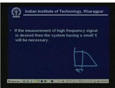
Now, if the measurement of high frequency signal is desired, then the system having a small tau will be necessary. Quite obviously, because our response we have seen again that the response falls down. So, if I want to take the response at the higher frequency, I must use a small value of tau, so that the omega tau will be, I can accommodate omega tau, will not be large, so that I can accommodate my frequency in this region, right?
