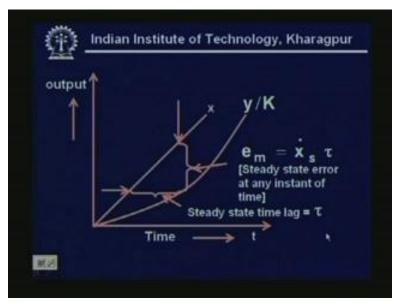
And interestingly, you see this steady state time lag is always tau. So, it means that steady state error will be at any instant of time, any instant of time X s dot into tau and so it is, time lag is tau.
