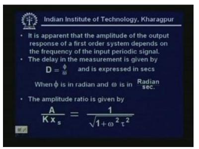
The amplitude ratio is given by A by Kx s equal to 1 upon under the square root 1 plus omega square tau square, we can see here.
