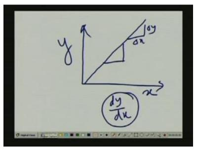
It means that if I look at it will be, suppose I have this characteristics calibration curve, this is x, this is y and I have a linear relation like this one. So, slope of this calibration curve, okay that is my dy by dx will give you the static sensitivity. So, this will give you the static sensitivity and since it is linear, you see anywhere the value of dy by, del y by del x, so if it is del x, it is del y, it is same.
