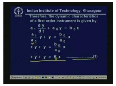
So, a naught, so you can see here, so that is we have multiplied entire equations by a 0. I got the equation a 1 by a 0 y dot plus y equal to b naught by a naught into x. So, dot we just replaced by dy by dt. So, tau, now I replace a 1 by a 0 equal to tau. Tau y dot plus y equal to b naught by a naught, upon a naught x. Finally, we have written tau y dot plus y equal to K x, right. K we remember.
