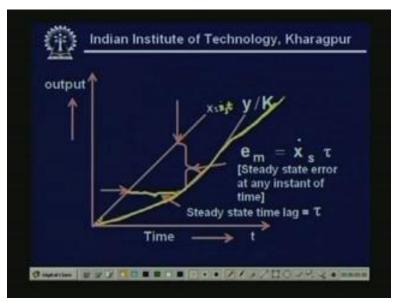
You see, if I plot it, it will look like this that steady state error at any instant of time, okay, hopefully it is finalized, it looks like this. So, x-axis we have plotted time and this is our output. These I have plotted. This is my input, so this is equal to actually X s dot into t, right and this is y by K. I have plotted the output. Actually this should be parallel, I mean it is, I cannot draw it nicely. I think it should be like this then. It should be parallel to the input.
