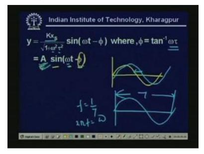
This we can write as equal to A sin omega t minus phi; phi is the phase shift of the input signal. There will be, there will be some phase shift that means that my, if my input is
