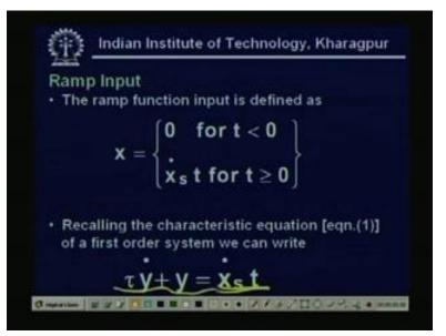
Recalling the characteristics equation, equation 1 of the first order systems, we call that first order systems here, we just replace X by X s dot t. X s dot means dX s by dt into t. So, tau y dot plus y equal to X s dot into t. This is our first order differential equation for ramp input. We will solve this equation and see how the output will come, how the response will come and how my, how my error in the measurement system will come?
