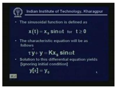
So, the solution to this differential equation yields, ignoring initial condition that y zero equal to y zero, get Kx s upon under square root 1 plus omega square into tau square sin omega t minus phi, where phi equal to tan inverse omega tau.
