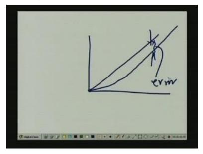
But, whereas in the case of ramp input, you see here, if I take a white page, in the case of ramp input, so there is always a steady state error, initially small. So, it is like that, so there is always a steady state error. This is our error. So, it will remain forever in the case of ramp input, since it is a time varying input function, right.
