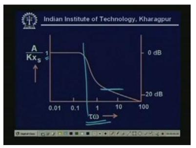
If I go back and see, our response we look at, for the frequency when I am getting the response here 1, so that is this desirable property. I cannot make the measurement at this region. I want to make the measurement in this region only, right, isn't it? So, this will be my frequency response of the operation, so that the omega tau has a lot of influence.
