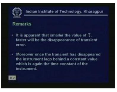
What is the remarks of a, I mean for a system with a step input? It is apparent that the smaller the value of tau, the faster will be the disappearance of the transient error. This is
