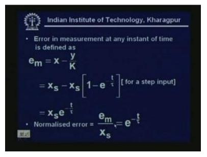
Error in measurement at any instant of time is defined as e m. We have used the subscript m that is to tell that it is an error in the measurement x minus y by K. So, it will be ultimately X s minus X s multiplied by 1 minus e to the power minus t by tau and it is for
