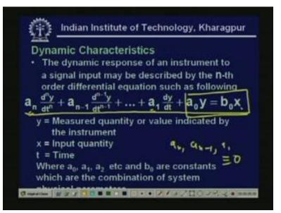
So, this differential equation, nth order differential equation if you put all zero that means from a n up to a 1 that means a n, a n minus 1 up to a 1, if you put all equal to zero, I will get the zero order instrument which looks like this. That actually I have shown just now. So, only this part if you take, it is a zero order instrument, right. So, this is our zero order instrument.
