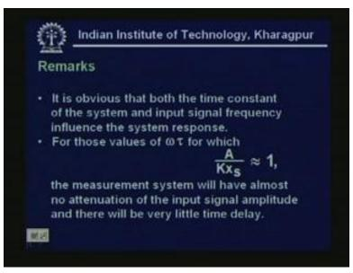
For those values of omega tau for which A equal to A by Kx s is almost equal to 1, the measurement system will have almost no attenuations of the input signal amplitude and there will be very little time delay. That is always we want that we have shown the response. Isn't it?
