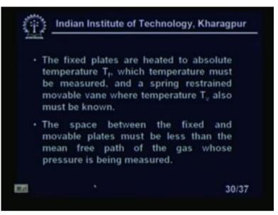
The fixed plates are heated to absolute temperature T f which temperature must be measured and a spring restrained movable vane where temperature T v also must be known. The space between the fixed and the movable plates must be less than the mean free path of the gas whose pressure is being measured.
