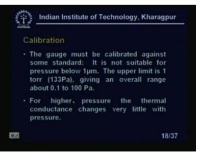
The calibration you see, the gauge must, must be calibrated against some standard. It is not suitable for pressure below 1 micron. The upper limit is 1 torr, 133 Pascal giving an overall range from 0.1 to 100 Pascal. For higher pressures, the thermal conductance changes very little with the pressure; thermal conductance changes very little with the pressure.
