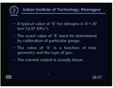
A typical value of the S for nitrogen is S equal to 20 torr to the power minus, which is 2.67 kilo Pascal to the power minus 1, right? The exact value of S must be determined by calibration of the particular gauge, right? So, for each gauge it is not gas independent, I mean like McLeod gauge and all those things. So, you have to measure
