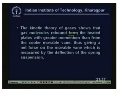
Now, kinetic theory of the gases shows that the gas molecules rebound from the, it is not from, I am sorry, this is from, from the heated plates with greater momentum than
