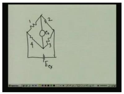
This is gauge 1, this is gauge 2, this is gauge 3, this is gauge 4. We have output voltage here, right, E ex, right? Now, the tangential stress are given by, we take a new page.
