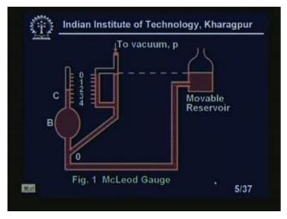
This is our reference capillary. So, until and unless this reservoir is, this mercury column in this reference capillary coming to this zero level. I will move the reservoir up and up, right? Once it comes to this zero level, I will stop moving the reservoir in the upward direction, right? The reservoir is subsequently raised until the mercury fills the bulb and rises in the cap, in the capillary to a point where the level in the reference capillary is located at the zero point, right?
