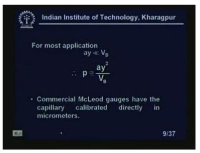
Commercial McLeod gauges have the capillary calibrated directly in the micrometers, right?
