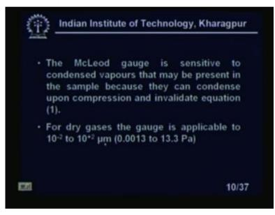
Now, McLeod gauge is sensitive to the condensed vapours that may be present in a sample, because they can condense upon the compression and invalidate equation 1. So this, we should be careful about that. For dry gases the gauge is applicable to the
