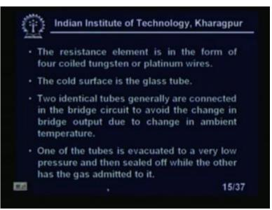
Now, the resistance element is in the form of four coiled tungsten or platinum wires as I have shown, right? The cold surface is the glass tube. The outer surface of the glass is a cold surface. Two identical tubes generally are connected in the bridge circuit to avoid the change in bridge output due to change in ambient temperature. One of the tubes is evacuated to a very low pressure and then sealed off while the other has a gas admitted to it.
