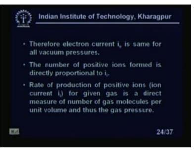
Therefore, electron current i e is same for all vacuum pressures. This is a great advantage. We will see the expressions. The number of positive ions formed is directly proportional to i i, ion current i i, I am giving the name. Rate of production of the positive ions, ion current i i for a given gas is a direct measure of the number of gas molecules per unit volume and thus the gas pressure, right?
