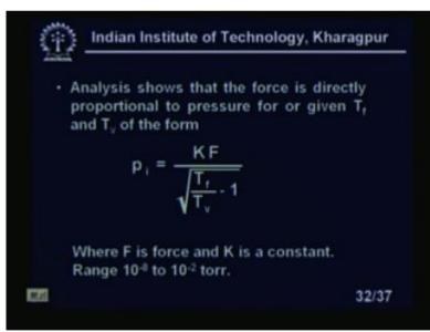
The analysis shows that the force is directly proportional to the pressure for a given T f and T v of the form, p i equal to K F upon under the square root T f upon T v minus 1, right, where F is a force and K is a constant. The range of the Knudsen gauge is 10
