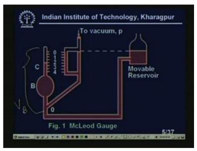
You see, the volume of the capillary that means I am telling the volume of the capillary up to this level, so this total volume I am telling is V B, subscript B, clear?
