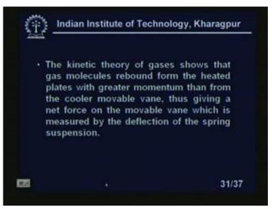
Now, kinetic theory of gas molecules rebound from the heated plates with greater momentum than from the cooler vane, movable vane thus giving a net force on the movable vane which is measured by the deflection of the spring suspension.
