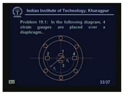
This r t is just the radius, where the, our circle on which this is the tangential strain gauges are placed, where r r is the radius of the circle on which, on which these two strain gauges which will sense the radial strain, this will sense the tangential strain, this will sense the radial strain, are installed, right, right? Let us go back again; already discussed.
