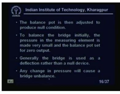
The balance pot is then adjusted to produce null condition, right? We have used that null condition; I have explained that thing. To balance the bridge initially, the pressure in the measuring element is made very small and the balance pot set for zero output. Generally the bridge is used as a deflection rather than a null device. Any change in pressure will cause a bridge unbalance. So, this unbalance we will calibrate in terms of ...
