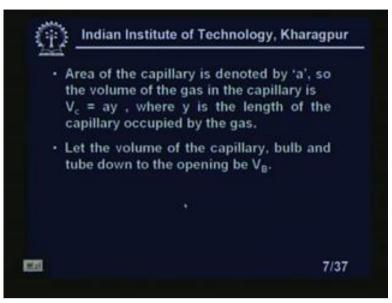
y is the length of the capillary occupied by the gas, right? That is true. Let the volume of the capillary, bulb and the tube down to the opening be V B. So, you see that V B is not only the volume of the capillary, it is volume of the capillary, bulb up to the point zero. I should, I refer back again.
