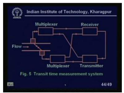
So, this is our transit time measurements. You have multiplexer. It will activate whether this will be transmitter or receiver and this is the receiver signals and we will have a circuit.
