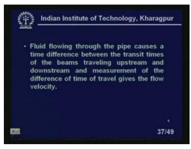
The fluid flowing through the pipe causes a time difference between the transit times of the beams traveling upstream and the downstream and measurement of the difference of time traveled gives the flow velocity. What is that? (Refer Slide Time: 36:16)
