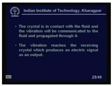
The crystal is in contact with the fluid and the vibration will be communicated to the fluid and propagated through it to, what far? To the point, where the other sensors are there, diametrically opposite side. The vibration reaches the receiving crystals which produces an electric signal as an output, right?
