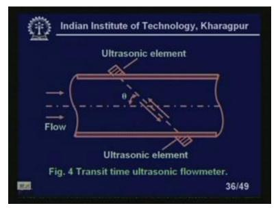
So, when the liquid is coming, when the, I mean this ultrasonic wave is traveling in this direction, this upstream direction, because it is moving and when it is flowing the, when the ultrasonic waves it is coming back which is in the opposite side of the beams, so there is a time shift between the two, right? Received signal transmitting between the time lapse between the signal transmitted and the received it will be different in two cases, right?
