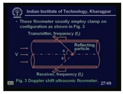
What is that to we can look at that if I look at ultrasonic flowmeter, it will, this is here. You see here, this is the wedge inside which we have put. So, the velocity of the fluid in
