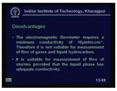
The electromagnetic flowmeter requires a minimum conductivity of 10 micromho per centimeter, right? Therefore, it is not suitable for measurements of flow of gases and liquids, of liquid hydrocarbons. So, it is not suitable for measurements of liquid, any oil
