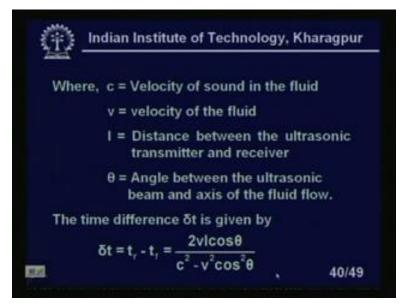
c is the velocity of sound in the fluid, v the velocity of the fluid, l is the distance between the ultrasonic transmitter and receiver, theta is the angle between the ultrasonic beam and the axis of the fluid flow, right? The time difference delta t is given by delta t equal to t r minus t f. If you subtract 2 vl cos theta upon c square minus v square into cos square theta, clear?
