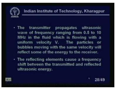
The transmitter propagates ultrasonic, ultrasonic wave of frequency ranging from 0.5 to 10 mega Hertz in the fluid, which is flowing with a uniform velocity of V. The particles or bubbles moving with the same velocity will reflect some of the energy to the receiver, right? Some of the energy will be, I mean received by the receivers which is again are piezoelectric crystals. The reflecting elements cause a frequency shift between the transmitted and reflected ultrasonic energy.
