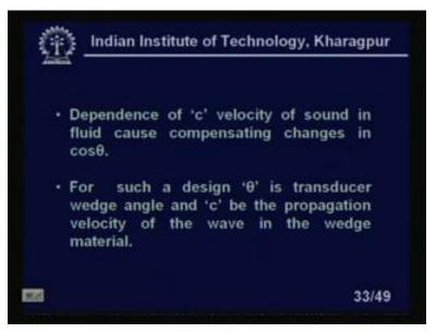
Dependene of c, velocity of sound in fluid cause compensating change in cos theta. For such a design, theta is transducer wedge angle and c be the propagation velocity of the wave in the wedge material.
