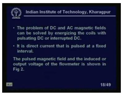
The problem of DC and AC magnetic fields can be solved by energizing the coils with pulsating DC or interrupted DC. We will use some interrupted DC, right, so that to solve this type of problem. Neither there will be any DC problem polarization effect, then electrochemical effect and then thermoelectric effect where those transformer feedback action which is common in the case of 50 Hertz AC energized magnetic field. So, this can, we can discuss in details.
