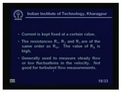
So, current is kept fixed at a certain value that can be measured by that resistance that by the ammeter. What is that ammeter? This ammeter, the, with the ammeter we can see whether the current is getting or remaining constant or not. The resistance R 1, R 2, R3, are of the same order as R w. Typically it should be quite small compared to the R, R s and the value of R s is high, right?
