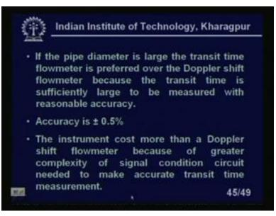
If the pipe diameter is large, then the transit time flowmeter is preferred over the Doppler shift flowmeter, because we are, at that time the transit time will be large and it will be
