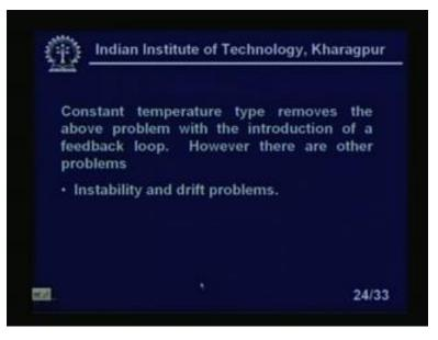
Constant temperature type removes the above problem with the introductions of the feedback loop. However, there are other problems. Instability and the drift problems of the there, because drifts of the amplifier will come in picture, right? With this, I come to the end of the lesson 16 of Industrial Instrumentation.
