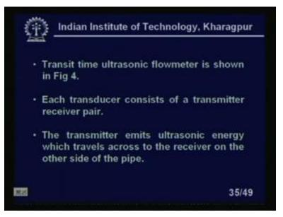
Transit time ultrasonic flowmeter is shown in Figure 4, next figure. Each transducer consists of a transmitter receiver pair. So, each transducer is a transmitter receiver pair and transmitter emits ultrasonic energy which travels across to the receiver on the other side of the pipe, right?
