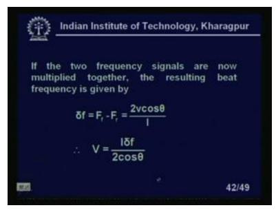
See, if I take this frequency shift, thus the frequency, I mean if the two frequency signals are now multiplied together, the resulting beat frequency is coming, difference and the sum frequency will  $\dots$  2 v cos theta by l if the difference frequency, so v is l delta f 2 cos theta. If l and 2 cos theta are same, fixed, so delta f we can see is directly proportional to the velocity of the fluid flow, right which is flowing through the pipe.
