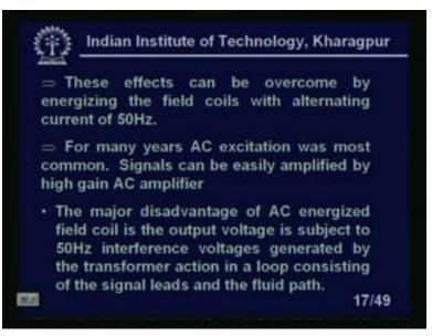
Solution - these effects can be overcome by energizing the field coils with alternating current of 50 Hertz. We can apply a 50 Hertz signals, alternating signals, right, so and it is used for over the years, right? For many years AC excitation was most common. That signals can be easily amplified by high gain AC. This is another advantage of the AC,
