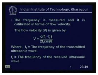
The frequency is measured and it is calibrated in terms of flow velocity. It is calibrated in terms of flow velocity and the flow velocity V is given by c f t minus f r 2 f t cos theta. What are those legends? f t is the frequency of the transmitted ultrasonic wave, f r is the frequency of the received ultrasonic wave or reflected ultrasonic wave.
