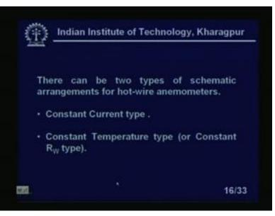
So, there can be two types of schematic arrangements of hot wire anemometers. That is I am telling either it will be constant current or constant temperature, right? So, constant current type and constant temperature type or constant R w type.
