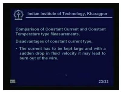
Now, comparison of the constant current and constant temperature type measurements, disadvantage of the constant current types, the current has to be kept large and with a sudden drop in fluid velocity it may lead to the burn out of the wire. So, this is a typical problem of the constant current type. That means the current has to be kept large, otherwise what will happen? So, usually it is large and if there is sudden fall in the fluid
