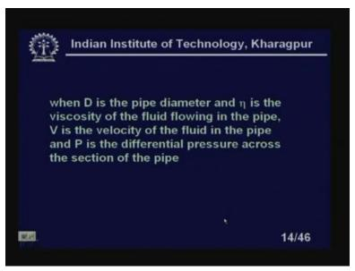
This will give you the Reynold number, where D is the pipe diameter, eta is the viscosity of the fluid flowing in the pipe, V is the velocity of the fluid in the pipe and P is the differential pressure across the section of the pipe, right?
