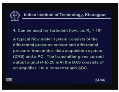
Number 4, it can be used for turbulent flows, because turbulent flow is characterized by when R e is much, is greater than 10 to the power 4, 10,000. A typical flowmeter system
