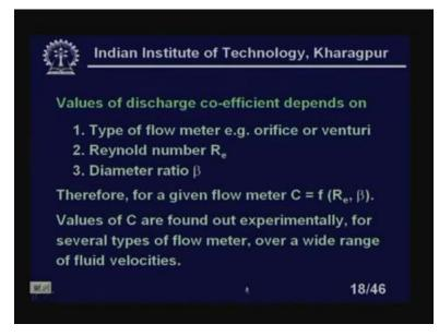
Values of the discharge coefficient depend on type of flowmeter that is orifice or Venturi, Reynold number R e, diameter ratio beta. So, therefore for a given flow rate, flowmeter, I can write C equal to, is a function, C is a function of R e, Reynold number and beta. Values of C are found experimentally for several types of flowmeters over a wide range of fluid velocities, right, because flowmeters velocity should be, C should be known to you.
