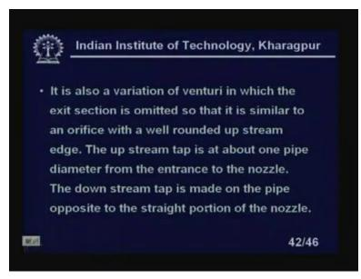
It is also a variation of the Venturi in which the exit section is omitted. We have, do not have any exit section if you look at very carefully, so that it is similar to the, similar to an
