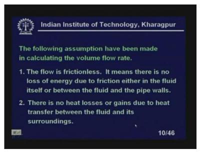
So, the following assumptions have been made in calculating the volume. So, you have to make some simple assumption to calculate the volume flow rate. These are: the flow is frictionless. It means there is no loss of energy due to friction either in the fluid itself or between the fluid and the pipe walls. There is no heat losses or gains due to heat transfer between the fluids and surroundings.
