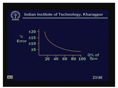
These error you can see here, excuse me, say error you see here, error here is quite low at the low flow velocity, quite low at the, at the high flow velocity and is very high when the flow velocity is, volumetric flow rate is slow.
