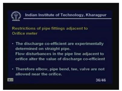
Now, restrictions of the pipe fittings adjacent to orifice meter - this is another most important thing practicing engineers must follow, so as that is the restrictions of pipe fittings adjacent to orifice meter. There cannot be pipe fittings, pipe bendings, tees, bags, etc., very near to the orifice, both upstream and downstream. What are those? Let us look at details. The discharge coefficients are experimentally determined on straight pipes, right?
