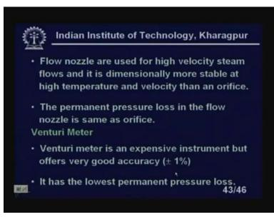
Flow nozzles are used for, because you know that in some situations or there is high pressures and high velocities, sometimes the orifice is not very stable. There is the question of buckling and all these things; that type of situation we have to use the flow nozzle and we cannot spend that money everywhere, I mean to install a Venturi meter instead of the orifice meter. So, in that type of situations you can use flow nozzle, because it is cheaper than the Venturi meter.
