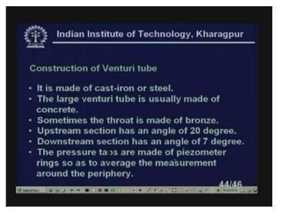
Upstream section has an angle of 20 degree and downstream section has an angle of 7 degree. These are all included angle, right? The pressure taps are, this should be, I am sorry this will be pressure taps, this will be pressure taps; pressure taps are made of piezometer rings, so as to average the measurement around the periphery.
