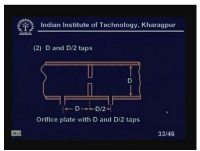
Now, we have an orifice plate with D and D by 2 taps. Here you can see that it is, upstream is D and downstream D by 2 tap. All these have some advantage and disadvantages.
