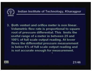
Now, both Venturi or orifice meter is non linear that is most important. If you see, volumetric flow rate is proportional to the square root of the pressure differential, right? So, this limits the useful range of a meter in between 25 and 100% full scale output reading. At lower flows, the differential pressure measurements is below 6% of full scale output reading and is not accurate enough for the measurement.
