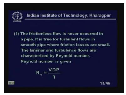
There is some restriction. Why I am calling it theoretical? We will find that we have to multiply by the discharge coefficients with the actual flow rate, actual volumetric flow rate. The frictionless flow is never occurred in a pipe. It is true for turbulent flows in smooth pipe where friction losses are small. The laminar and turbulence flows are characterized by the Reynold number and a Reynold number is given as R e equal to VDP by eta.
