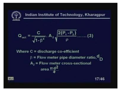
Therefore, the theoretical expression of volume flow rate is corrected as C. We are introducing a new factor C under the square root 1 minus beta to be the power 4 multiplied by A 2 under the square root 2 P 1 minus P 2 by row, where C is discharge coefficient and beta is the flowmeter pipe diameter ratio, small d by capital D and A 2 is the flowmeter cross sectional area. This is equal to pie d square by 4.
