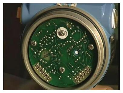
We can open this side and see here the circuitry and we can connect here and there is a .... things here and this side you can make all the connections sort of things for taking the, both the, giving a signal and taking the 4 to 20 milliampere of current. This circuitry which we, this, this actually the .... which you can take it out for making repairment and all that type of job.
