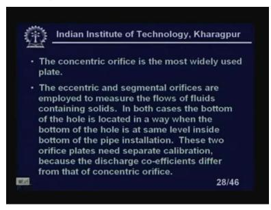
So, the concentric orifice is the most widely used plate. Eccentric and segmental orifices are employed to measure the flow of the fluids containing solids. In both cases, the
