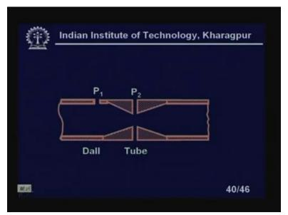
Now, this is a dall tube. So, we have a pressure, you have pressure tap here P 1 and pressure tap here P 2. So, these are all, basically there are some relative advantages and disadvantages in all these types of things. Flow nozzle and dall tube, let us first discuss the flow nozzle and dall tube, compare, then we will discuss the Venturi in details.
