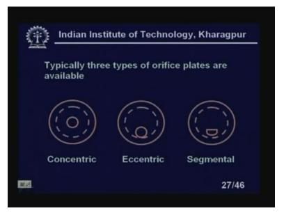
Let us go back again. So, these are the three different types of orifice, if you look at. So, there is a concentric orifice, eccentric orifice and segmental orifice. All has different application that is the reason we are plotted, we are given like this.
