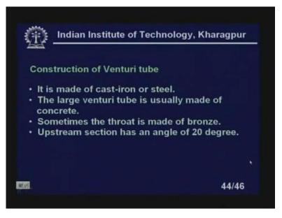
The large Venturi tube is usually made of concrete, because if it is very large, so it is very difficult to make, made of cast iron or steel. In that case we go for the concrete. Sometimes the throat is made of bronze, as I told you earlier, for easy replaceability. Upstream section has an angel of 20 degree, included angle. That means if you look at, so it looks like this.
