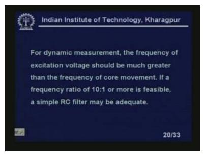
So, for dynamic measurement, the frequency of excitation voltage should be much greater than the frequency of core movement. If a frequency ratio of 10 is to 1 or more is feasible, a simple RC filter may be adequate.
