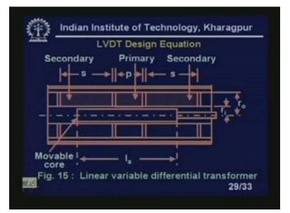
This is our, see schematic of our LVDT. Even though you see that these are the two primary windings, this is a primary winding, because you see this is basically a cylinder sought of thing, right? It is cylinder, I mean here we have the, this core, you see this iron core, so this is our primary. This is the coil, like this one; it is a primary and two secondary, identical secondaries. Now you see, this length of the secondary we have given S, this is length of the primary we have given P.
