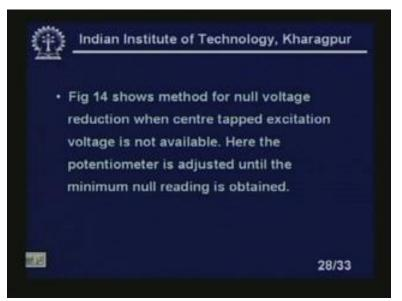
So, figure 14 shows actually method for null voltage reduction when centre tapped excitation voltage is not available. Here, the potentiometer is adjusted until the minimum null voltage reading is obtained. If it cannot be zero, we can make, we cannot make it zero, make it minimum, so that that will be that means at zero null position, that some minimum voltage is, we will get. That will suffice in most of the cases.
