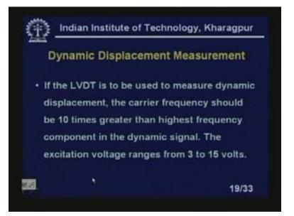
Now you see the dynamic displacement measurements. If the LVDT is to be used to measure dynamic displacement, the carrier frequency should be 10 times greater than the highest frequency component in the dynamic signal. We will show the phase sensitive demodulation output after few slides. The excitation voltage ranges from 3 to 15 volts, right, because in some situations, I may need to make the dynamic measurements even though frequency should not be that high.
