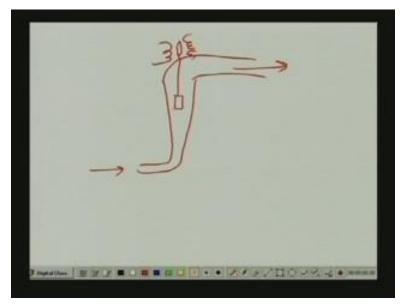
Other applications of LVDT if I look at, you said that we have seen that the rotameter in many places, so we have a core and a channel like this one. So, the float is here, so the flow is in this direction, it is coming out in this direction. So, what they do? With a ..... ceiling they connect a core here, same similar two secondaries in opposition. So, if I draw it nicely, it looks like this.
