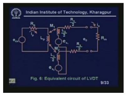
We have taken here, this inductance is L p. Primary inductance, this is primary resistance R p, this is excitation voltage ex and this is the resistance of the, there are two secondaries, we are taking the, if we assume that two exactly identical, so I can take this inductance is L s by 2, this resistance is R s by 2. So, we will get a simplified equation. This is the, M 1 is the mutual inductance between the primary and the one of the secondary.
