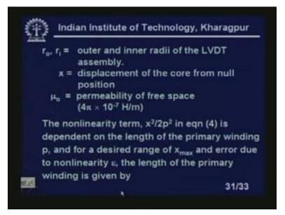
So, the non linearity term x square minus by 2 p square in the equation 4 is dependent on the length of primary winding P for a desired range of X max and the error due to nonlinearity, I mean epsilon, the length of the primary winding is given by this.
