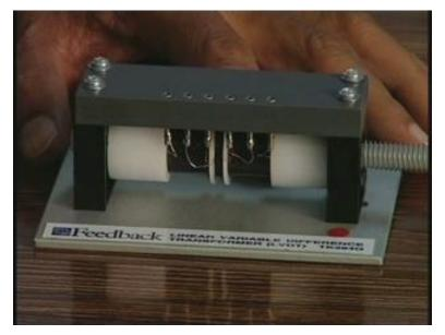
You see here, this is an LVDT - linear variable differential transformer. It has one primary and two secondary. The secondaries are usually connected in opposition to get a null position and through, after doing the phase sensitive demodulations, I can sense on which side of the, which side of the null position my, the core lies?
