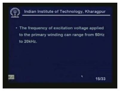
The frequency of excitation voltage applied to the primary winding can range from 50 hertz to 20 kilohertz.
