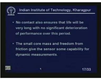
No contact also ensures that life will be very long with no significant deterioration of performance over this period. The small core mass and the freedom from the friction give the sensor, gives the sensor the some capability for dynamic measurements.
