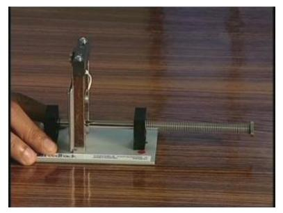
This is another application of the capacitance sensor which can be utilized to measure the displacement. Usually capacitance sensors are based on the three different criteria. One you can vary the area of the plates, you can vary the displacement between the plates that means separation of the plates and also you can vary the position of the dielectric medium inside the capacitor. The particular gauge which you are, you are looking at now basically depends on the displacement.
