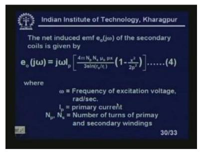
Now, net induced emf of the secondary coil is, will be given by this. You see here, so this is our net induced emf in the output: e j omega j omega I p 4 pi N p N s mu naught px upon 3 s natural log of r o by r i 1 minus x square by 2 p square - equation number 4, where omega is the frequency of excitation voltage in radians per second and I p is the primary current, N p, N s are the number of turns of primary and secondary windings.
