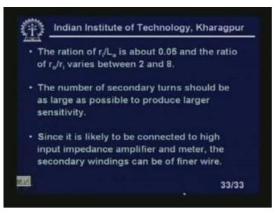
This is necessary and you see, if you look at, so this ratio, in fact this will be ratio, the ratio of r i by L a is about 0.05 and the ratio of r o by r i varies between 2 and 8. The number of secondary turns should be as large as possible to produce larger sensitivity and since it is likely to be connected to high input impedance amplifier, quite obviously and the meter, the secondary windings can be of finer wire, right?
