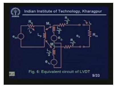
If I go back, you see, e s1 is this one and e s2 is this thing, right? So, this is the induced secondary voltage, right? So, this is our actual equation. So, you see the induced secondary voltage. This is applying on the primary sides. But in the secondary side this will induce a voltage like this one, e s1 equal to e s2; e s1 equal to M 1 di p by dt and e s2 equal to M 2 di p by dt. So, all, with respect to the, the primary current, right?
