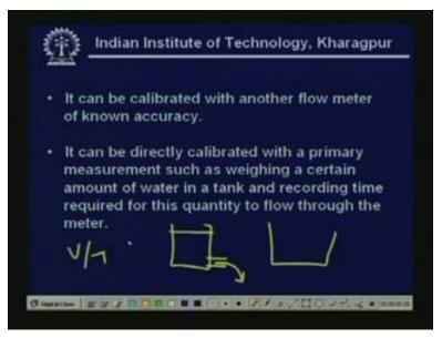
Number 2, it can be calibrated with another flow meter of known accuracy. It can be directly calibrated with a primary measurement such as a, such as weighing a certain amount of water in a tank or a recording time required for this quantity to flow through the meter. How does it look? It looks like this. It looks like, suppose I have a flow meter, I have a vessel. So, I know how much is the height, I know how much is the water
