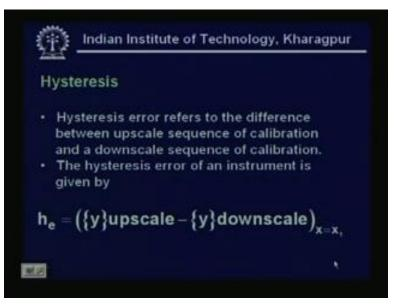
Hysteresis is another important ... Hysteresis error refers to the difference between the upscale sequence of calibration and downscale sequence of calibration and the hysteresis error of an instrument is given by y upscale minus y downscale at X equal to X 1. What does it mean? It looks like this.
