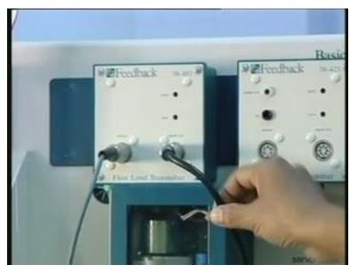
Now, for that you see here there is a, you have a float level transmitter which will transmit 4 to 20 milliampere of current to the process. This system, this, first it will go through this chord, it will go to the process interface.
