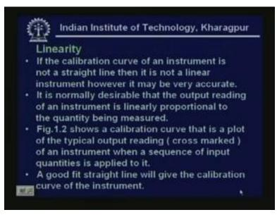
Now, it is normally desirable that the output reading of an instrument is linearly proportional to the quantity being measured. Figure 1.2 shows a calibration curve that is a plot of the typical output reading, cross marked, of an instrument when a sequence of input quantities is applied to it; we will show in the next slide. A good fit straight line will give the calibration curve of the instrument. How does it look?
