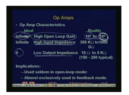
So, if you see actually you know ideally operational amplifiers have some characteristic, but real operational amplifiers actually have characteristic, which are very close to the ideal characteristic that is why operation amplifiers are so extensively used. So for example, the input impedance of the amplifier is ideally infinite. Ideally it has an extremely high rather the open loop gain is infinite, that is the value of G is very, very large.
