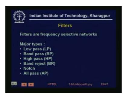
Now we come to the other important block, which is called filter. So, we have various kinds of filters for example, the filters are basically frequency selective network. So, as we all know that any arbitrary waveform can be always thought of as a sum of sinusoidal waveforms of various frequencies. The job of the filters is that they will allow some of the frequencies or they will amplify some of the frequencies and they will not allow some of these frequency.
