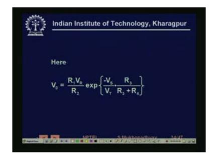
So, the output voltage in this case becomes exponential of Vs, so it is an anti-log operation.
