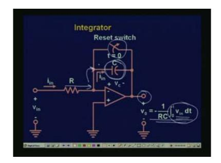
So, circuits are available with very high CMRR values. Now, we come to a circuit called the integrator. So, if we want to integrate what we do is, we put a capacitor here. So, now this current flowing will now still flow through this switch is open when it is working. So, therefore, the output will be 1 by RC into integral 0 to t Vin dt. So, the output voltage in the output voltage we have produced a voltage, which is proportional to the integral of Vin.
