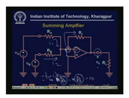
Then, in many cases instrumentation we need to add up signals. For example, you can take sensor suppose, you want to compute the average value. Actually have put two sensors, which are both measuring temperature and you want to measure the average temperature. So, then what you have to do is, you have to multiply each one of them by again say 1 by n and then add all of them. So, that is require a summing amplifier.
