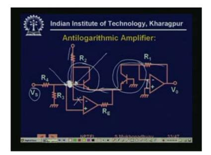
Using the same principle one can also construct an anti-log amplifier. Actually this circuit is as it is drawn is erroneous, this line will not be there, this line should be deleted. So, you see again we have a diode here and we have again because of this virtual ground, we have a diode here. So, in this case you can understand that voltage here at this point is actually proportional to Vs. It is actually R 3 by R 4 plus R 3 in to Vs.
