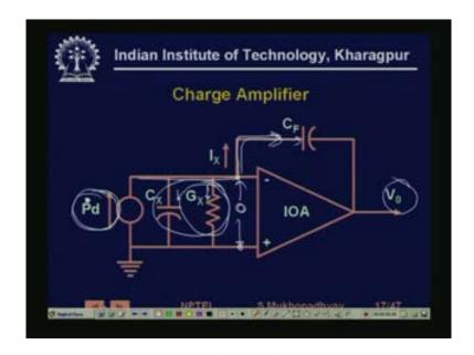
Next we have a charge amplifier. So, you see that there are sudden cases where, we need to produce a voltage which is proportional to the charge. For example, as we have seen in the piezoelectric crystal, that the piezoelectric crystal produces charge which is proportional to the force applied or the displacement of the piezoelectric crystal surfaces. So, in this case you can see that the input signal is actually assumed to be a pressure so we have put P dot.
