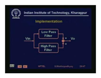
So, that is what is shown here, that low pass and high pass are shown in parallel.
