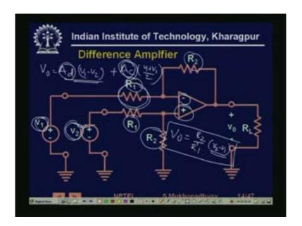
Similarly, we can have a difference amplifier. Now, see this configuration is slightly different in the sense that one of the sources are connected to the non-inverting input through a resistance network and the other is connected to the inverting input. So, it is a combination of inverting, non-inverting and also note that the resistance values are made equal. So, what happens, what is the result? Result is that you get that V output is equal to R 2 by R 1 into V 2 minus V 1.
