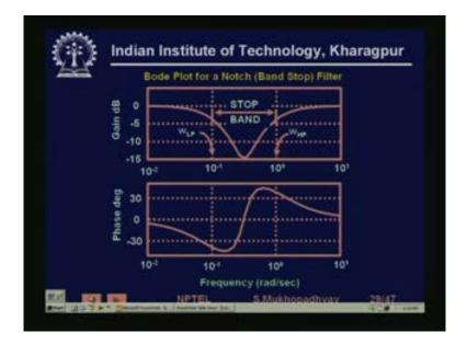
So, Bode plot is also shown. The Bode plot as you see you can see that falls down at some frequencies. So, reject this stop band.
