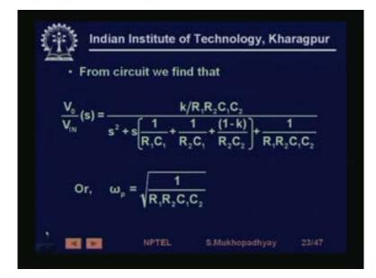
So, in the Sallen and Key filter the transfer function is given like this where, this K is actually the gain of the last hop block, which is 1 plus 1 plus R 2 by R 1 because it is an non-inverting block if you have noticed. So, obviously from the transfer function, we realize that it is a low pass transfer function, the top is constant and the bottom you have an second order polynomial in s.
