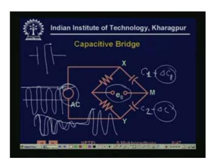
Similarly, it is not only that resistive sensor can be incorporate in to strain gauge bridges. Actually, this this theory that the output voltage is depending on the bridge ratio is true for general impedances. So, therefore we can we can instead of resistances, we can also have you know capacitive sensor where you have capacitance C 1 and you have capacitance C 2 and therefore, this is C 1 and this C 2.
