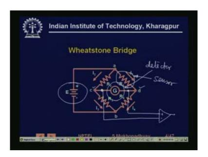
The Wheatstone bridge structure as we are seeing. In this case the bridge is drawn for 3-4 resistive elements, so this is the source. There are 4 resistances, this is the so called detector and in the case of an instrumentation setting generally, what is done is that, this bridge is operated in the unbalanced condition. As we can easily realize that, the voltage between this c and d points depend on the resistance ratios.
