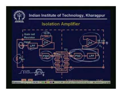
Next, we talk about an isolation amplifier. You know there are certain cases where the input sensors may be at some very high voltage. For example, suppose you want to measure a motor current. Now, we typically what we do is we take the winding of the motor and in series with the winding. Sometimes we just connect a resistance and we tap this voltage just to sense the current through the motor winding.
