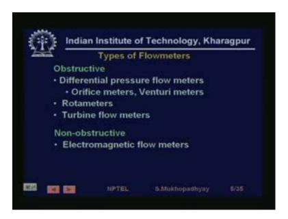
So, having said that, let us basically try to characterize flow meters. So, flow meters can be characterized in 2 ways. The first is obstructive or you know intrusive measurement. So, intrusive means that the instrument or the sensor will be put in the flow. So, it will affect the flow in even if in a small way, but it will affect the flow, it will obstruct it.
