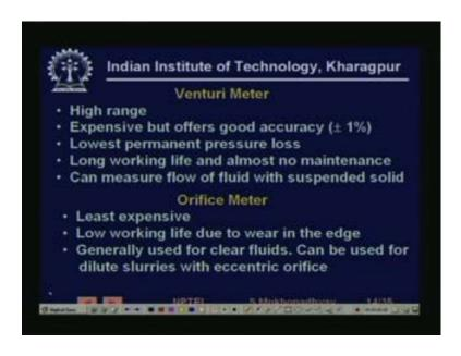
If you compare venturi meters with orifice meters turns out let us see, what is happening here. So, you have venturi meters can work with or work on very high ranges. You can have very big venturi. They are expensive compare to orifice meters because you need to make the whole pipe section they are nicely machine not just a plate, but they are definitely offer good accuracy and lowest permanent pressure loss.
