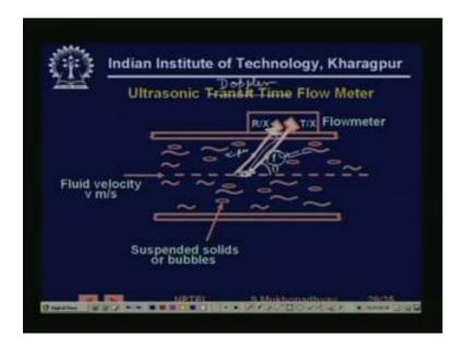
Similarly, we have we have an ultrasonic, this is not a transit time flow meter this is actually, this is wrong title that we have got, this is a Doppler flow meter here is a. So, what we are doing is, this is use for particulate. So, you see in the fluid we have some solid suspended particles right. So, you have an ultrasonic transmitter and you have an ultrasonic receiver. So, at this transmitter is transmitting an ultrasonic pulse which is sound pulse in this direction.
