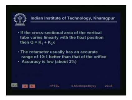
If you if you vary AT minus AB proportional to X, then you have a measurement Q is equal to K 1 plus K 2 X. The rotameter is usually accurate and you can see that, here the measurement is linear with X and you have better range ability than that of the orifice.
