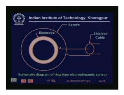
So, you can put electrodes on the pipe and from this electrode, for example, in this case it will collect charge. So, you collect charge from this point and you collect charge from this point and then you correlate these 2 charges. That way you can measure the velocity. So, we are going to skip this.
