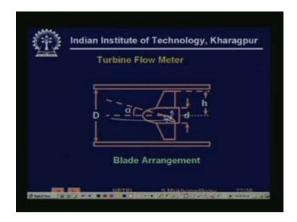
You will find that this is the blade. So, you see this is the blade and actually it is not properly drawn if the blade is like this. So, when the liquid passes it actually pushes the blade it pushes the blade. So, the turbine rotates right. It actually the blades are made slightly slant right. So, when they are made slant when the fluid will pass it will push the blade this. So, that is how it rotates.
