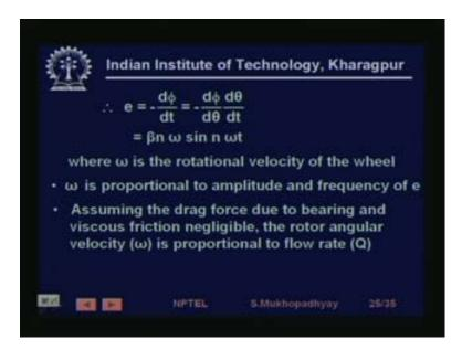
So, now we can it is a simple matter to calculate what is e, what is the induced EMF in the coil that is nothing, but we have we actually have a permanent magnet. So, permanent magnet means the magnetic strength is constant and we have we have put the coil across which an EMF is induced as flux pulsates. So, that is given by simple d phi d t and it turns out that this is simple calculates will tell that it is beta n omega sign omega T.
