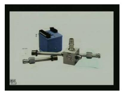
Of such a meter, you can see that this is the magnetic peak off and these are the pipe sections which you can connect with it and this is meter. So, you have connect the pipe section the turbine is already put inside it. So, this completes our obstructive flow meters and we take a quick look at the un-obstructive ones. For example, electromagnetic flow meter.
