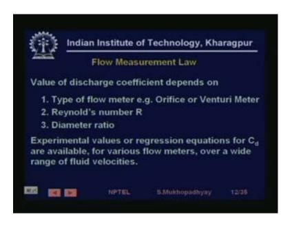
So, value of discharge coefficient depends on various things. It can depends on the type of flow meter there is an orifice or venturi and each manufacturer for each model will give you a detail description of how to obtain the discharge coefficient. Reynolds number and diameter ratio that is, what is the diameter of the upstream pipe and what is the diameter of the hole you are using.
