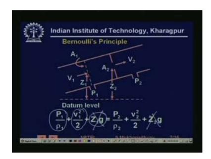
So, it says that this is the pressure energy, pressure energy is P by row. So, this is the pressure energy, this is the kinetic energy and this is the potential energy. So, it says that at any 2 points these are going to be conserved roughly. So, you get this equation if generally in our situation pipes are horizontal. So, if they are horizontal then Z 1 equal to Z 2 and you can ignore these 2 terms generally.
