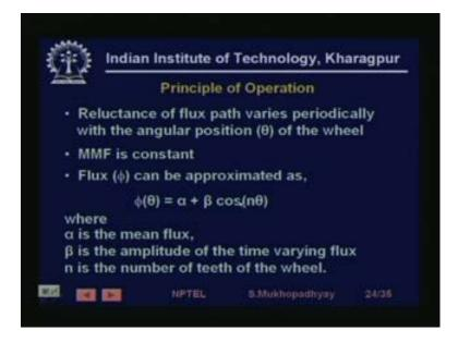
So, basically and what is this frequency of oscillation. This frequency of oscillation is actually n times, that is n times the rotational speed because once the turbine rotates n teeth will pass at this flux pulsation will go through n cycles. So, actually this flux
