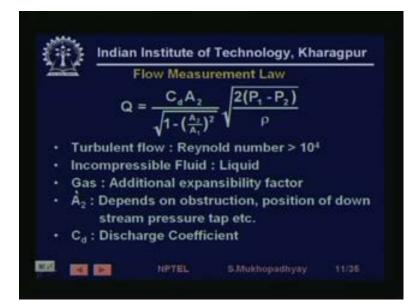
It turns out that the flow is actually related to, this is the pressure right, this is the P 1 minus P 2 is delta P which is the pressure difference across the obstruction. So, if you take one of the taps the upstream taps will have pressure P 1 the downstream tap will
