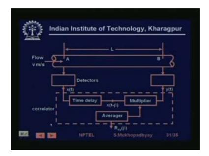
So, the last we will actually the last one is correlation flow meter. I will just explain the basic idea without going into details because there is lack of time. So, the idea is that if you want to this is typically used in situations where you have 2 phase flow that is you have bubbles in a gas or you have sand in air or you have line dust in air. You want to measure the measure the volume flow rate.
