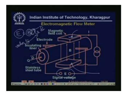
So, here what we are is let us see the parts we have a pipe. So, there is a pipe this is a pipe line, the actual flow is through this part. So, what we have created is that we have created a magnetic field these are coils. These are coil assemblies, these two. So, we have created a created a magnetic field by sending through this coils. These are actually schematic connections, when there is just shown that this is they actually connected to 2 sources.
