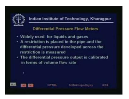
These are the most common and widely used for liquids and gasses in the industry and basic idea is that you place we will see it very soon. Basic idea is that you place a restriction in the pipe. That is the pipe is flowing at some point you obstruct the flow and you make a hole. So, now the liquid which was coming from this side, upstream when it meets the obstruction and the hole it has to flow through the hole.
