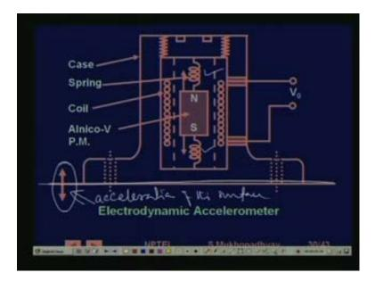
Acceleration sensing, is not very much used in the industry not or not too much when compared to that velocity and velocity and position sensing are much used. This is a typical configuration of an accelerometer, which is so. So, therefore, in fact, you know acceleration sensing is mainly used in the industry in the context of vibration sensing, which is sensor, which is widely used especially for maintenance and fault diagnostic purposes in all kinds of machines.
