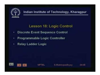
Having talked in terms of the continuous controls we shifted to logic controls which are also equally important and equally prevalent in industrial manufacturing which basically control sequence of operations of machines and generate they are often sometimes used for protection. Sometimes used for supervisory control where several sequences of control modes are executed, sometimes they are used for generating alarms they are more commonly used in discrete manufacturing.
