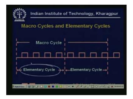
And the communication is actually organized overall into cycles called macro cycles and within each macro cycle. So, macro cycle is the basic cycle over which the communication is periodic and then within macro cycles you have elementary cycles. So, an elementary cycle is resided by the fastest by the device which needs to communicate the fastest, so let us see the next example we will understands it better.
