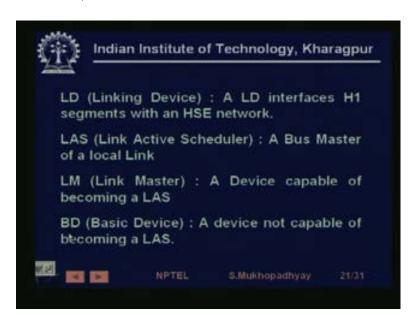
So, LD is a Linking Device as LD interfaces each one segments with an HSE or I do not know what HSE means, link master that is what I said, BD is basic device, a device not capable of becoming a link master.
