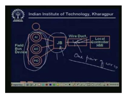
Contrasted to that, look at a this is here see what happens is that here you have these field bus devices. So, the field bus devices can be locally connected to a junction box or let us say a remote I mean some kind of a data concentrator, that is if they cannot be directly hung from a network, if they can be directly hung from a network that is even simpler. And then from this junction box actually starts the network, we will see this physical configuration just now.
