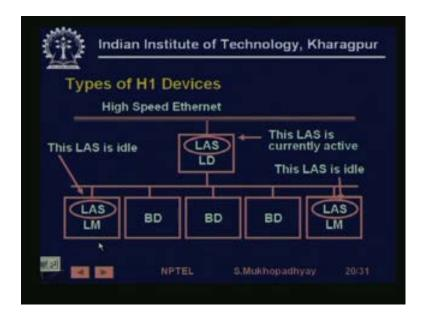
So, exactly same diagram which is repeated, so these are the link master and they are basic device, basic devices are not capable of becoming link masters or link active schedulers, while link masters are capable of becoming link active schedulers.
