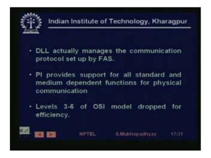
The data link layer actually manages the communication protocol it takes care of the digital communication details, error coding, parity checking, etcetera. And the physical layer provides a the electrical and medium dependence, so if you have wire, if you have RAF, then it has to be radio transmission, if you have fiber optics, then there has to be optical communication. So, all these details are handle by the physical layers and levels to 3 to 6 are dropped for efficiency.
