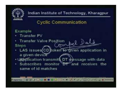
For cyclic communication, typically applicable in the case of control, so you know transfer process variable or transfer valve position, valve position is just an example. So, it continuously has to take the process variable, compute the controls and then output to an output device, so this goes on. So, this is an example of cyclic communication, so if there is cyclic communication, what the link active scheduler does is that it issues a CD or Compel Data token to a particular device.
