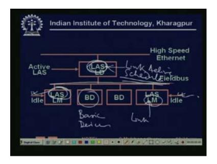
So, these are supported by the data link layer, so pictorially it looks like this on the bus, this is the field bus, there are various devices these are basic devices BD Basic Devices and these are Link Masters. So, LM is a kind of device which is capable of becoming a link master and there is among the link masters, there is a particular device which is called the link active scheduler. So, at this time this link master can also become the link active scheduler, but it is at this time ideal.
