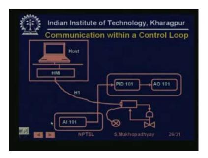
So, for example, take this loop this is a PID loop with say an analog input a PID and an analog output. So, these are you know actually you know on different devices and the analog input, so they are all on the network and the analog input this is the function
