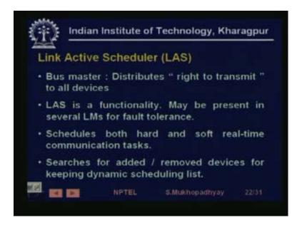
So, link active scheduler is as I said it is a bus master, which distributes right to transmit to all devices. It is actually a functionality some software which may be present several link masters or fault tolerance and it actually does this scheduling of the various, you know soft and hard real time communication task. So, soft real time communication task are those, which also need to be finished in time, but even if they are slightly delayed there is not, so much of a problem.
