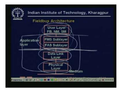
So, you have finally, the field bus architecture, so you have the physical layer, the data link layer and the application layer broken up into two parts. And then you have the user layer, which involves the function blocks which are you know abstract computing blocks which specify abstract communication. Let us, say between an analog input device and a process controller or a process controller and an analog output device.
