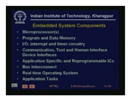
What do they contain; they are actually processor base systems. So, they generally contain a number of processors is there, they can be various kinds of, they can be micro controllers, they can be micro processors, they can be special purpose processors like digital signal processors, etcetera. Obviously, contain program and data memory all microprocessor base systems contain that and they contain special circuitry.
