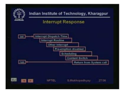
So, various systems have various interrupt response, so when an interrupt comes, first the interrupt is coming, then the interrupt service of routine is of control goes to the interrupt service are routine. Then, in the interrupt service of routine, one sees what are the other pending interrupts, which interrupts should be interrupt should be executed. In some times, some interrupts are so important, that temporarily what one has to do is that, it has to disable interrupt.
