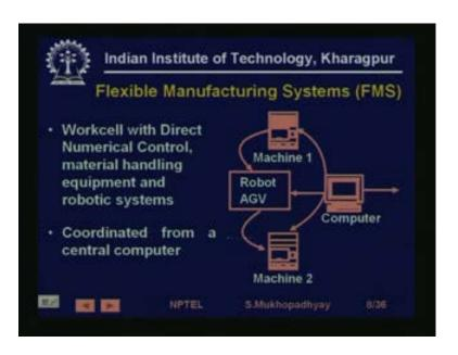
So, similarly when you are flexible manufacturing systems, flexible manufacturing system essentially it is coordination, so you have all these embedded systems. So, basically, you see that, once you have local systems, which have computational probability in them, because of the embedded electronics. Then one can easily think of the next, would be think of communication of digital electronic communication between these and so called smart devices.
