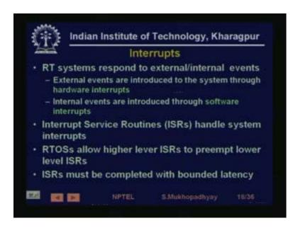
So, these are basic principles by which data transfer takes place and there is another very important concept of interrupts, it turns out. Now, suppose that, there has to be see the CPU is the actually to all the time doing calculations, various kinds of calculations. And now, it has to do calculations as well as it has to do input output in the sense that, it can do can read signals.
