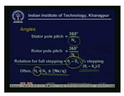
And we can understand that, if you have Ns number of stator teeth, then each phase is separated from the other by 360 degree by Ns. If you have the rotor pole pitch as Nr, then it is 360 degree by Nr, for the rotor tooth pitch and the rotation for full stepping is theta r minus theta s, generally theta r is less than theta s, so because it is a smaller.
