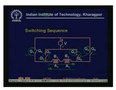
So, moving on now, how do you excite the stator phases, suppose let us take A 2 phase case. So, we have two coils A 1, A 2 and B 1, B 2 and I am showing them, basically you know, you either have, you assume that in the same figure, that either you have Q 1, you have Q 3, you have Q 2 and you have Q 4. So, assume that for the A 1, A 2 coils, you have these 4 switches and similarly you can have another circuit in which you have the B 1, B 2 coils in which you can have Q 5, Q 7, Q 6 and Q 8.
