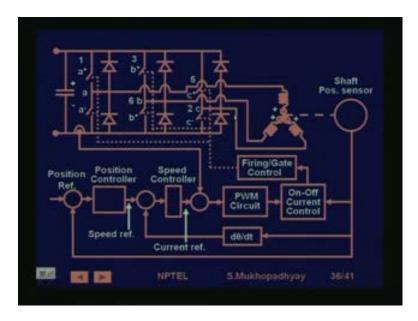
So, we come to a control scheme, so what we are basically doing is that, we want do just like in a DC motor, we want to torque control. So, we have seen in the case of DC motors, this is absolutely similar, in the sense that, if you have a position control loop, then we have a position reference and we give a position feedback, then we have a position controller, which gives a speed reference. So, it is actually a cascade loop, this we have seen in the case of the DC motor.
