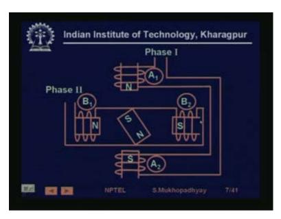
So, imagine this case, that you have these phases A 1, A 2 and you have these phases B 1, B 2 and you have we are just for simplicity, we are assuming that we have only one pair of rotor poles.
