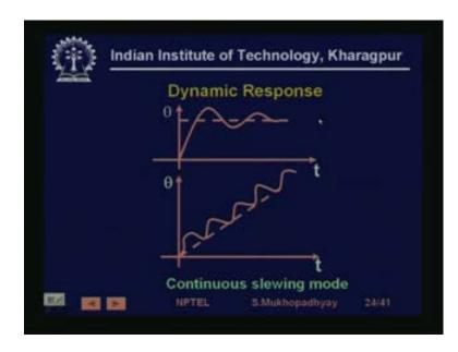
Now, it turns out, generally when we are using a motor, we want to move it as fast as possible. So, if you are giving pulses slowly, then what will happen is that, you excite one phase motor rotor will come and will stand still. So, it will actually stop at that position, it might excite, because of it is inertia, it might give us a little overshoot. So, it might give a little overshoot, but it will stop, but if you let it stop and then excite, then you are taking more time.
