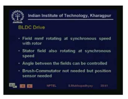
So, in the brushless DC moto,r that is why it is called a DC motor, because here the field and the armature m m f's are kept perpendicular, nearly perpendicular, but the field m m f is rotating at synchronous speed with the rotor. See the rotor is rotating and you do not have any brush, so the rotor m m f is rotating. So, to keep them perpendicular, what you do is that you sense the rotor position.
