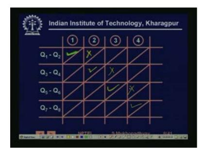
So, what happens is that, so we the switching sequence like for example, first you what you will do is that in the first place, you will sequence switch Q 1, Q 2. So, you will switch Q 1, Q 2 let me change the color, if you switch Q 1, Q 2 then the rotor will get aligned in one direction. Then, in the second step, you will switch off Q 1, Q 2 this you can do, this is one strategy and you switch on Q 3, Q 4.
