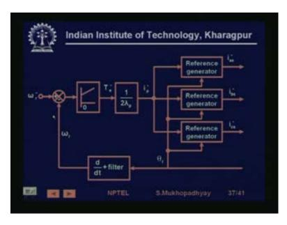
So, this is exactly the same thing, that we are taking, this is just a speed control loop, so the speed reference is there, real speed, then T i control. Then, this is at a proportional controller and then you generate the current references.
