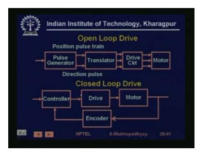
So, you can have two kinds of drives for stepper motors, either open loop or closed loop, in open loop drive, we are not taking any feedback. So, you are kind of assuming that every pulse, that you have given has been executed by the motor; obviously to this assumption will be satisfied, when your pulse frequency is low. So, you are moving slowly this can be satisfied, provided the load torque is not too much.
