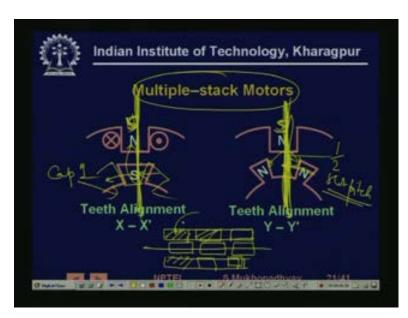
So, what happens is that, so there are the same number of teeth, but they are slightly offset, in such a way that when one tooth, this is for one cap, say cap 1, when one tooth will align with the stator tooth at one end, the other teeth will actually align with the slot. So, this aligns with tooth and this aligns with slot, so what happens and you see this is S and this is N, because there is an internal electromagnet in that.
