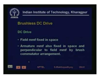
So, we will first see, how, why BLDC drives are called BLDC drives, this is a very important concept to understand. So, in a DC machine, you have the poles are fixed. So, the poles are fixed on the stator, it does not move, so you have fixed, so the field m m f is fixed in space, it does not move. Now, the armature is excited, so the armature is a coil, it is excited by current, so that also creates an m m f.
