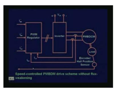
And then this current reference, will actually go to a PWM regulator, which will really create the switching not only to have the current at certain level, we will also have the sense of switching, such that the m m f's rotate in the proper direction. So, this is we did it in a fast manner, but you can understand that this is exactly similar and the main key
