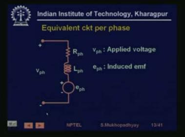
If you look at the equivalent circuit per phase, then it is just a coil, so it has a resistance, so you are exciting it by a phase voltage and there is a resistance, there is an inductance and there is a back here, so that is the induced e m f.
