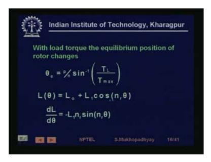
So, this is some expression, which shows that the inductance is varying as there is a DC component and there is a pulsating component, like I was showing. And then d L d theta is actually is a sinusoid, so the torque is also is a sinusoid.
