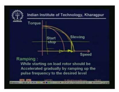
So, if you see the torque speed characteristic will see that, when one is trying to start the motor, when the motor has no inertia, it is not moving, it is actually at rest, then initially you have to start it, you cannot give very high frequency pulses, because if you increase the pulse frequencies, then actually what will happen. If you increase pulse frequency too much, that before the rotor can move another phase will be excited.
