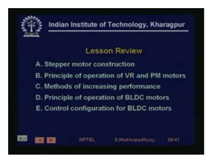
So, coming to the end of the lesson, we have seen stepper motor construction principle of operation of variable reluctance and permanent magnet motors and methods of increasing their resolution and speed of rotation by slewing. And we have also seen the basic principle of operation of the BLDC motor and we have seen one control configuration of BLDC motor and seen that it is just like a DC motor, except for that PWM switching, which creates the stator phase to rotate.
