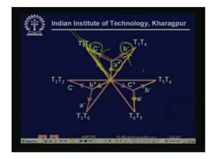
We will go to the next diagram, so in the next diagram you will understand that how the stator m m f direction is changed. So, if you have the coil a in a certain directions, say one terminal positive and the other terminal negative, we call it a plus. So, the m m f is in this direction, if you change the polarities, it will be a minus, this is in the opposite direction, similarly you have b plus and b minus and you have c plus and c minus.
