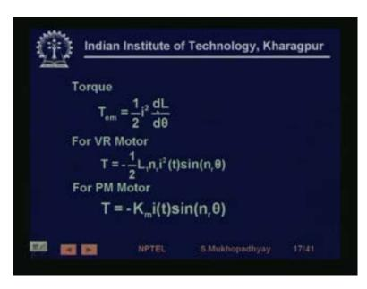
And you determined will be the torque is half I square d L d theta, so it turns out that, these are expressions for the permanent magnet and why this happened. So, these are the torques generated by the permanent magnet motor, in the permanent magnet motor flux is constant. So, this the torque generated on the permanent magnet motor and this is the torque generated on the variable reluctance motor and finally, what will be the torque generated.
