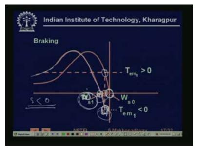
Now, for braking, so you know, you can do this torque speed control by varying the stator voltage and the frequency and you can, you see that you can also use it for braking. So, let us take the case of generative braking, so in this case what we can do is suppose that this we were operating at this synchronous speed or at we were giving this sort of supply frequency and this was the rotor speed, this was the rotor speed.
