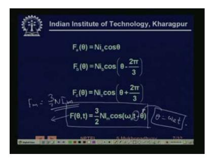
You know which are rotating, which are distributed in time in phase by time phase by 2 pi by 3, so and the Mmf if a current Ia flows, the Mmf due to the current in the a coil with theta if a constant current Ia flows is given by this while for Fb it is displaced in space by 2 pi by 3 and in Fc it is displaced by plus 2 pi by 3. So, now it is very easy to
