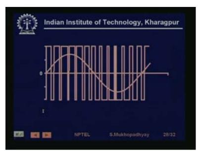
We are not going into this, so this shows that if you have a PWM switched wave like this then it its Fourier transform will generate an ac wave, it will generate fundamental like this and its harmonic content will also be improved over the square wave VSI in the sense that lower frequency harmonic will not be present.
