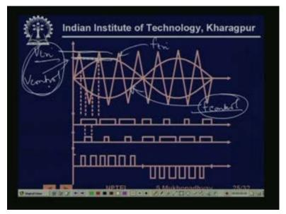
So, going back you see that we have two kinds of modulation, firstly, this is V triangular, go back to the white pen, so this the V triangular and this the amplitude of the V control. Similarly, this V triangular has some frequency f triangular and this has some frequency f controller, so we can see that by varying, we can change the frequency by simply changing f control of course, we have to assume that f control f triangular is much, much higher than f control.
