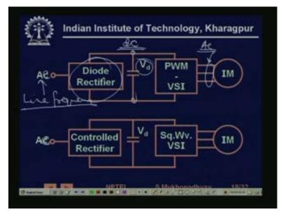
We need to have, so as far as the power electronics is concerned, we are trying to make a voltage source, supply source which will generate three-phase balanced ac supply to the stator, but whose voltage and frequency can be changed. So, how are we going to change, so that it can be achieved in two ways one is that so; obviously, we have this is line frequencies and this is also ac, but this is at a different this is at a controllable frequency and usually quite it may be high frequency.
