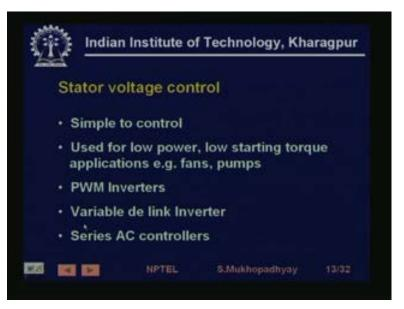
So, in summary stator voltage control, it may be simple control for example, if you are having an inverter, just these if you control the dc input supply voltage of the inverter that will give you stator voltage control. You can have even simpler, you can have series ac controllers things like you know triax using which you can do stator voltage control, but they are used for low power and low starting torque operations like you know typically fans and pumps whose torque varies with the load.
