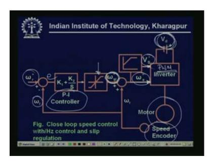
So, now, so you see that using we have seen that we can how we can vary voltages and frequencies, so now if you want to implement a variable voltage, variable frequency control loops, so what happens is that this is the motor. So, we are sensing the speed, this is a speed sensor, speed encoder you are feeding it back to the controller omega r. So, the controller is see this is the reference speed, this is the speed error and this is the PI controller, typically a PI controller is used.
