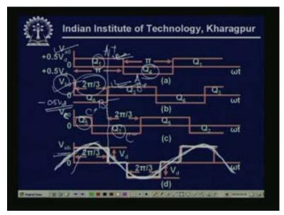
So, now you see the previously we have seen that if we switch on, so look at this, so here if we switch on this immediately this goes to plus V, so suppose this is a plus Vd this is supposed this 0. So, immediately it will go to plus V if we switch on this immediately this terminal will go to 0 or may be if we can call it plus V by 2 minus V by 2 in which case anyway it will go to the negative terminal, this is going to the positive terminal.
