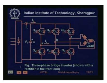
So, this is what you do, so you have a, this is again a PWM three-phase with a motor connected, so there is nothing new in it. So, if want to generate three-phase supply then you use three waves, Va Vb Vc and then with respect to these three waves you actually generate the PWM waves, so that is the way it is done.
