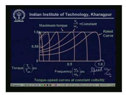
So, these are the you know torque speed characteristic at various this is again this is speed omega r by omega s and this is torque. One thing is interesting, first the maximum torque level can be maintained, so you have, you can achieve a very high starting torque with this control. They are almost like the maximum torque, so these kind of drives are going to be useful for machine which start on load.
