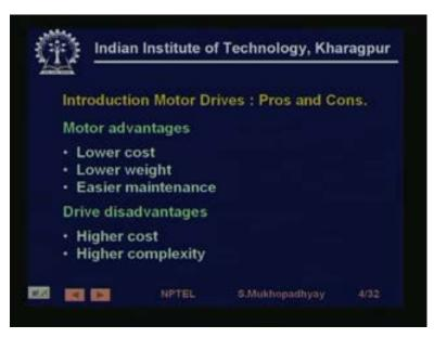
So, to this end, first let us see what are the advantages of an induction motor, see these advantages we are considering against what, we are considering visa V typically visa V DC motors. So, what did we see in the DC motor that DC motors have higher weight, their armature cost weighs more and cost more, basically because of the brush commutator arrangement.
