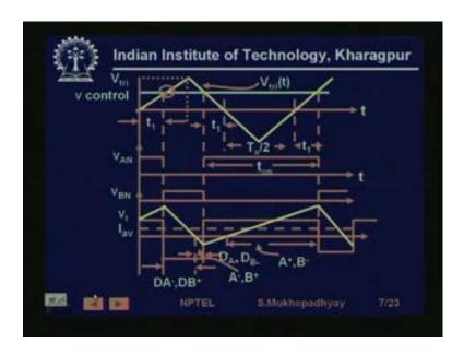
So, you see that as we vary, let us note this, why it is called it is also called PWM control is because of the fact that as you make the control where either speed controller makes the control voltage level go up and down. So, what happens is that you see that during this time A plus and B minus rather A minus and B plus are on and during this time A minus and B plus are on, so whenever, so you see that this voltage pulses.
