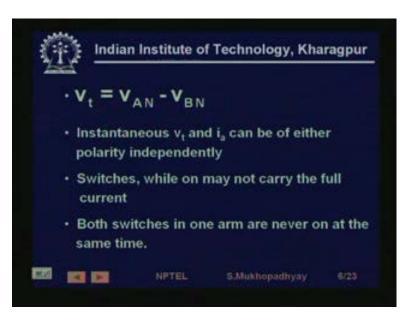
So, having said that we will first note that the terminal voltage across the armature voltage is basically VA minus VB, so we note that and as we will see that in this circuit, the instantaneous terminal voltage and currents can be of either polarity, you can have you can have positive positive, positive negative, negative positive and negative negative. So, they can be changed independently, it is not necessary that if the voltage is positive current has to be positive.
