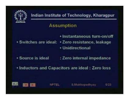
There is zero resistance, but the switches are unidirectional you must remember that in all other respects is like a switch, but expecting for the fact that we cannot have a current flowing in the opposite direction in the switch, these are the properties of this electronic switches. We will also assume that the source is ideal that is the DC source is ideal, it has zero internal impedance and if it has zero internal impedance that is, it has zero regulation.
