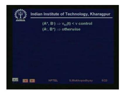
If the triangular voltage instantaneous value is less than V control then we are going to have A plus and B minus as on and if it is not then we are going to have A minus and B plus as on, so let us see what happens. So, now we go back to our circuit, so this is my triangular wave control static.
