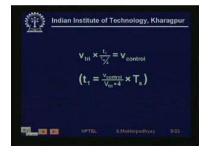
So, suppose a time t 1 the triangular wave becomes equal to V control, so therefore, this equation will hold and therefore, this time once you are given V control and we are given
