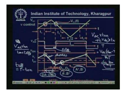
So, this is what is happening, so the movement V control is as long as V control is less than V is control is greater than V triangular, we have A plus and B minus on. So therefore, voltages VAN is positive and VBN is zero, B is at the neutral voltage. Similarly, the movement it crosses this VAN goes to zero and VBN goes to positive, so if you see, if you want to draw the terminal voltage then it will look like, so initially it will be VAN minus VBN, so it will be positive VBN.
