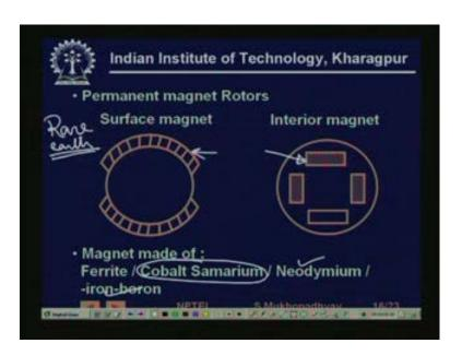
So now the armature is now, so now the field has come to the rotor the DC field, see why brushes were required because you wanted to feed armature current into the rotating. Whenever you have a, you want the feed current into a rotating body you have must have either a brush or a slip ring kind of arrangement, which is difficult to maintain, so therefore, what we do is we change the places where we want to give supply.
