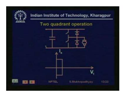
Now, this is the basic four quadrant operation, now we look at simpler versions of this for example, we look at two quadrant operation, If we have two quadrant operation then we have only this circuit. So, you see that we are only using one arm, the previous circuit that we have seen this is the DC source, we are using only one arm and we are correcting the motor across this across this arm, the other arm is fixed to the ground, so then what happens is that, now with this circuit.
