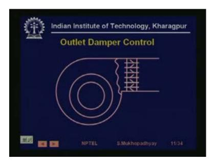
The next control which is used is called the outlet damper control for the fan, so outlet damper means basically a damper means you know is like a set of veins, you know just like say sometimes on the you must have seen what is what are these called there, when you put something on the windows to keep out the sun. So, you know there you can change gaps you can move them either you can keep them like this or you can keep them like this, so that some air can flow.
