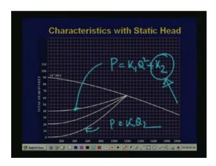
So, only thing is that in the case of the pump there is a there is sometimes pumps operate with a static head, so if you have a static head then the load characteristic can be this is one with without static head where P is equal to K Q square type of characteristic, but a pump can also operate with the static head where the characteristic is P equal to K 1 Q square plus K 2.
