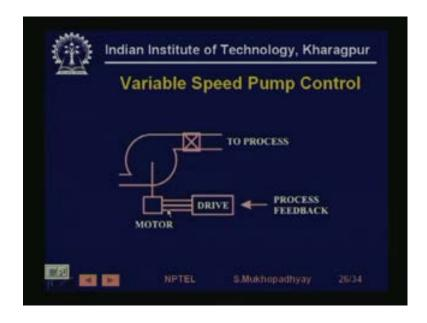
This is a variable speed pump control, so you have you have a constant speed drive one we are controlling is either you have a constant speed motor drive and you have a valve or you have a variable speed drive of the pump, depending on the feedback depending on the load. Basically, that the drive has to be controlled and some speed reference has to be given, we will see in our future lectures as in detail as to how these how the speed of a motor and a pump can be controlled next.
