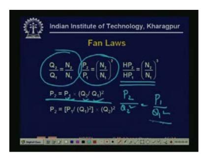
Now, here before we discuss that we need to understand what are known as the fan laws, so what are the fan laws the fan laws say that in a fan roughly Q 2 by Q 1 equal to N 2 by N 1. If you operate if you change the speed the curve shifts in such a manner that on the Q axis you are going to get proportional to these things and P 2 by P 1 equal to N 2 by N 1 square, so the horse power variations are going to be into by goes to vary as N 2 by N 1 Q.
