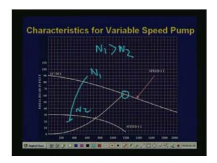
Now, if we control the speed as before the pump characteristic will now come down, this is N 1, this is N 2, and N 1 is greater than N 2, so the operating points will now shift from this to this, just like a previous case.
