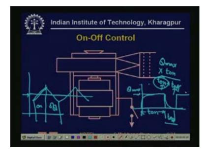
Now, let us see that what are the various ways of controlling one of the easiest ways of controlling air flow is to switch on and switch off a fan you know this happens regularly, if you see a if you see home air conditioner, you must have notice that the fan I mean the in that case the compressors which is on and off. So, it is a kind on-off control, so in a similar way if you want to control flow, then you can also switch off and switch on the fan.
