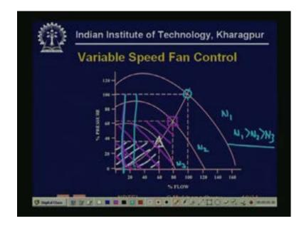
So, we see this variable speed fan control, so now what happens is that if you want to reduce the speed, we are not going to put any damper or any valve in other words the characteristic of the system remains unchanged. Now, we are changing the speed of the fan, so the fan characteristic shifts, so this is let us say N 1 this is N 2 and this is N 3 and N 1 is greater than N 2 is greater than N 3.
