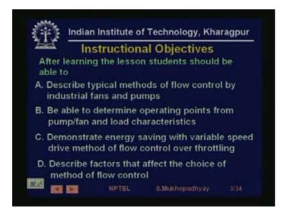
So, it flow can be of gas or liquid, so accordingly we have either what are known as fans or blowers or we have pumps, fans blowers and pumps constitute an enormous very significant fraction of the loads which are driven by motors and motors which consume a large amount of electrical power in the industry. So, they are very common and common applications and very significant from the energy point of view.
