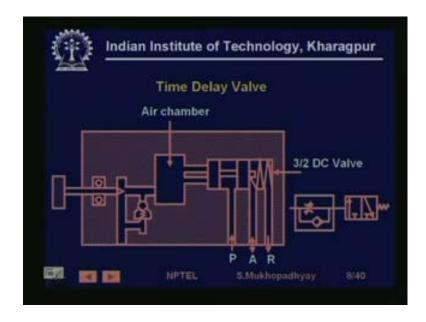
So, you see that air this is the pilot port, so the air comes and fills this chamber after it after this, so pressure builds up slowly because of the chamber and then, it shifts the valve then it actually applies the pressure on this pool and that will shift the valve. So, this is the basic mechanism by which time delay is created.
