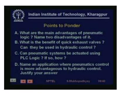
So, points to ponder there are some question what are the main advantage of pneumatic logic, so we have already stated that and what are the disadvantages obviously, disadvantages in terms of speed and complexity. What is the benefit of quick exhaust valves we have and can they be used in hydraulic control of course, cannot they of course they cannot be can pneumatic system be actuated using PLC logic if.
