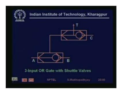
This is just an example which shows that by you know by casketing this shuttle valves you can have a three input OR gate also. So, that is, so you this at this point you have pressure applied when it A or B and then that is applied to one port. So finally, the pressure is applied to the system when you have A or B or C, so it is a three input OR it is a it is a three input OR.
