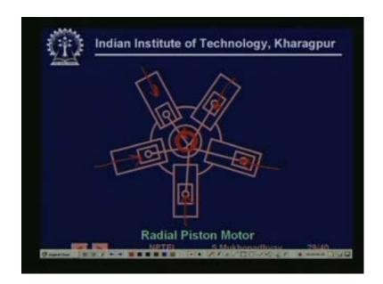
So, this is a picture for a radial piston motor, so you see that if you apply pressure to this if you apply pressure to these pistons in sequence cyclically then, this because of this mechanical arrangement there will be there will be a there will be a rotational motion. So, this is naturally this is of a positive displacement type, there is at a in every cycle of the piston movement a certain amount of air is air goes through the system. Similarly,
