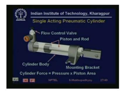
So, you see this is a cylinder where this is a cylinder body you can see the piston and the rod which gets connected to the load you as we have seen that you can put a flow control valve here sometimes, you can put a quick exhaust valve here. So, this is a normal pneumatic cylinder, similarly you can have pneumatic motors.
