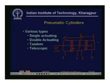
So, in such cases one uses you know pneumatic cylinders and they can be of various types, they can be single acting where may be spring loaded, so from one side you apply the pressure. So, it moves only this side retraction is may be by a spring generally it is by a spring, so that you actually do not require motion on the other side, if you have a double acting cylinder then the connecting rod can move this way, that way in both ways and you apply.
