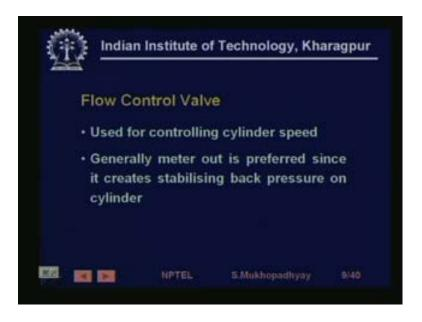
Similarly, you have flow control valves, so in flow control valves are mainly used to have a controlled speed of the actuator especially when it is raising load, so you know sometimes as we have mentioned in hydraulics that sometimes we want that, sometimes we want that while it is retracting it should be at high speed to save time, but while it is driving the load it should be at lower speed.
