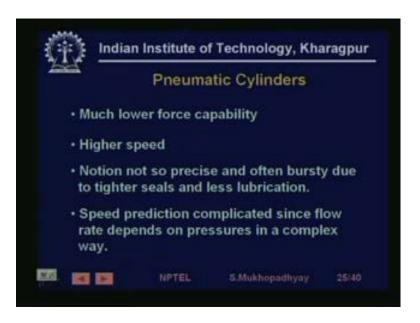
The pneumatic cylinders have lower force capability and, but they have higher they have high speeds because, they are generally driven against slower loads it also and the, this is not notion this is motion, so motion is not. So, precise because of the fact that you know there is the fiction is higher and there is seals are tighter, because to prevent air leak, so that you know the energy developed by the pump is not wasted.
