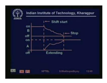
So, you see that you can start at a when see at the at a certain point you can start shifting and then, as it as it shifts the pressure at one terminal will fall and the pressure at another terminal will end will raise and then, when it raises up to a certain level then the then the shifting has to stop, so that, so that a certain amount of pressure is reached across the cylinder.
