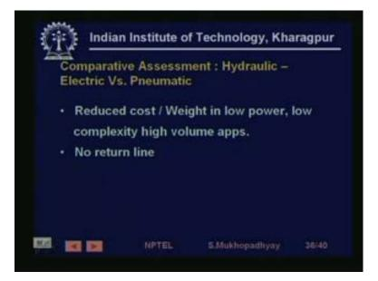
Now, we come to the last topic which is the comparison of hydraulic and hydraulic electric and pneumatic systems, so it turns out that for low power low complexity high volume applications of course, a generally pneumatic system sometimes tend to give an advantage that is why it is used in you know things like in use in pneumatic tools in large you know assembly shops like in an automotive factory.
