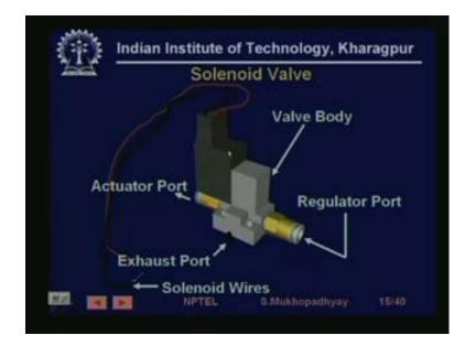
For example, this is a this is you know a typical solenoid valve, so you directly can drive current into a solenoid valve which will pull the spool, similarly you can have electronic interfacing, so this is a slightly more elaborate configuration.
