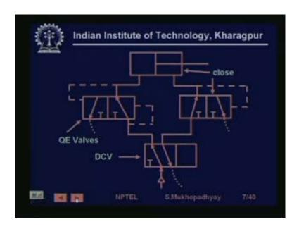
So, this is an actuator which is being driven, so what happens is that the air flow this is the DCV, so the air the air flows into this goes through this and raise the actuator, so the actuator moves when it moves it actually expels the air. So, you know it actually expels the air, so because this is a your know pressure driven, so when this pressure line increases this valve, this valve is going to shift as we have shown the mechanism.
