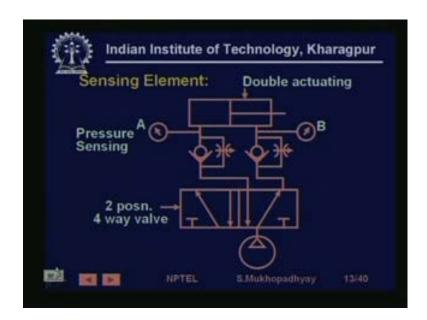
So, exactly that is shown, so you see that you are sensing this pressure A and pressure B and then, you have to use an appropriate logic to actually drive this valve, so that a certain amount of pressure is force is developed.
