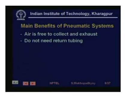
So, the main benefits of pneumatic systems is that, air is free to collect and exhaust, so you know, it is simply collected you do not need to buy it and therefore, it is cheap and it can be exhausted into the atmosphere, so you do not, so you do not need return tubing. So, you see that for hydraulics you need one pipe or tube for carrying the fluid to the place of work, namely the load and you need another pipe or tube to bring it back.
