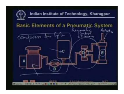
So, let us look at the basic elements, the basic equipment in a pneumatic system, so we start with the compressor, so this is the compressor A, then after the compressor you have a, you sometimes have a check valve B, then you have an accumulator or reservoir of compressed air, this is very much necessary in pneumatic systems to improve response speed, as we will discuss. After that, you have you can have a various kinds of equipment.
