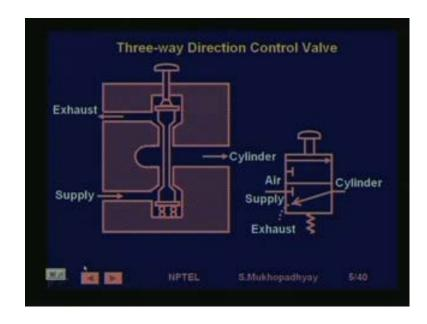
Then we come to 3 way valve, basically this is a, there are 2 ports, one is supply, the other is exhaust and again as you can see, this is also spring loaded, so when there is no this is when this is button operated, so when the push button is not pressed, then this is supply is closed and cylinder is connected to exhaust.
