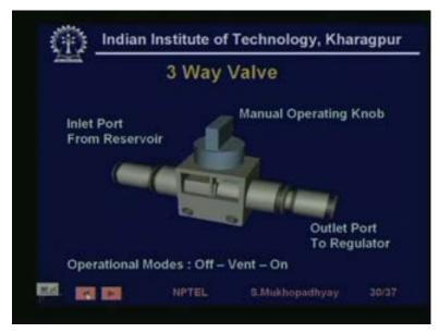
For example at, this is a typical 3 way valve, which is manually operated using this knob and it has three operational modes, so namely off-vent and on. So, it can be made off, in which case air will not flow, if it on then the air will move from inlet to the outlet and if it is in vent mode, then the inlet and outlet will be connected to the atmosphere. (Refer Slide Time: 42:14)
