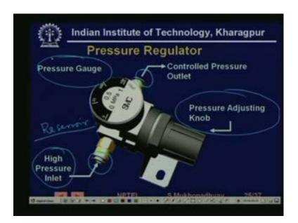
So, this is just a typical picture of a pressure regulator and so you have this high pressure inlet, you have the low pressure or the control pressure outlet, so this is going to the system or the equipment, where the pressure is needed, this is coming typically coming from the reservoir. So, now the pressure setting can be adjusted by this pressure adjusting knob and often there is a pressure gauge, so that you, one can see that the inlet pressure variation.
