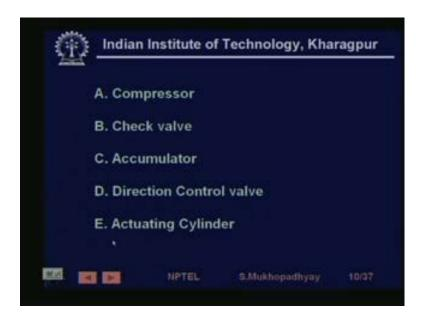
So, A compressor, B check valve, C accumulator, D direction control valve and finally E is actuating cylinder or actuator.
