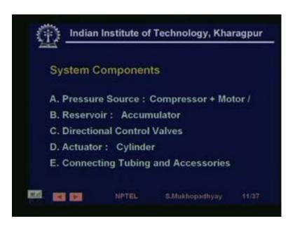
Now, in system components, compressor is a pressure source, sometimes you can have a linear air cylinder or sometimes you can have also have a pneumatic motor, reservoir or accumulator, reservoir accumulator is very much necessary. Because of the fact that pneumatic system response tends to suffer, because suppose you want to move a cylinder, then you have to create the pressure create pressure on it.
