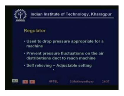
So, a regulator is used to drop pressure at to a level which is appropriate for a machine and it prevent pressure fluctuations on the air distribution duct to reach the machine and settings generally, for regulator settings can be adjusted and it is self relieving in the sense that, if the pressure I mean there is too much inlet pressure then it is it generally relieves that pressure.
