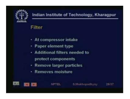
So, then the filter can be connected at is generally connected at compressor intake and various types are possible, paper element type is a popular one and sometimes, you put additional filtering you need, just before the equipment to, you know ensure further that these are, that the that your components are protected and so it removes the large particles and it also removes moisture, because especially particulate matter and moisture.
