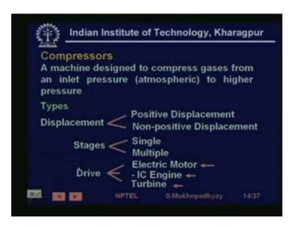
Then we look at compressors, compressors are the mechanics which are designed to compress gases from an inlet pressure which is generally atmospheric. So, it takes air from the atmosphere, filters it and then compresses it to a high pressure, and there are, this mechanism can be of generally of two types; one is positive displacement, where each kind a certain given volume of air is converted from the atmospheric pressure to high pressure.
