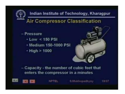
So, compressor, so is for example, this is a typical compressor where, you know this is we can see from the picture that this is a IC engine driven compressor and this is the compressed air supply. So, that is the accumulator and it looks like a portable just a picture which is downloaded from the net, so compressors are available at various, you know sizes or capacities and so 150 psi, up to 150 psi would be low pressure, 150 to 1000 is medium and greater than 1000 psi will be high pressure.
