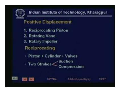
So, positive displacement could have involve linear motion or could involve circular motion, so you can have a reciprocating piston type or you can have rotating vane types or rotary impeller. So, either you have rotational designs or you have translation designs, but in each case, one cycle of rotation or one cycle of, to and fro motion will take a certain given volume of air and push it take it to the low pressure inlet port and push it into the outlet port.
