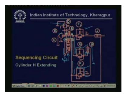
Next we have a sequencing circuit, so in the sequencing circuit what is happening is that, here now, in this example, we have more than one cylinder. So, far what we have been doing is that, we are we have handled only one cylinder, but sometimes it happens that, you need to operate multiple cylinders and for example, suppose you have a wood working machine, you have a plaining machine. So, before you plain the machine, before you start moving the plaining cutter, you have to hold the job.
