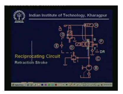
In the next stroke, now we have an, we have a retraction stroke, so what happens is, when it reaches the end, it operates this limit switch at the end, at the extreme end of the extension stroke. That limit switch is actually connected to the solenoid, in such a way that immediately when the limit switch is made or switched on, this solenoid is put off. So, when the solenoid is put off, this directional valve assumes the right position, so what is happening in the position.
