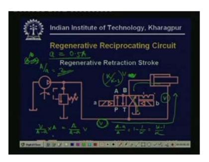
In the retraction stroke, now you are in this position, so now, this simply this is the path, directly this is the path, that is there is no fluid addition or anything. So, now what is happening is that, if this is V, then this is V and obviously, because it directly goes into this and what is going to be this, this is going to be naturally this will be, so A into, rather A minus a into V, suppose it moves distance x, so if this is V suppose the area is half, then this side it will be k into V.
