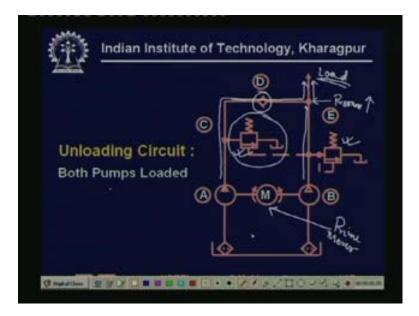
So, if I come to our first circuit what is that, in this circuit, it is called an unloading circuit, so there are, see the circuit there are two pumps, can you realize that this is the, this is actually hydraulic pump, this is a hydraulic pump. This is also another hydraulic pump and they are being driven by a common motor, so this is the prime mover and these pumps are actually connected in parallel, this is where it is going to the load or the system.
