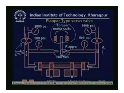
Next we see another type of servo valve, which is a flapper type servo valve, so you see what is happening here, what is happening here is that, again here the, this is the valve, the valve is being moved by applying pressure here or pressure here. So, you have to create a differential pressure, how do you create that pressure as such, this is also this is 100 psi, this is a you know restrictor, so it is a pressure reducing valve, so simply a series obstruction.
