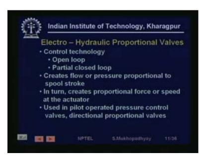
So, we can have open loop technology where we, when can you use open loop control, you can use open loop control when, this we have studied in control theory, that why do you need feedback. You need feedback, when you know that the system model can change and there are lots of unknown disturbances, so if you have this sort of situations then you use closed loop feedback control, but in a situation, but for closed loop feedback control you need, you may need an expensive feedback arrangement.
