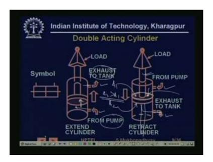
For double acting cylinders are also very simple devices, so here you can see that you can, these have two ports, one is pump, one other is tank. Actually, you have two ports, so one, so if you connect this one to pump and this one to tank, then the fluid will enter here and will go out here and we will be pushed in this direction. On the other hand, if you reverse that, if you take this one to pump and this one to tank, then fluid will enter here and will go out through this direction.
