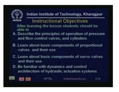
Describe the principles of operations of pressure and flow control valves and cylinders, basic components of proportional valves, learn about basic components of servo valves and be familiar with the typical, you know control architecture of hydraulic actuation systems, these are the instructional objectives of this lesson.
