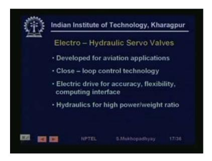
Now, let us come to servo valves, they are they were typically developed for aviation applications, because in aviation you have to make very precise movement of this control surface of the aircraft, against very heavy load which is aerodynamic, because the aircraft is moving at huge speed through the atmosphere. So, very precise motion has to be created against high load, it is for these purposes that these servo valves are originally developed.
