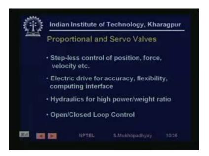
So, it is, so therefore we use, what are known as proportional and servo valves, so you have here, what the I mean, the advantages are that you have a step-less control of position, force, velocity etcetera and you can drive this, these are typically electrohydraulic valves, so that you can drive them accurately using, mainly using current and so that you can sometimes have computing interfaces, one of the major areas of application is avionics.
