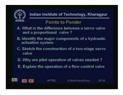
Last, points to ponder, what is the difference between a servo valve and a proportional valve, is it in terms of feedback, is it in terms of performance accuracy or is it in terms of structure, drive, what. Identify the major components of a hydraulic actuation system, this is the one of the major, this question you should be able to answer, because this is
