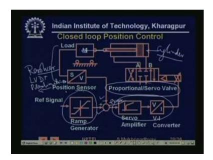
How do you do closed loop position control, so very simple, this is a, see this is a position loop, so you have a proportional or servo valve here, that is driven by this electronics and moves the load, this is the cylinder, which the position of the load is sensed by the position sensor, this is a position typically an LVDT, sometimes a potentiometer, could be a resolver if it is a rotary and these two are compared this and the error is fed.
