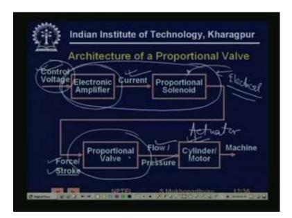
A typical proportional valve will have these elements, so it is operated by a control voltage, which can be given manually or which can come from a computer. Then, there is usually a set of electronic circuits, which do various kinds of things, which do filtering, which will do amplification, which can do, sometimes if part of it is digital they will do digital to analog conversion and there can, there is a main thing is that it must add some power.
