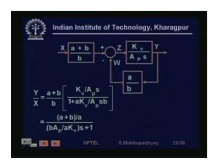
So, you have an effective feedback arrangement where, what is coming this is the motion created by the motion X, this is the motion created by the feedback W and this is the net motion Z, at any point of time and that is going to create, so motion creates a flow and this is a flow again. So, that is going to create a volumetric flow, that divided by A P will give you the linear motion, A P is the area of the piston, that integrated 1 by S will give you the motion of the plane W.
