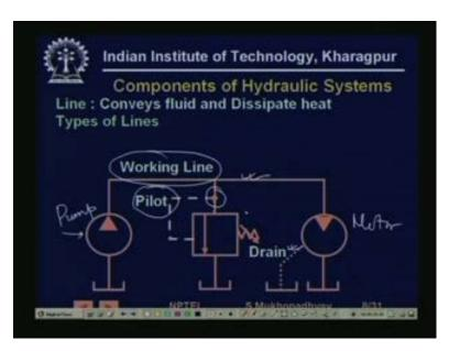
Now, how does the liquid flow, the liquid actually flows in pipes, now this is, you know one of the this is a kind of drawback for the hydraulic system in the sense, that you have to have an, you have to have some piping. And, you not only have to have piping, from the pump to the load, as the liquid is flowing, because it is a liquid, so you need to also have the return line, so that adds some cost and some maintenance.
