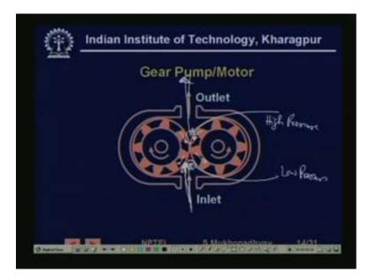
On the other hand, look at gear pumps, in the gear pumps, you have meshed gears, so what is happening, you can you can imagine, that as this gears are rotating, so as this gears are rotating in this zone, as this you see this teeth is moving this way, and this teeth is moving this way. So here, it they are compressing the fluid and some high pressure region is created, on the other hand, here the meshed teeth, I mean the actual drawing is
