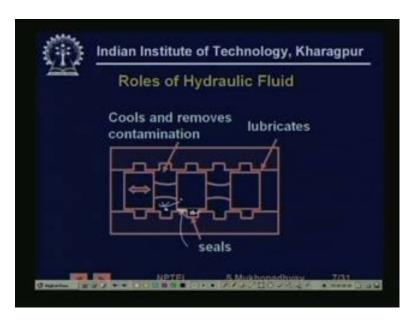
Now, what does a, so this is a picture which says, what the hydraulic fluid does, so you see that, the hydraulic fluid apart from the fact, that it lubricates, it cools and removes contamination, there is one point, that I did not mention, that is it seals also. So, because of the viscosity of the oil, if you have, if you for example, the fluid here and the fluid here, are going to be effectively sealed by this liquid film, so this liquid film here, is going to act as a seal.
