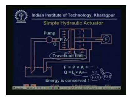
So, let us look at a simple hydraulic actuator, so you see that, we are creating a pressure here, so that creates a force F depending on the area and the pressure, so F is equal to P in to A. Now, let us look at the velocity, what is the volumetric flow rate Q that is equal to the area into L, where L is the travel per unit time, in other words L is the velocity. So, F is equal to P into A and Q is equal to L into A or in other words we can write, that V is equal to Q by A.
