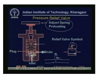
So, this is a simple pressure release valve, so you see that, this is the inlet, this is the inlet, so very simple, this is the drain, so actually this valve, can be connected across a
