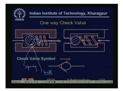
So, first the check valve, so the check valve what does it do, it will allow flow in one direction, but not the other direction, and it is, so you see, how it works, very simple, this is a, this is one of the constructions, there are various kinds of check valves. In fact, the
