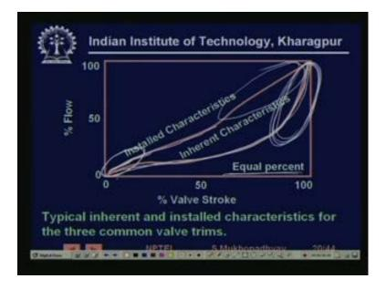
In effect what happens is that, for example, this is the case of an equal percentage valve, at some delta P, so you see that the inherent characteristic is almost like an equal percentage nearly. On the other hand, if you put the valve, that valve into along with a pipe and a pump and a system, then initially, there is a lot of fresh delta P available,
