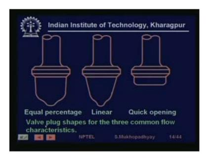
And, now how are these characteristics realized, they are realized by various profiles of the plug, so in the case of the globe valve here, say we have there are three kinds of, these are three plugs, which realize equal percentage, linear or quick opening characteristics.
