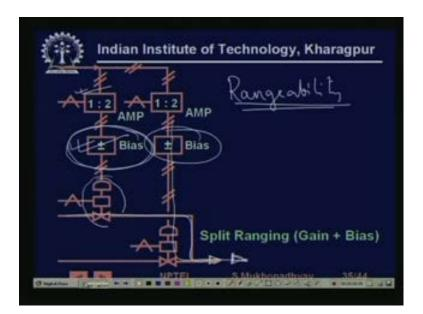
Similarly, these are sometimes you know, there is, there is a very important quantity for a valve called range ability. So, range ability means, that what is the maximum to minimum flow ratio, so the maximum flow to the minimum controllable flow is it to say, so valves can have, you know some sometimes valve manufactures claims, that they have you know, 10 is to 1, 15 is to 1, 13 is to 1, 30 is to 1, kind of you know range abilities.
