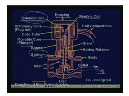
So, what I was saying is that the electro hydraulic valve pilot stages solenoid valves are used and this is a particular construction of the solenoid valves. So, you see that this is the valve, this is the plug, this is the plug, and this is the closed position shown, so this is inlet and it is flowing through this, and going to this is the flow of fluid, there is a spring loading, this is here the stem is actually connected to a magnetic core, which is called the plunger.
