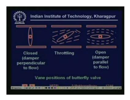
So, this is the picture which shows that, so look from a side, when the disc is, in this position then the damper or then the damper is perpendicular to flow and the valve is closed. When it is moving in and throttling or controlling the flow and when it is in this position, then when damper is parallel flow, then is completely open.
