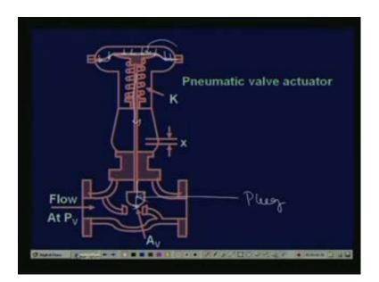
This is on the other hand, this is the particular pneumatic actuator, so again same thing, again you have a plug and you have these ports. So, what happens, is that here, by spring force, this is a particular valve, where you can close the valve by applying air in the
