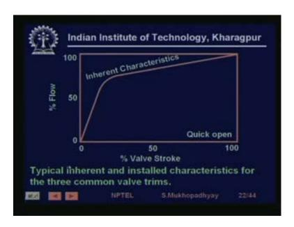
This is the characteristic for an inherent characteristic for a seeing, and they are not so much use, so the installed characteristic is actually not drawn.
