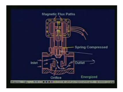
On the other hand, when this will, you see that, if this is energized, then the flux is flowing like this as shown and it is pulling the plunger up. So, when the pulling the plunger up, then this spring is compressed and this opening is, opened and the fluid flows, so this is the way a solenoid actuator will work.
