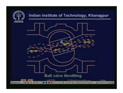
This is this picture shows how when a ball valve rotates, then how the flow throttling takes place, so you see, that as it is rotating. So this, the effective area of flow, they gets reduced, so as it rotates slowly the effective area of flow, will get reduced and therefore, the flow will get reduced, so the flow gets throttled.
