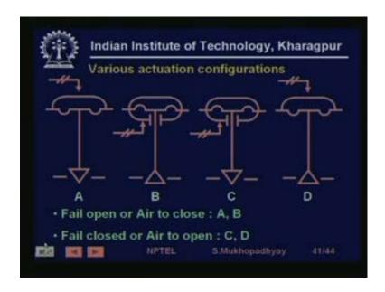
The lastly, you know valves are, one has to put and have a view towards, what will happen, if the actuation fails, because you know sometimes this flows, can actually cause explosions etcetera. So, valves are constructed in various configurations, which are shown here, for example, fail open or air to close, so if this air supply somehow fails, then this valve will fail and it will fail in an open situation, so the, if the air supply is not there then the valve will remain open.
