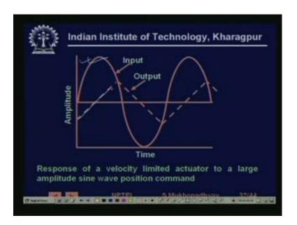
So, for example, if you give a large and then high frequency sinusoid, then the stem position will not be able to follow it, but rather it will, go up like this, so there will be a distortion you know. So, these things are to be kept in mind, when one is designing, a process control loop with a valve, that they have, this rate limits any actuator, most of the electromechanical actuators, actually have a rate limit.
