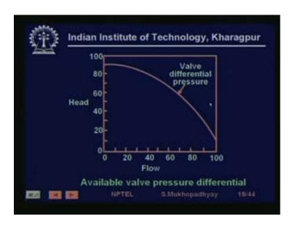
So, the operating point that are established, will always have delta P falling, so the valve differential pressure available, actually falls quite sharply with the flow, so it is not constant.
