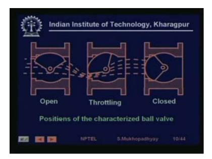
This is another, kinds of ball valve, where the ball is of a certain shape, so it is called a characterized ball valve. So, here you can see that, as again as it rotates this surface, slowly comes and closes the flow, and therefore the flow the flow can be throttled or it
