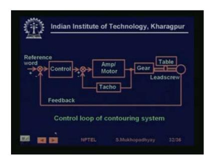
So, similarly you can have a reference word system, where which is a very conventional control system, where you simply use a, you give a simply give a position commands, it is a very conventional position feedback, using a, using this typical cascade control architecture. That is there is an, there is a loop inside a loop, so there is a tacho feedback for speed control and that is an actual feedback.
