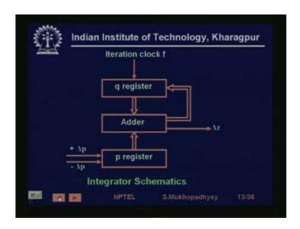
Let us, I think we should see the picture first and, the so you see this is the picture, so you see, this there is this q resistor which is finite this is a fix length resistor, pretty small length. So, what we do is, with and this is my p resistor, which gets added every time and by using these two plus and minus inputs, I can increment the value of p or decrement the value of p, in the case of linear interpolation, it need not be exercised p is constant.
