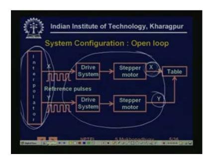
There are typically, there are two kinds of configurations which are used, for smaller systems, when with less critical requirements we use, open loop systems. So, you again you have a drive, you have motors, this is the table, that you can see, so this is the table in which, these are the two axis of motion, two axis X and Y, which create independent motions along the two axis of the table.
