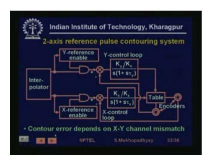
So, again with that was only one loop shown, and with respect to that, so now, you have two loops shown. So, this is the table, this is your Y axis control loop, and this is your X axis control loop, so you see the interpolator is giving reference words here, and the encoder is giving feedback, and rest of the control loop is just, shown by the transfer function. And there is an enable, so whenever the interpolator can enable these pulses, when it actually disables it, then these inputs go to 0.
