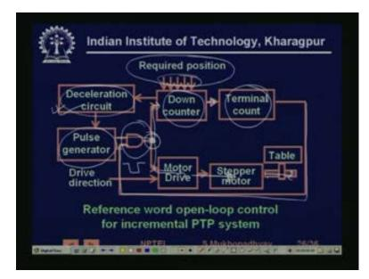
So, this is the typical circuit for a point to, so you see that, this is the reference word system, so we have the required position is actually, given by the interpolator, in terms of a digital word, that gets stored in a down counter. Now, this, from this down counter, it
