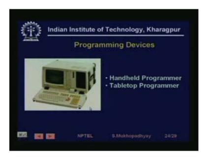
Then, you have programming devices and this is the typical programmer, programmers are of two types, either they could be handheld which you can take to the shop floor and directly program the PLC or they could be table top, where you have and which are of a higher capabilities. And where you actually develop programs offline and may be go on just load it there, because these have very good program development environments also. (Refer Slide Time: 53:08)
