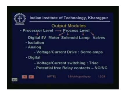
Then, we have output modules, they do the reverse, they translate processor level signals to process level signals, they are output devices and these process level signals, then go to things like motors, solenoid lamps, valves we have to actually do work. So, they have to be converted in form generally they have to made sometimes mostly they have to make be made analog or sometimes even on off kind of signals, but they have to be increase in power because, their suppose to do work.
