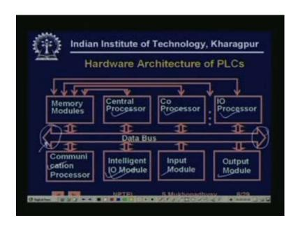
So, having looked at that let us see the how these various things are schematically connected, we just saw a diagram. So, you see that this is the scheme in which these various processors and the modules are connected, they are all connected by a bus, this is... And obviously, as we have seen that various I/O modules are mounted in rack. So, there will be a ribbon cable like thing, there will be a flat cable which will act as a this bus, you know it will connect the various modules.
