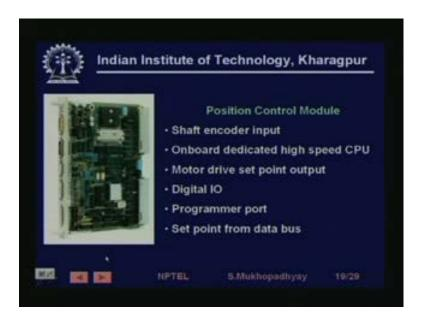
So, again position control module onboard dedicated high speed CPU, position control is generally requires very fast computation. So, you have dedicated high speed CPU by high speed CPU means, you have CPU with you know higher capabilities you used higher order processors, when you have low speed controllers, you use you know generally you use things like micro controllers to realize them, while here you could use higher end processor like may be 68,000 and motor drive.
