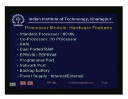
So, let us look at these modules at some level of depth now, so you have a typical processor would be I mean this is just an example, it could be 80186, it could also be from the 68,000 line various choices are available, sometimes these processors are you know proprietary not standard processors. Along with the standard processor as I said you could have co-processors, for specific purposes like I/O, like handling the
