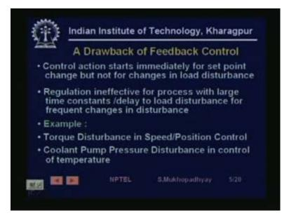
So, the main drawback of feedback control is that the control action starts immediately for set point change, but not for a change in the load disturbance. So, it immediately response to any change in set point, but not, so for a change in the disturbance, will see how. Therefore, why is it so? Because of the fact that the, if you see the feedback loop let us see the feedback loop, back again to appreciate this. I am sorry we are going back, you are not going back you should have gone back.
