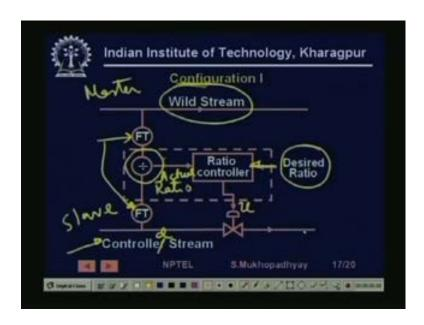
So, the first one is configuration 1, let us see that. So, you see in ratio control we have two streams the first one we call the wild stream. So, we do not directly control that stream, that stream is controlled by other considerations may be from production volumes, but, so it is like it is like a master stream which changes independently because of some operator change etcetera.
