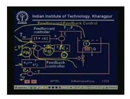
So, what is happening here, first let us, it is the same process. So, we have the feed forward controller. So, we have a T set point which is coming through a command pre filter command pre filter and T i they are going through this F i this should be this should be rho C p and then we are getting u right?
