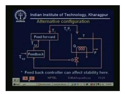
On the other hand, we could also connect these in a slightly different way for example, here what are we doing, here we have the usual feed forward. Again we are again we are measuring the disturbance this is the feed forward controller and we are giving u here standard again the same situation.
