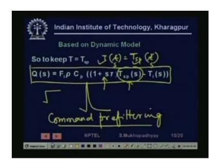
So, if we have, if we want to keep T is equal to T sp, T is equal to T sp means we want to now make T t is equal to Tsp t, that is every time instant not the final values every time instant we want to keep T t equal to T sp t. Then, obviously, if we consider them in the Laplace transform domain then t s will be equal to Tsps.
