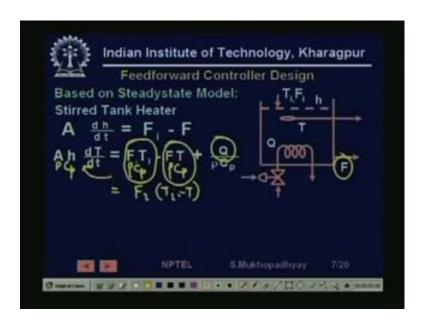
So, now having recognized this let us understand, let us see how we can design feed forward controller. Now, as we said that design of the feed forward controller would require a model now, models are difficult to obtain, but even with those difficulties steady state models are actually easier to obtain. So, therefore, let us first see that how based on a steady state model we can design a feed forward controller.
