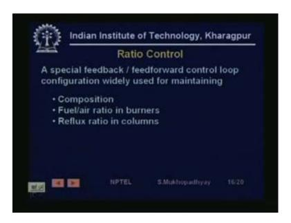
So, it is a special feedback feed forward control loop configuration which is widely used for maintaining composition control, fuel air ratio in burners, for example let us say if you have a if you have a any kind of burner let us say a boiler. So, boiler has a furnace see you have to produce flame, for producing flame you need two things, you need the fuel and you need the air, but they must be provided in such a ratio such that complete combustion takes place.
