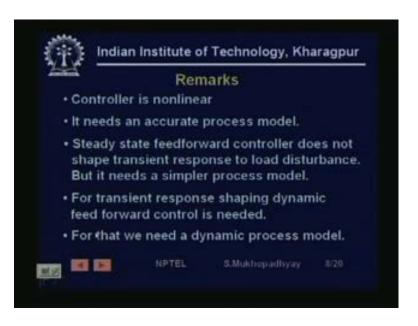
So, let us have see some remarks about the controller first that the controller is non-linear because, you have you have F T all these things can get multiplied together. So, there is no guarantee that is going to be linear. But that does not make in a difference to us we can always make non-linear calculations in a process. It needs an accurate process model as I have said, if you make errors in any of the coefficients you are going to get an error in control.
