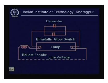
This diagram shows the complete functioning. We have the all the accessories shown. There is a glass envelope, it's a long tube where the lamp at either end there are two electrodes which are basically similar to your, what we found in the sodium vapour lamp or mercury vapour lamp. It shows the complete circuit diagram. This is the total line voltage applied across that ballast or choke which is known as which is predominantly electromagnetic off late we have been using
