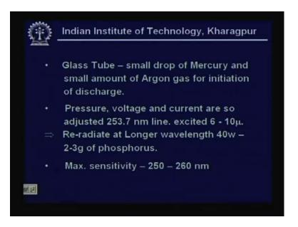
You have a glass tube with a some small drop of mercury and small amount of argon. Again why argon? Argon is necessary to vaporize your mercury to initiate the arc because it's still is an arc lamp or a discharge lamp. There the whole process is such that we control the pressure, voltage and current so that we have in the 253.7 nanometer line and then radiate at longer wavelength. A typical 40 watt fluorescent lamp will use about 2 to 3 grams of phosphors. We will see these what phosphors are.
