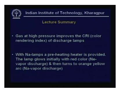
Gas at high pressure does improve the colour rendering because mercury vapour lamp radiation shifts to the mid spectrum, with sodium lamps a preheating heater is provided and as the initiating vapour is neon we get a red colour which turns to characteristic orange yellow colour.
