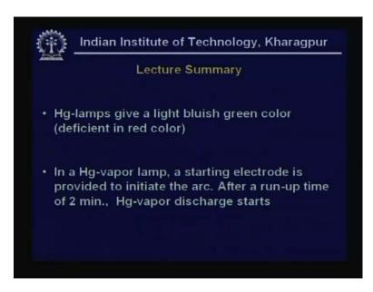
Now mercury vapour lamps as already said characteristic bluish green colour is what they give. As we have known that the gas vapour decides the type of colour. In a mercury vapour lamp a starting electrode is provided and typical run up time could be anywhere from 30 minutes 2 minutes I said here we are waiting 2 minutes because these day technology is available to start quickly.
