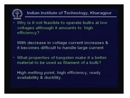
Why is it not feasible to operate bulbs at low voltages although it amounts to high efficiency? With decrease in voltage current increases and it becomes difficult to handle large currents. What properties of tungsten make it a better material to be used as a filament of a bulb? High melting point, high efficiency that is luminous efficacy, ready availability and ductility. Thank you.
