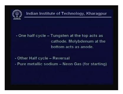
So the tungsten acts as the cathode and the molybdenum acts as anode. If the tungsten at the top acts as cathode in one half cycle, molybdenum at the bottom acts as anode and in the other half cycle the whole process reverses. The metallic sodium is placed and there is a starting gas in fact in the mercury vapour lamp, we had argon as the starting gas. Here we often have neon gas,
