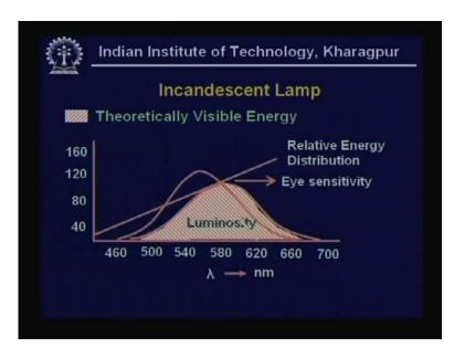
This is for the incandescent; we have seen the relative energy distribution. As can be seen higher the wavelength higher is the energy available eye sensitivity, so you find which is more or less visible energy is somewhat similar to what we obtain in the case of sunlight whereas the low pressure mercury vapour lamp has two bands, one in the uv zone.
