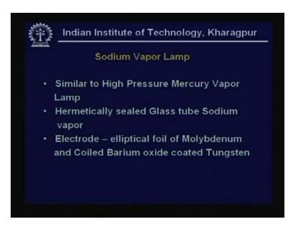
This is the electrode and so if you have recall the picture we saw of the discharge tube, one half cycle tungsten at the top acts as cathode, molybdenum at the bottom acts as anode that means each of the electrodes, each of the electrodes recall that they had a foil of molybdenum and barium oxide coated tungsten.
