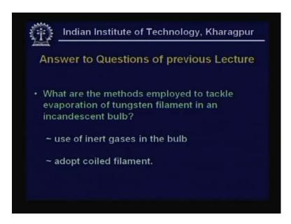
Some of the questions which were asked in the last lecture like what are the methods employed to tackle evaporation of tungsten filament in an incandescent lamp? Use of inert gases in the bulb, adopt coiled filament.
