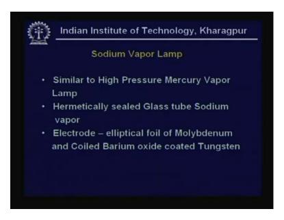
Mercury was in the liquid state, on the other hand sodium in a solid state which can get vaporized pretty easily. This is sealed, hermetically sealed in a glass tube just as it. Now here again we have two electrodes, one which can act as cathode and anode depending on the half cycle to which it is applied. These are made of elliptical foils of molybdenum and you have barium oxide coated tungsten on top of this on the base.
