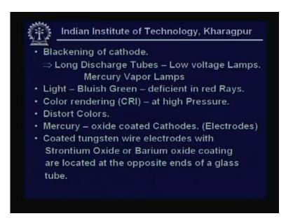
This blackening of cathode and therefore calls for long discharge tubes and so keeping this in mind we look at the mercury vapour lamps which are extensively, there are two categories of a discharge lamps which are of importance, one is mercury the other is sodium. Mercury in fact because it's got the radiation located around blue region. In fact light due to mercury vapour is bluish green and its deficient in red rays because of which the colour rendering is very poor.
