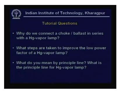
Continuing with the questions, why do we connect a choke or a ballast in series with a mercury vapour lamp, what steps are taken to improve the low power factor of a mercury vapour lamp, what do you mean the principle line, what is the principle line for mercury vapour lamp. The principle line...
